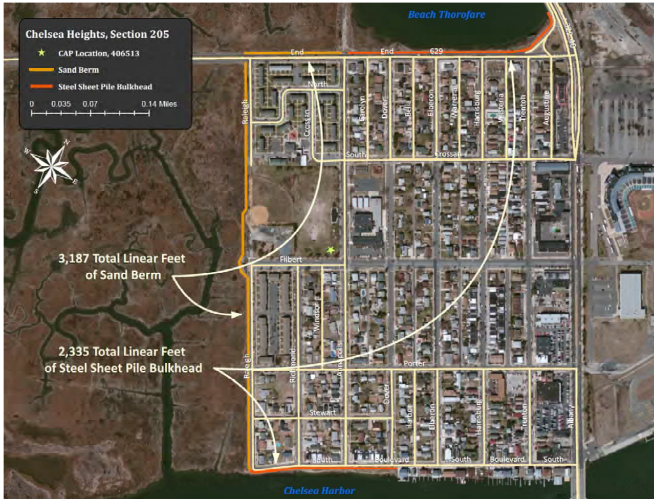
Figure 3: Location of proposed steel sheet pile bulkhead and sand berms.
