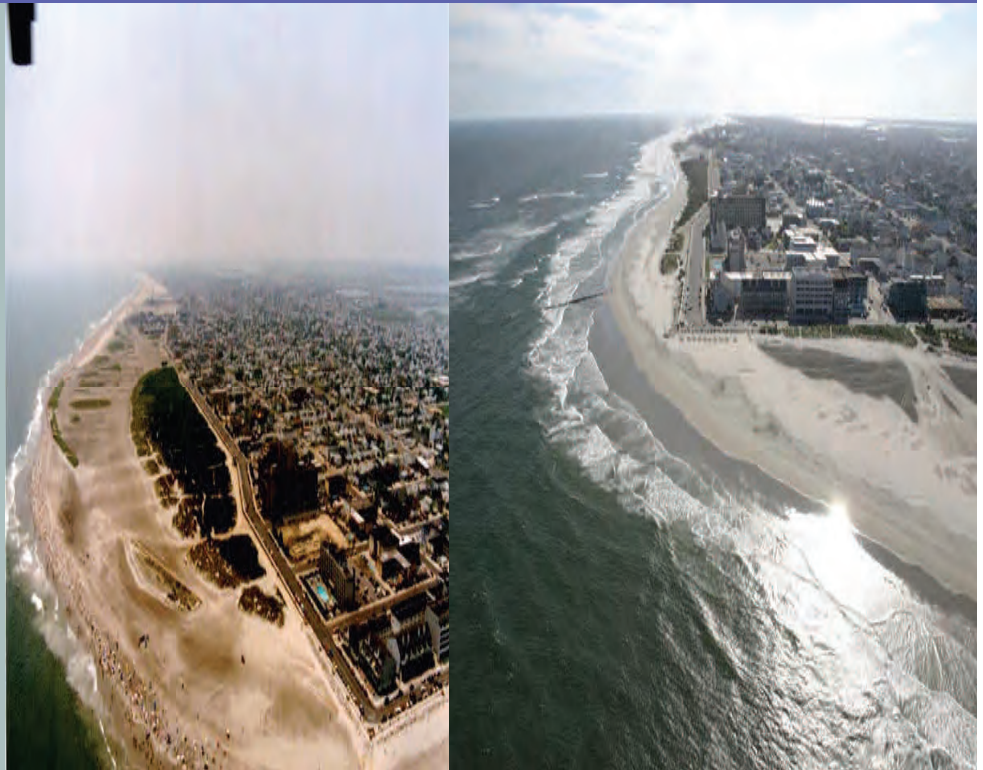
The photo to the left shows the extend of the North Wildwood Beach from July 1989. The photo to the right from 2004 of the same area demonstrates the extent of the erosion that has taken place since 1989.
