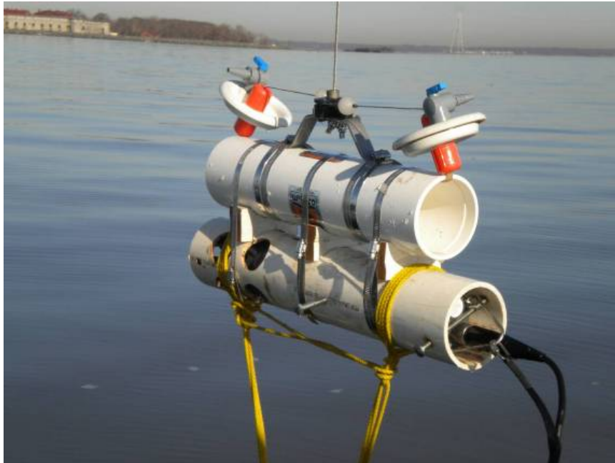
Figure 2-2. YSI water quality meter attached to open sample bottle for the Point of Dredge TSS and turbidity testing for the Delaware River Deepening project
