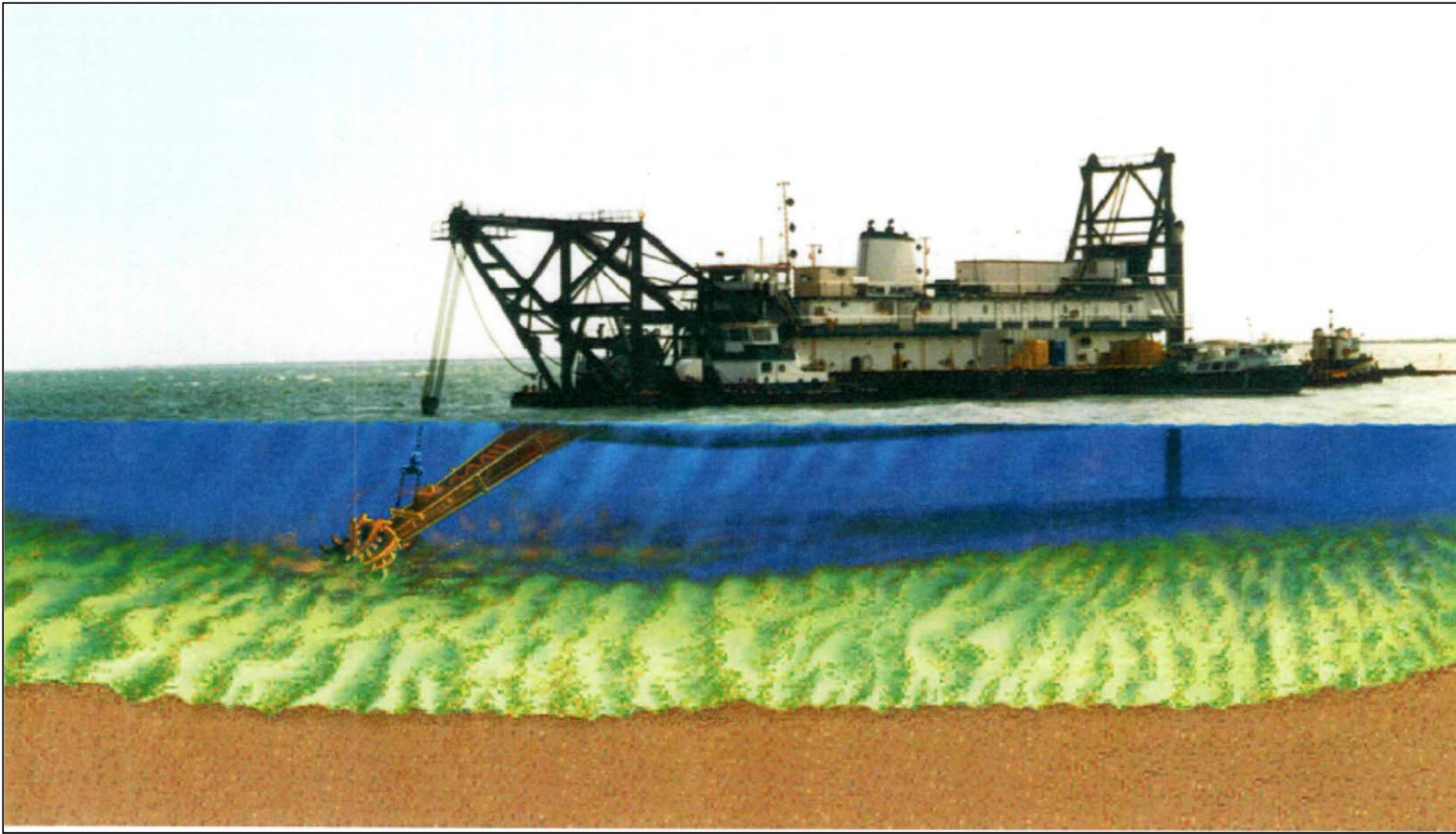
Figure 1-2. Configuration of a typical cutterhead dredge
