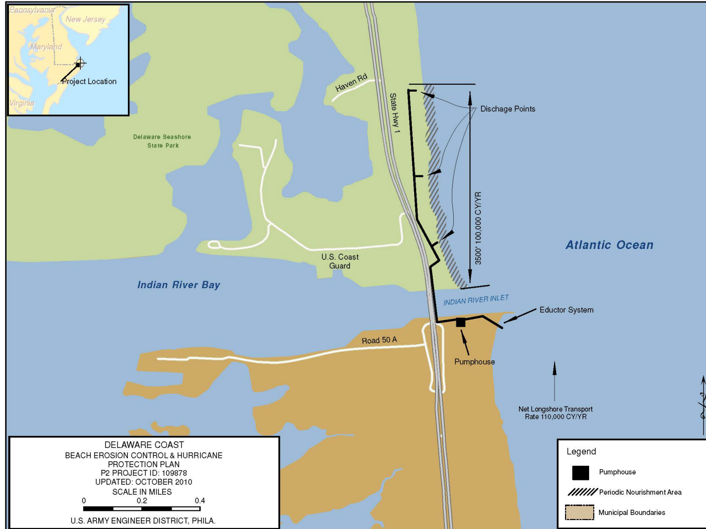
Figure 1. Delaware Coast Protection - Indian River Inlet Sand Bypass Plant and North Beach Beachfill Placement Area
