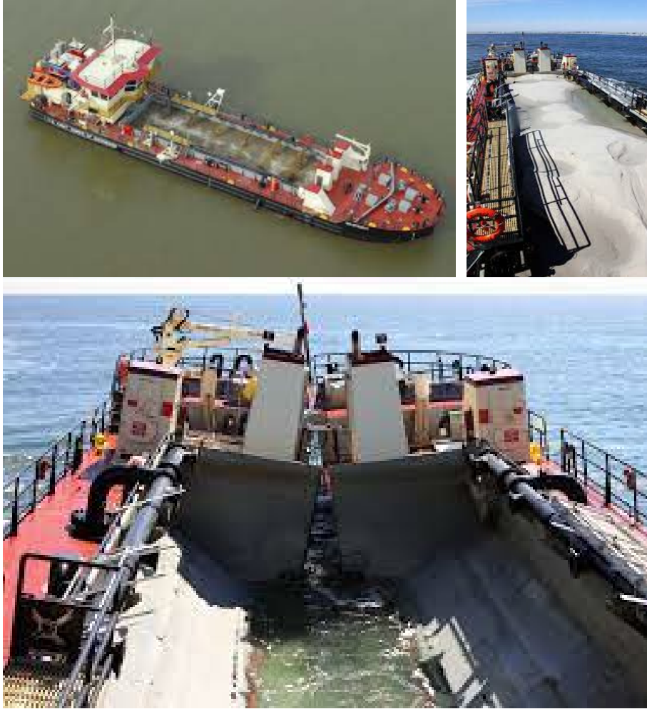
Figure 15. The Dredge Murden with a Capacity of 518 Cubic Yards is In-Filling (left), Laden with Sand in Transport (right), and Split-Hull Bottom Dumping (bottom). Photos are from Wilmington District USACE (upper left) and Philadelphia District USACE (right and bottom).
