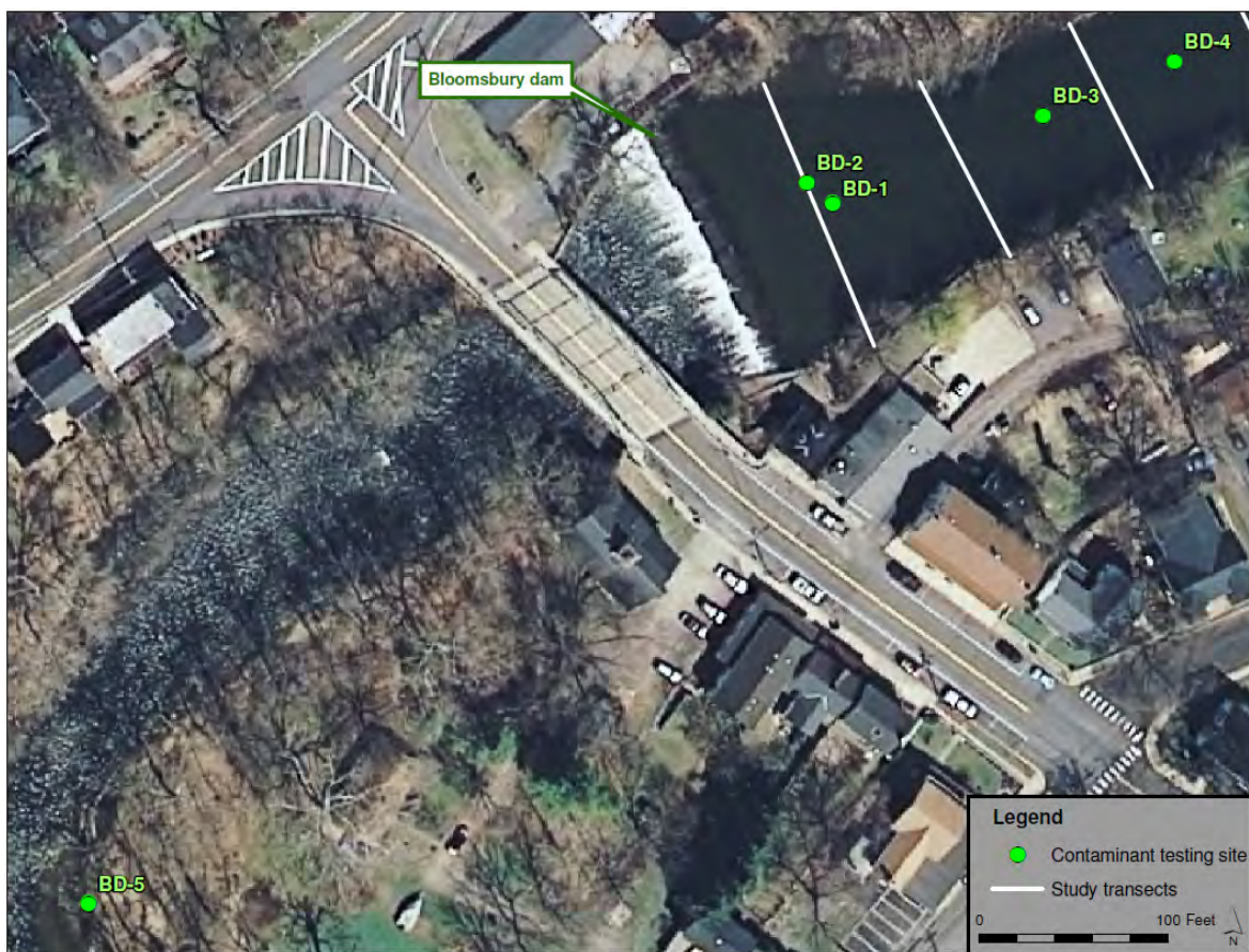
Figure 2-1. Sediment sampling locations for contaminant analysis at Bloomsbury Dam. Transect lines indicate the locations of the sediment depth measurements.
