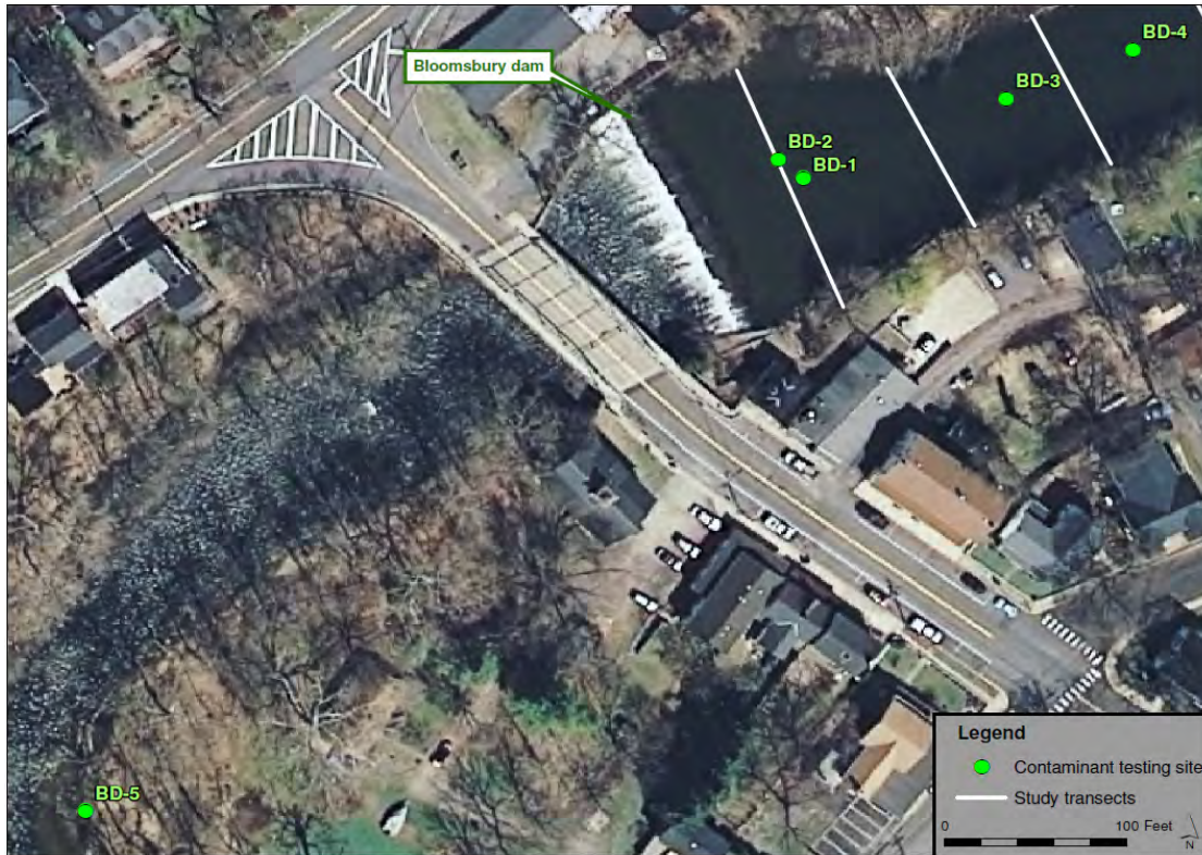
Figure 9. Sediment sampling locations for contaminant analysis at Bloomsbury Dam. Transect lines indicate the locations of the sediment depth measurements.
