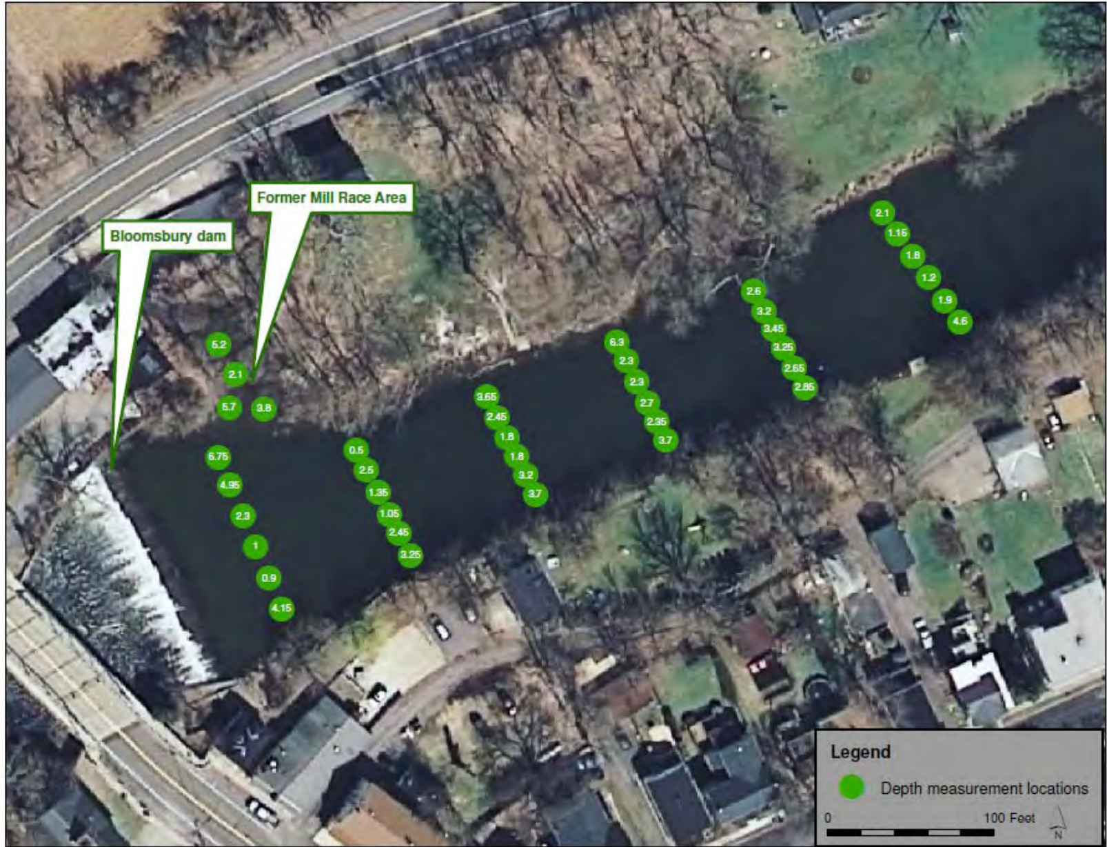
Figure 3-3. Measured sediment depth at each sampling point behind Bloomsbury Dam and at the Former Mill Race Area.
