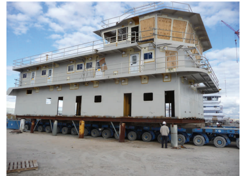
Rolling Prefabricated Deckhouse
