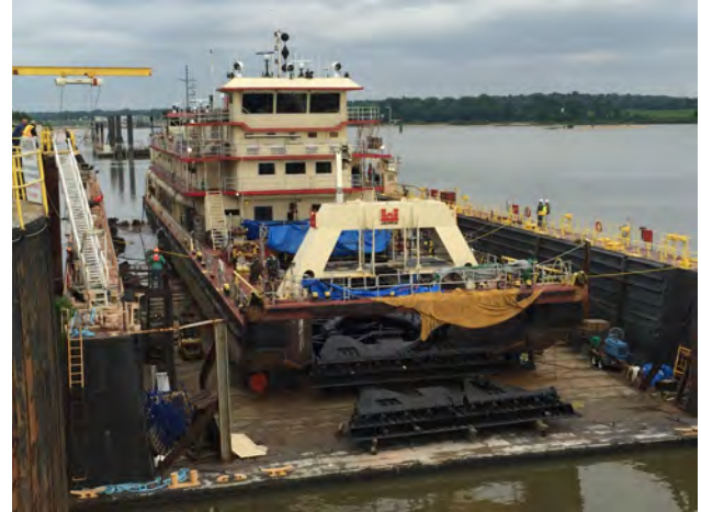
JADWIN in EEY Drydock with new ladder and gantry
