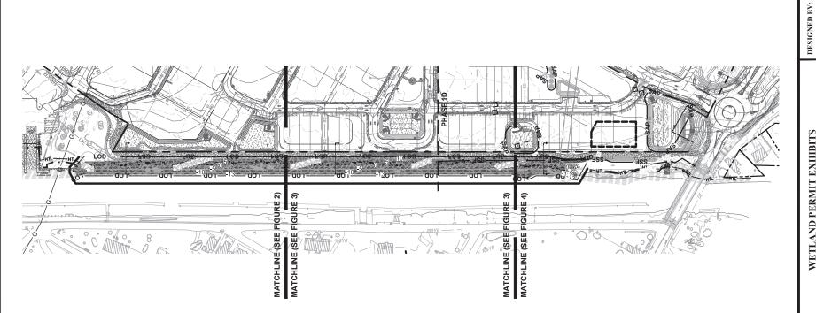
TOTAL LIMIT OF DISTURBANCE: 1.96± AC WETLAND LIMIT OF DISTURBANCE: 0.82± AC RIPRAP FILL VOLUME: 5267± cu. yd.
