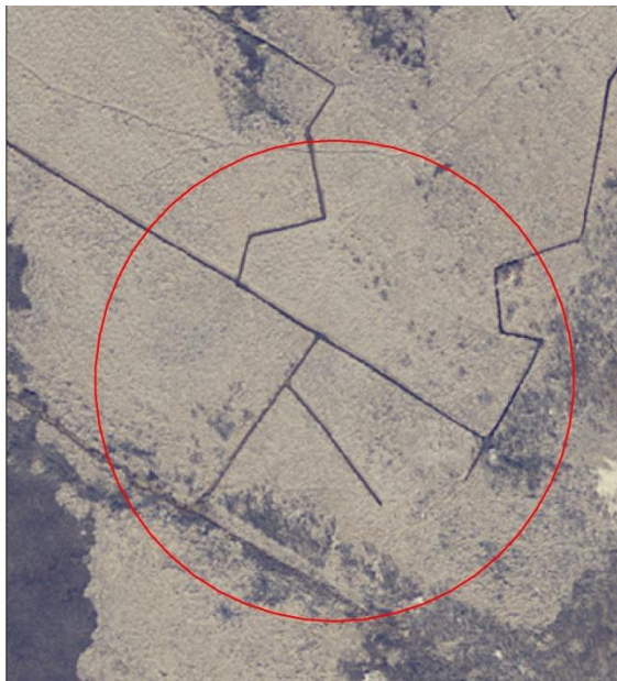
Example 3: Multiple narrow ditches throughout AA. 312.9 m 2 : 3.9% of AA is ditched: Score: 6
