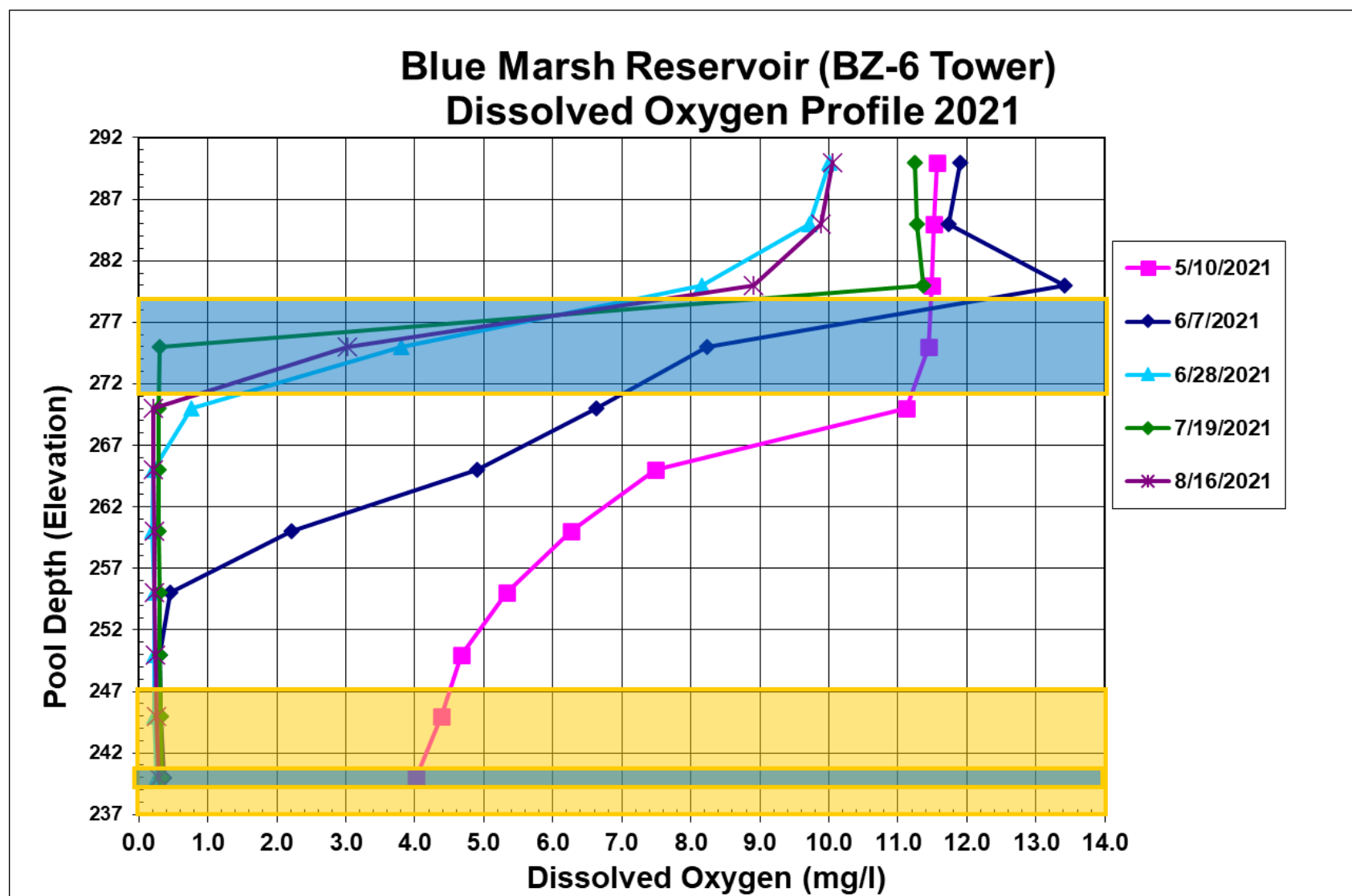
Figure 3-4. Release portal elevations and dissolved oxygen stratification at station BM-6 of Blue Marsh Reservoir in 2021. (PADEP water quality standard for DO is a minimum concentration of 5 mg/L.) See Appendix A for summary of plotted values.
