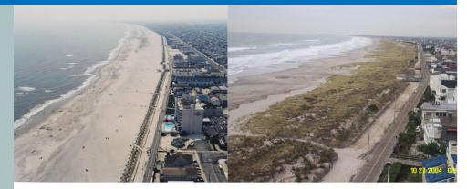
Shortly after the completion of initial construction, the City of Ocean City planted beach grass and installed sand fence to encourage dune growth. Years later, as shown above, continued periodic nourishment by the Corps has allowed the same area to expand into a substantial dune field.
