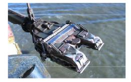
Dredging is accomplished by a drag arm on each side of the ship with a drag head a each end. As the ship navigates the channel with its dredging pumps engaged, the drag heads are lowered to the channel bottom. Like vacuum cleaners, they pull the dredged material into the ship's hoppers.
