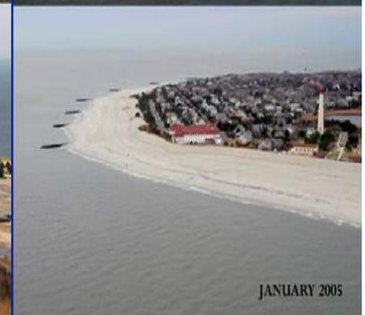
**Left:** Beach and wetlands that were lost to long-term erosion have been restored, and the dune line has been reconstructed seaward.
