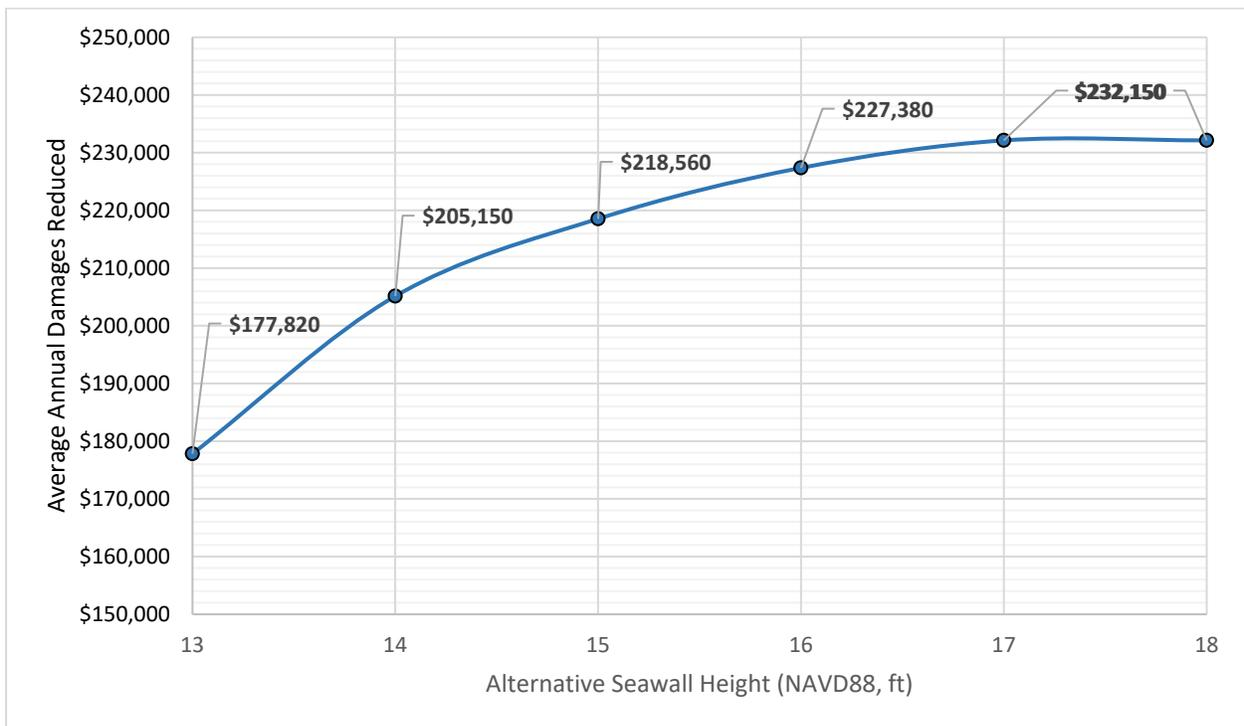
As the alternatives increase in height, the rate at which each successive foot added to the seawall improves Average Annual Benefits diminishes until the seawall at 17ft NAVD88 maximizes damages reduced. To optimize the seawall height, the percentage increase in benefits from each successive foot will need to outpace the percentage increase in cost from each successive foot. Cost estimates are shown in the following section and Average Annual Net Benefits shown in Table 12.
