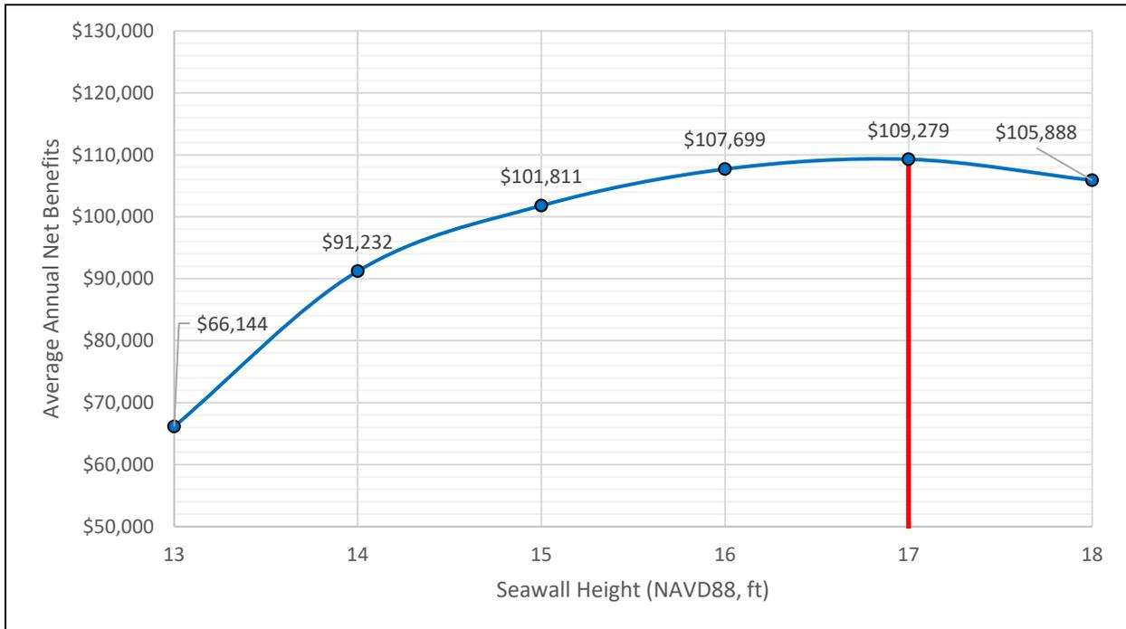
National Economic Development (NED) Benefits are maximized for this study area with the construction of a concrete cap atop the existing seawall to bring the final seawall elevation to 17ft NAVD88. Figure 12 shows the optimization at 17ft NAVD88 with \$109,000 in AANB.
