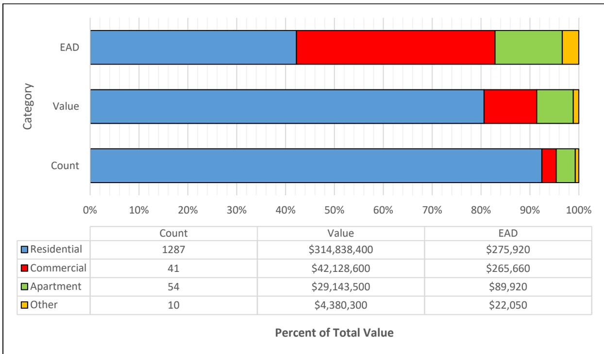
Residential structures constitute an overwhelming majority of total inventory count and value, but only a plurality of equivalent annual damages at 42.2%. Commercial structures have lower volume, but higher depreciated replacement values and risk levels, contributing a 40.6% share of without-project expected annual damages.
