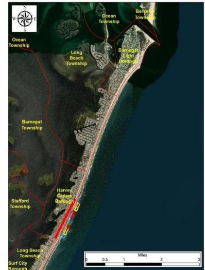
**Above:** The first component of the project involves dredging between the jetties and placing the sand in the nearshore of Harvey Cedars, NJ to support the federal beach project. **Below:** Looking east at Barnegat Inlet with previously created island in foreground.
