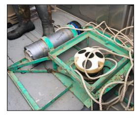
**Top Left:** ISCO water sampler platform sampling water flows in a tidal creek.
