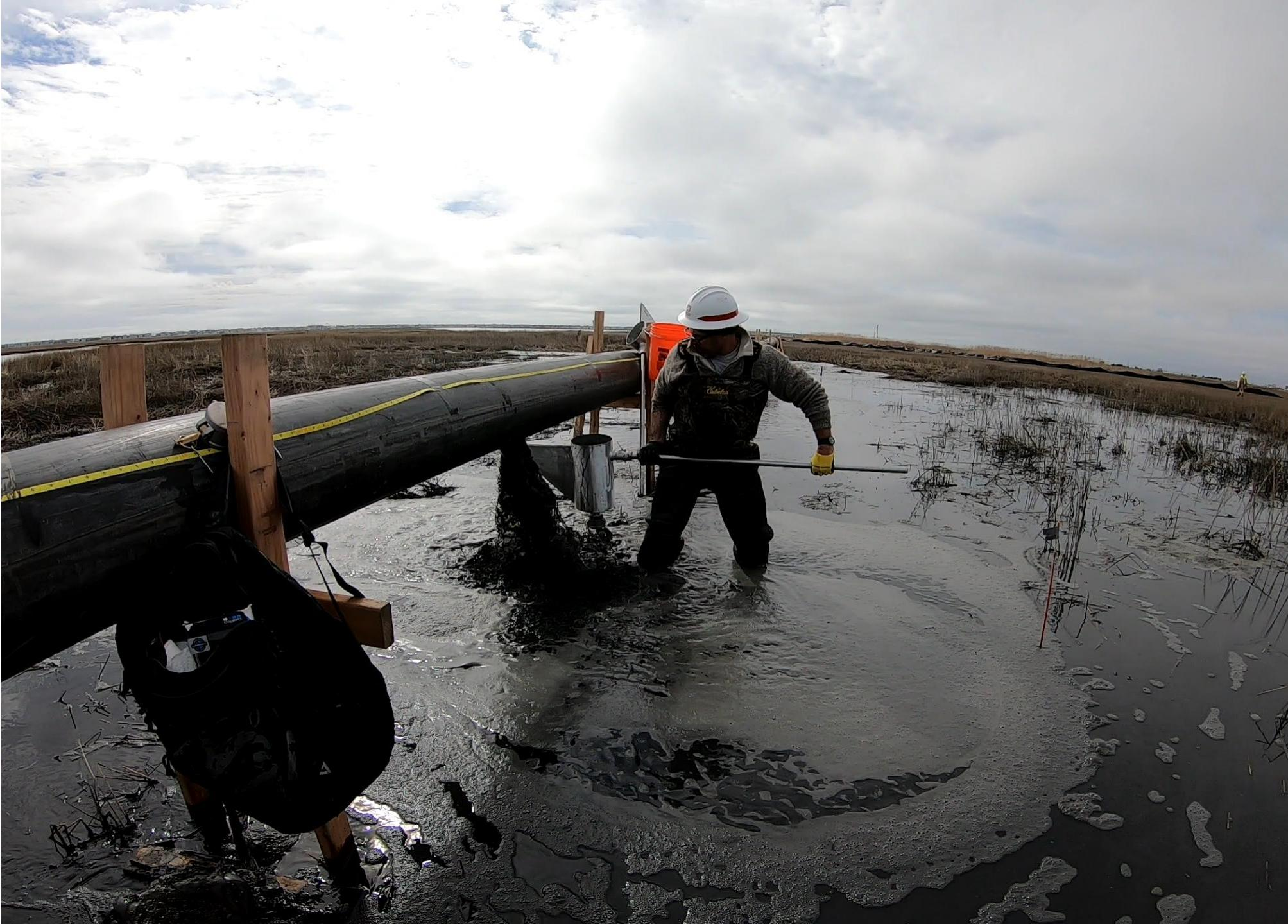
**Slurry sediment analysis from each distribution hole and the end of pipe discharge for two hole sizes and two flowrates.**
