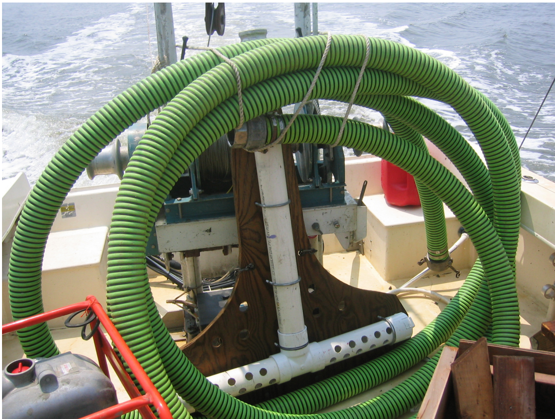
Figure 2-6. Suction-dredge and intake hose used in the juvenile horseshoe crab survey
