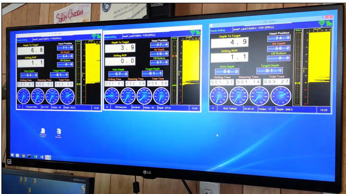
**Figure 3 – Monitoring of the Three Drill Frames in the Survey Office**
