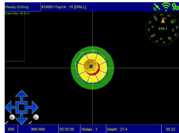
System in Drill Mode with Dashboard off. The benefit of this feature is the ability to view the current pattern while in drilling mode.
