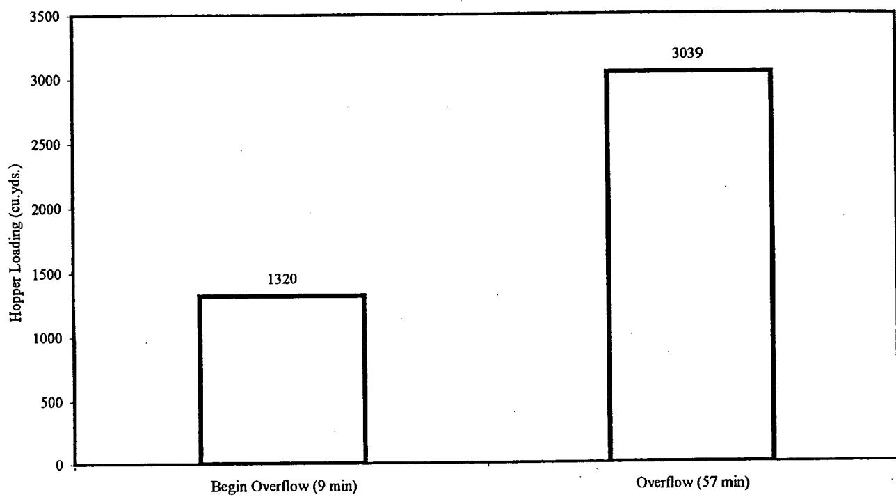
Figure 4: Hopper Loading at Fine-Grained Site
