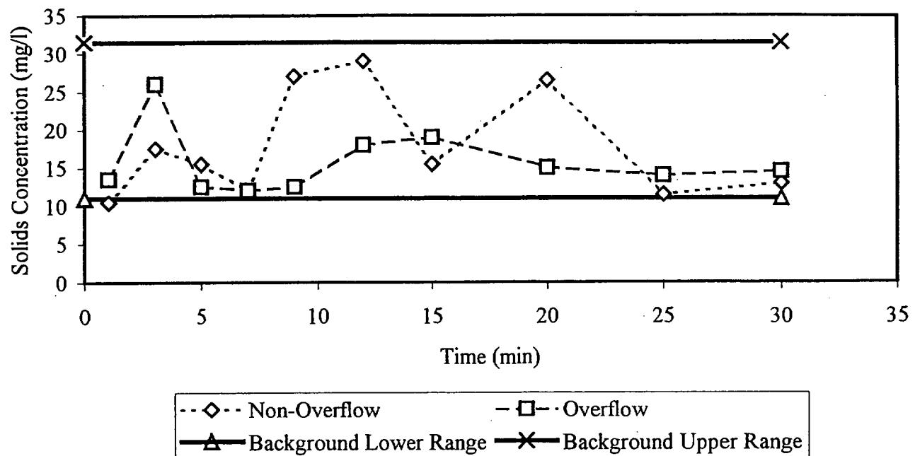
**Figure 18: Plume Solids Concentration Coarse Grained Site**
