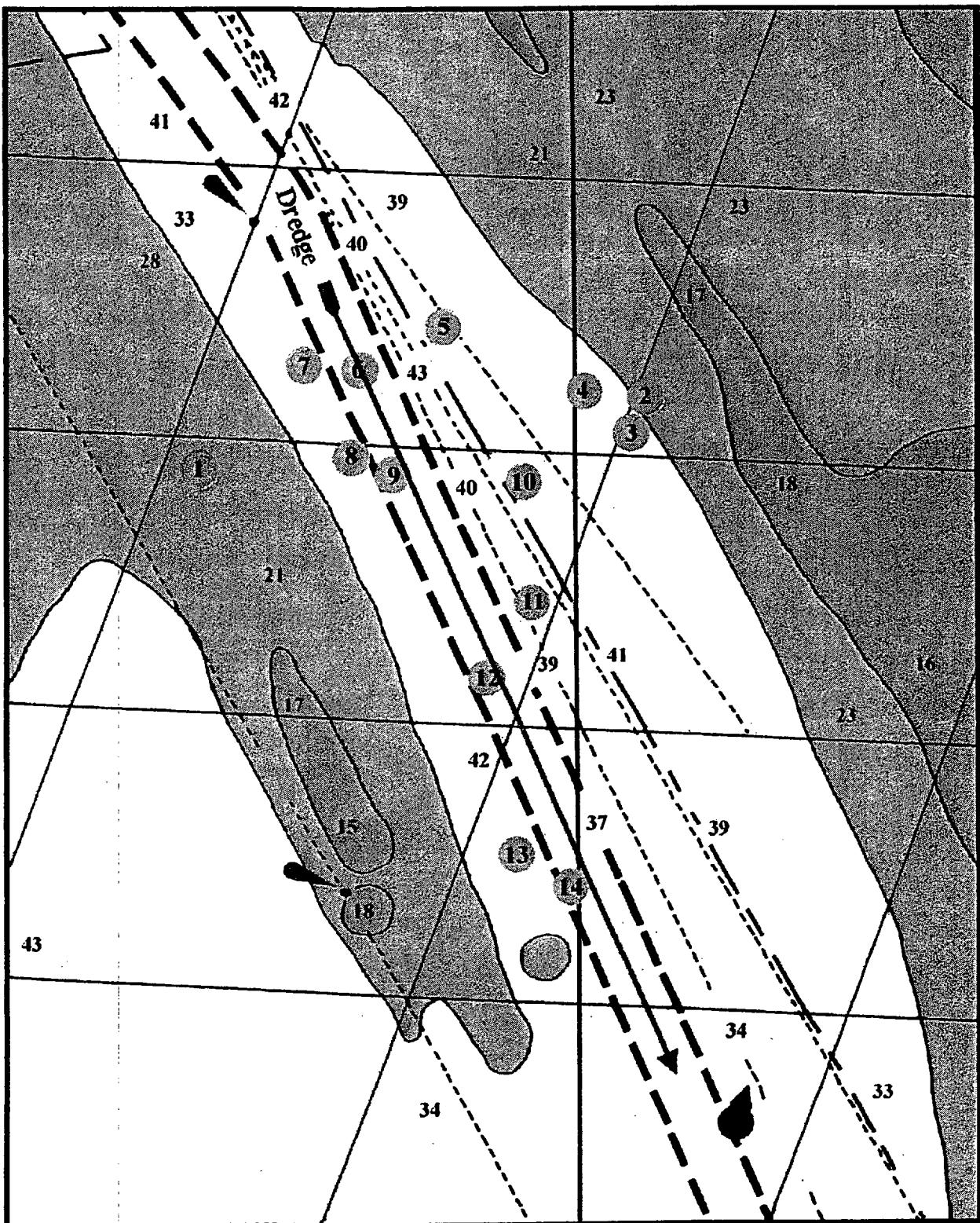
**Figure 2.** Sediment profiling imagery stations occupied during hopper dredge loading and overflow tests at the lower study site. The figure has been modified from a NOAA navigation chart with depths indicated in feet. Approximate start and end of test locations of the dredge are indicated by the red arrow.
