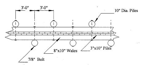
Terminal Groin Profile is the same as for groins but extends 450 ft offshore from the berm crest.
