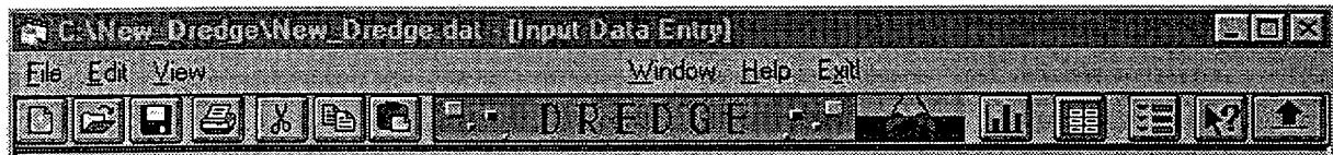
The button bar provides direct access to the most commonly used menu items. An icon on each button suggests the action that results from pressing the button; allowing the mouse pointer to hover over the button momentarily will display a tool-tip description. Pressing the left mouse button while the pointer is over the rectangular area of the button initiates the associated action. Table 2 describes the available buttons and the associated actions.
