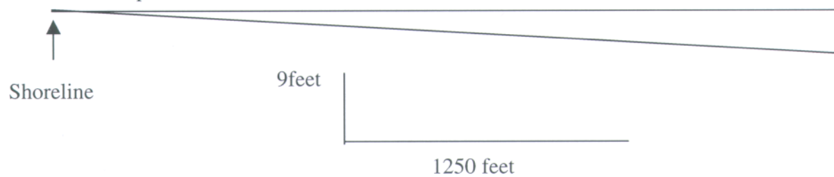
Figure 2-3. Reedy Point South CDF outfall configuration
