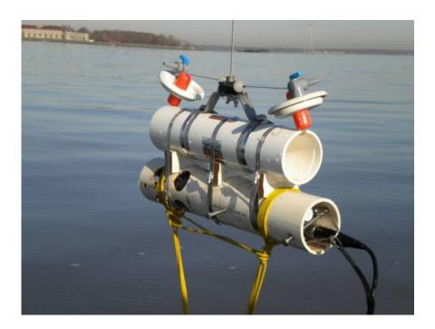
Figure 2-3. YSI water quality meter attached to open sample bottle for the Point of Dredge TSS and turbidity testing in Reach C of the Delaware River Deepening project
