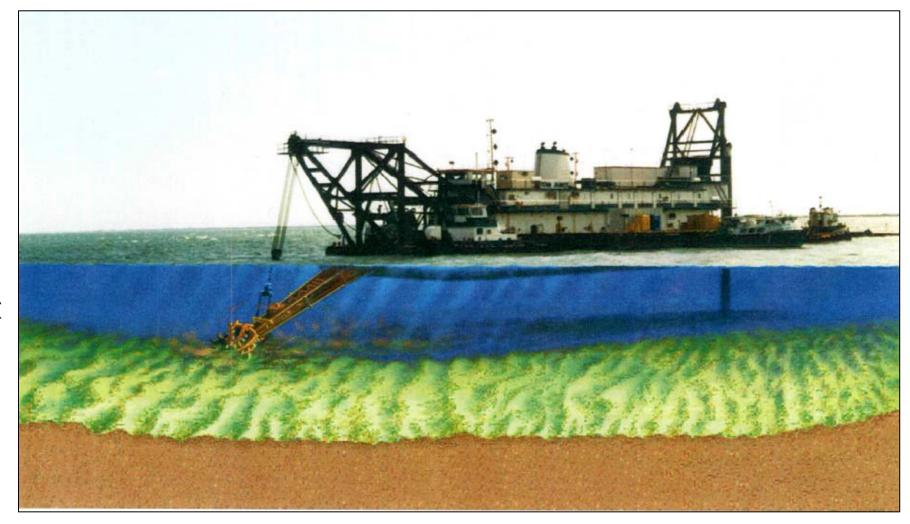
Figure 1-2. Configuration of a typical cutterhead dredge
