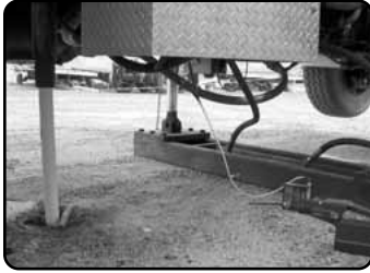
CPT sampling (view under truck)
