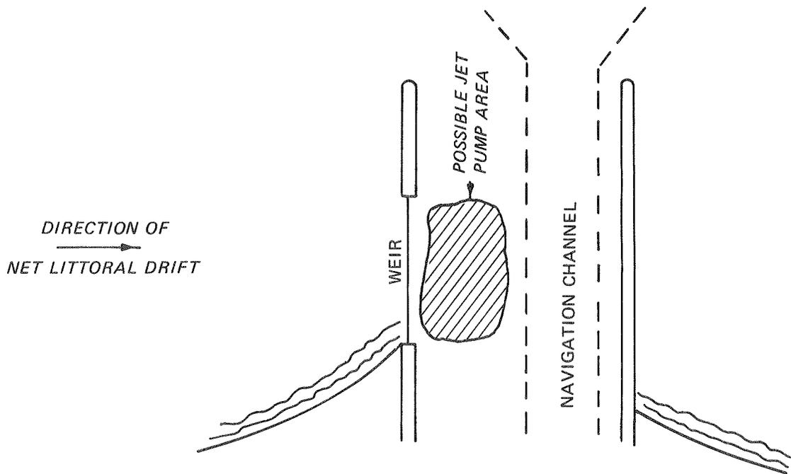
Figure 15. Jetties with weir section
