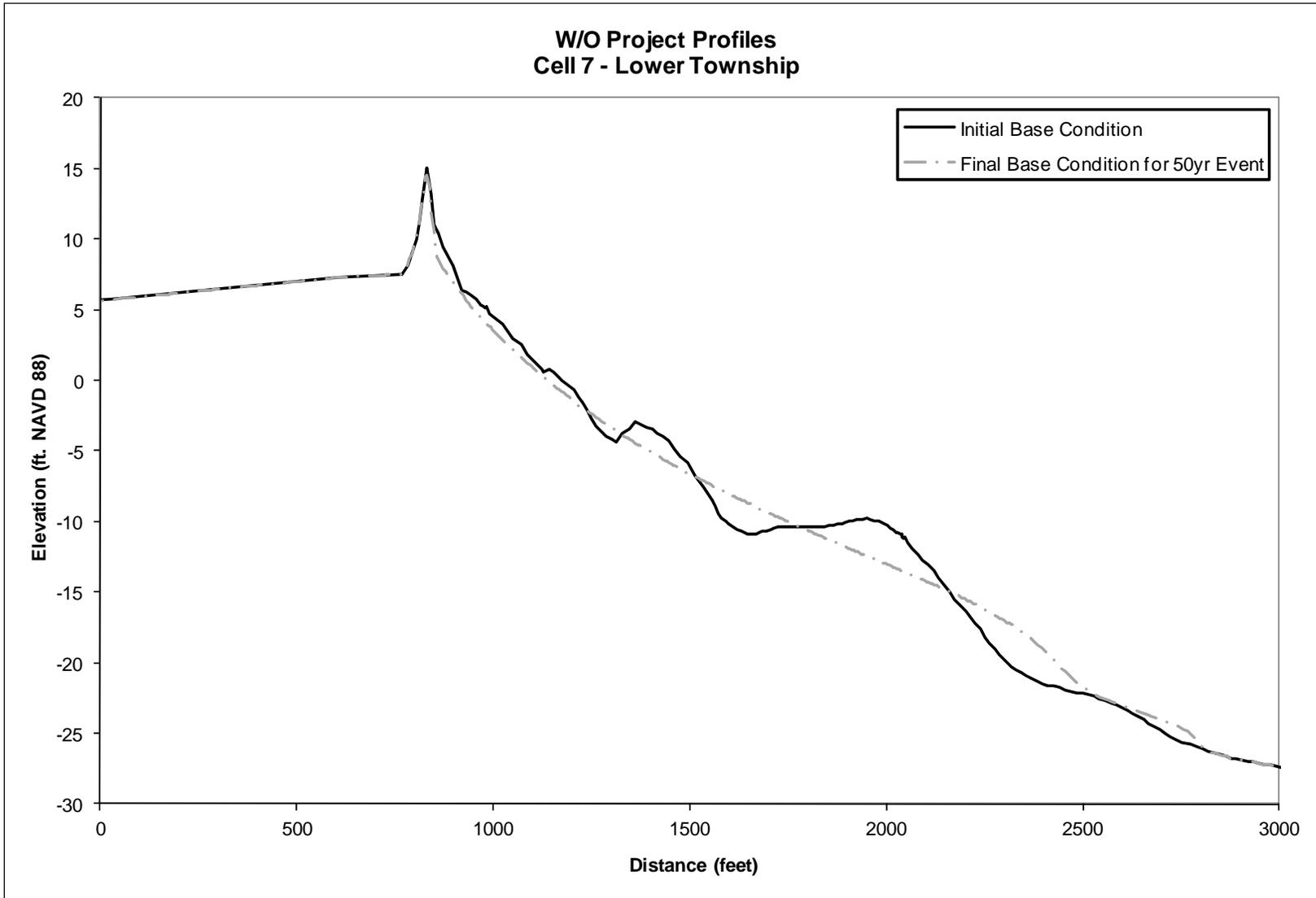
**Figure 42. Pre- and Post “50-yr” Storm Beach Profiles for Without Base Conditions in Cell 7**
