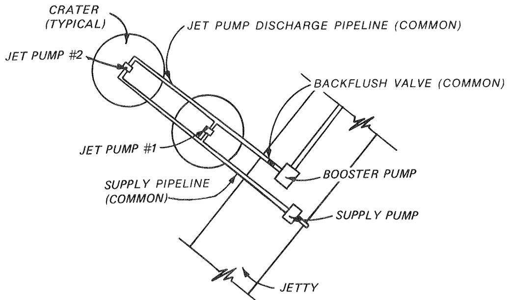
Figure 24. Two jet pumps with common discharge pipelines
