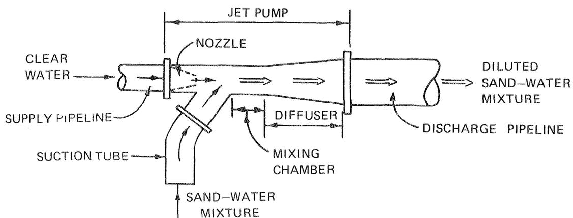
Figure 3. Jet pump principles of operation
