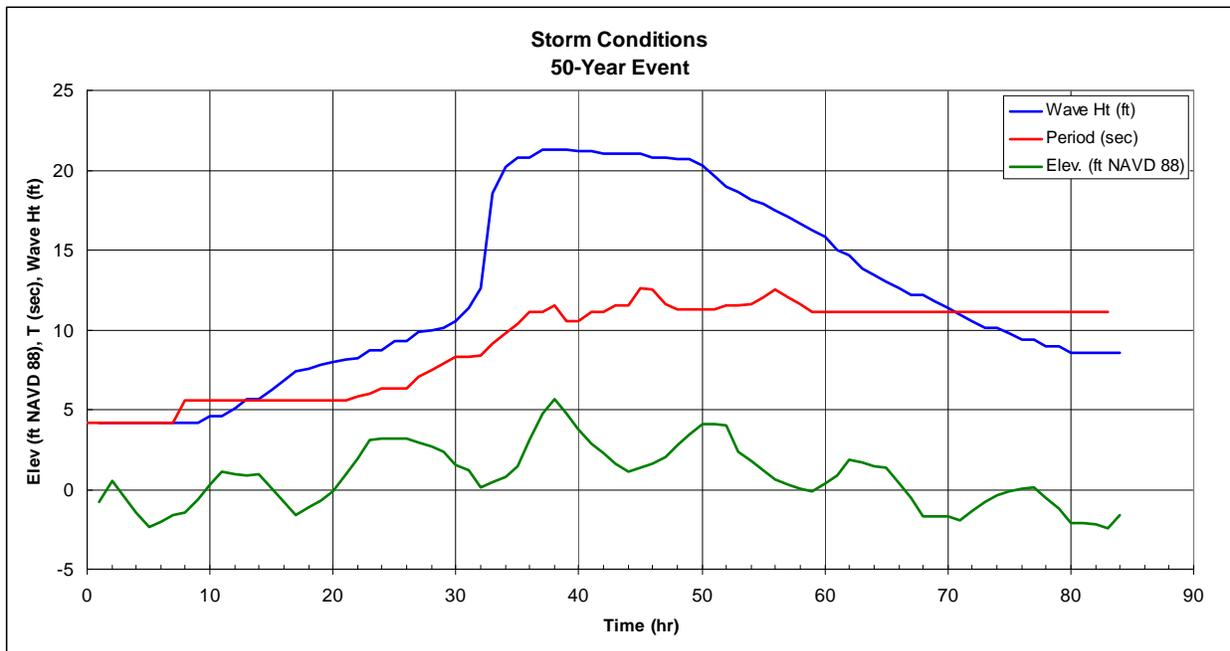
**Figure 32. “50-yr” Storm Conditions used in Storm Damage Analysis**
