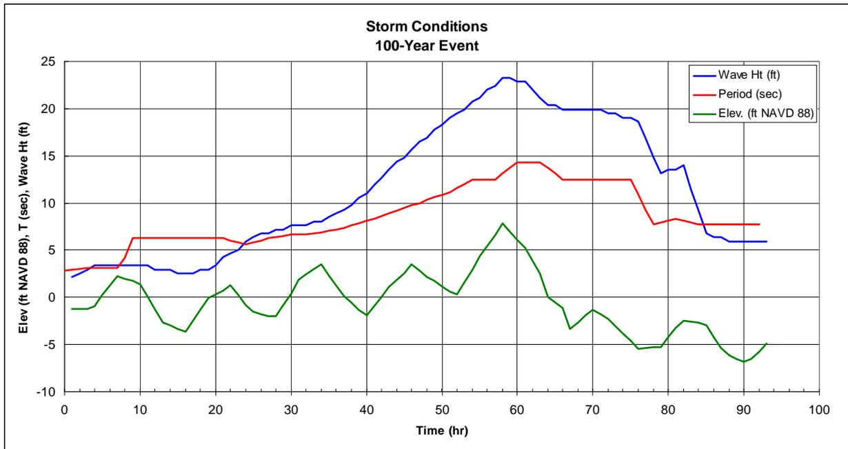
**Figure 33. “100-yr” Storm Conditions used in Storm Damage Analysis**
