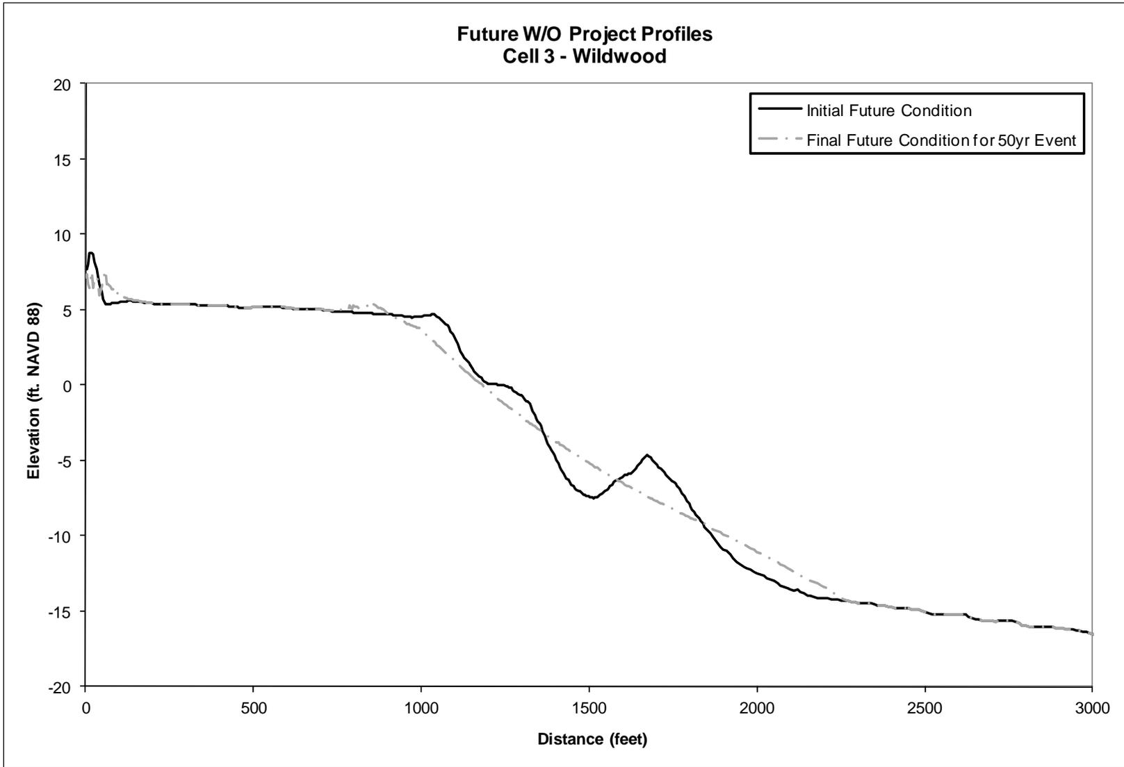
**Figure 45. Pre- and Post “50-yr” Storm Beach Profiles for Without Future Conditions in Cell 3**
