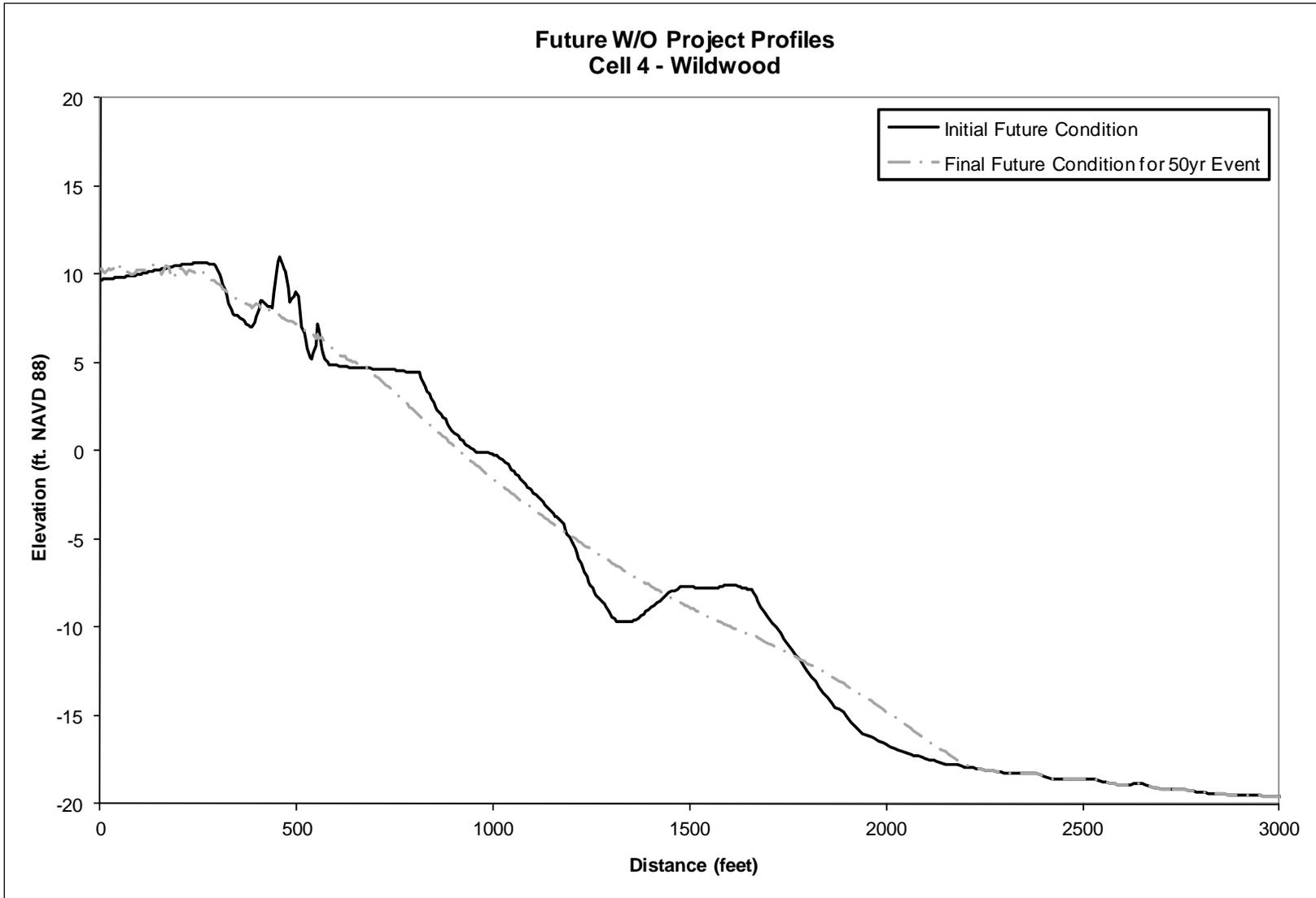
**Figure 46. Pre- and Post “50-yr” Storm Beach Profiles for Without Future Conditions in Cell 4**
