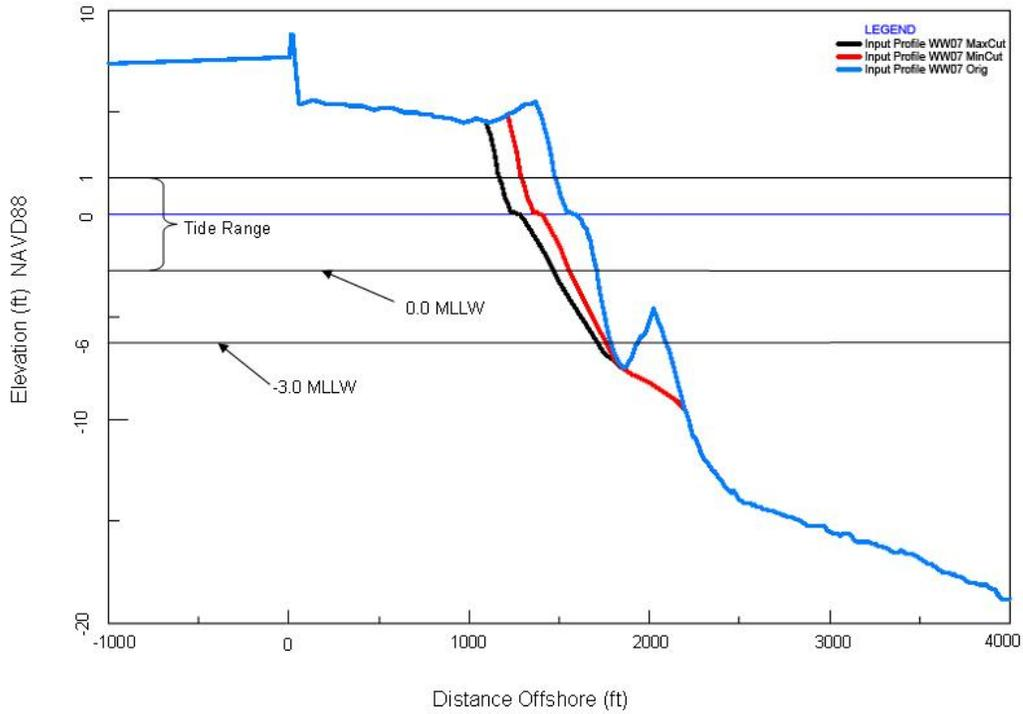
Figure 4. Beach profile at Wildwood showing proposed borrow location. Note this figure has an error, it shows the tide range as 6 ft. This will be corrected on Wednesday AM.
