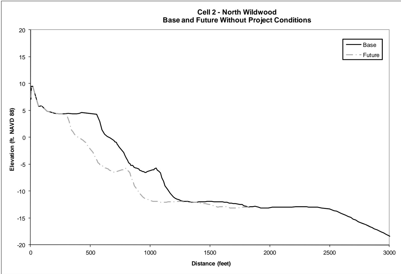
**Figure 23. Base and Future Without Project Conditions for Cell 2**
