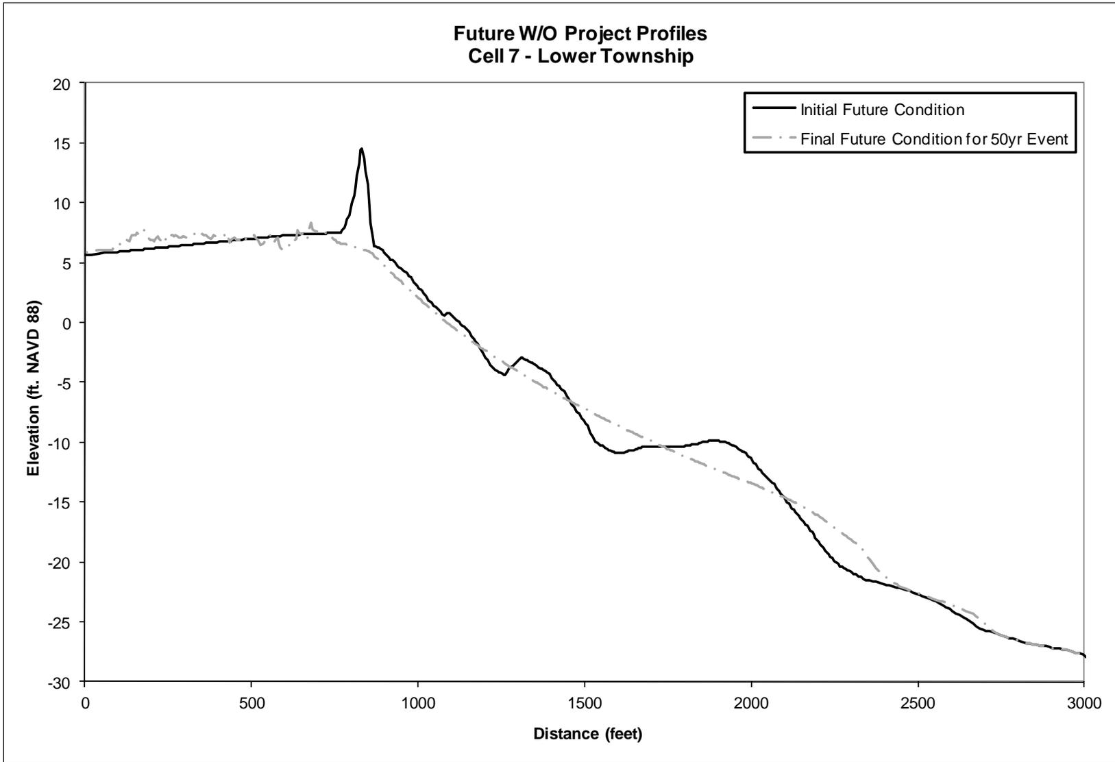
**Figure 49. Pre- and Post “50-yr” Storm Beach Profiles for Without Future Conditions in Cell 7**
