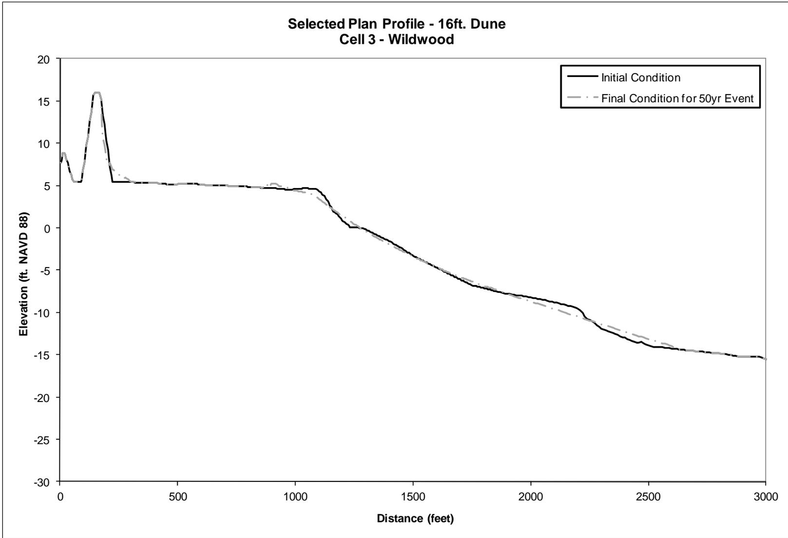
**Figure 54. Pre- and Post “50-yr” Storm Beach Profiles for Selected Plan in Cell 3**
