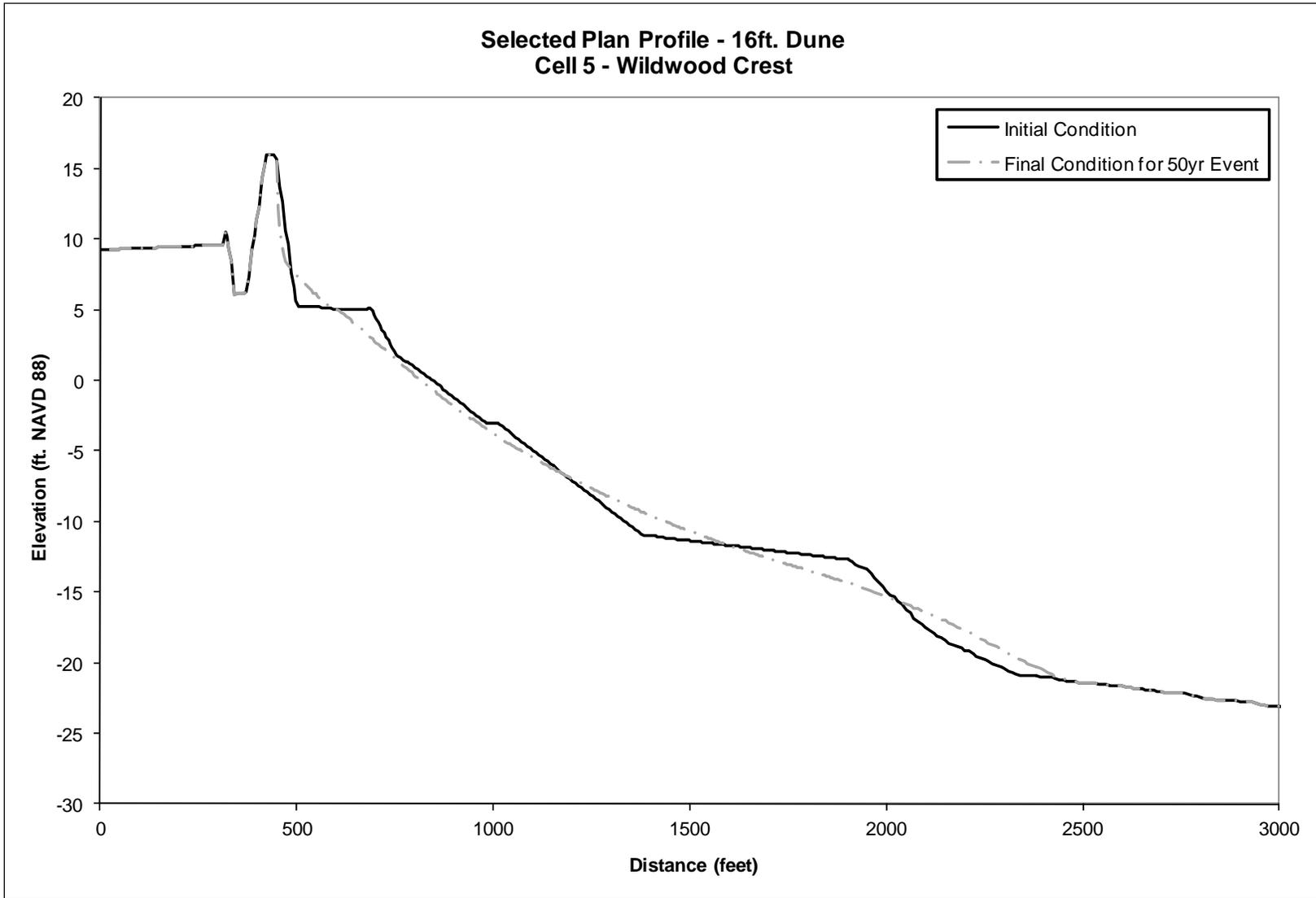
**Figure 56. Pre- and Post “50-yr” Storm Beach Profiles for Selected Plan in Cell 5**
