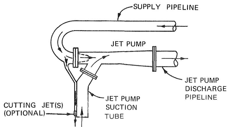
Figure 7. Elevation view of jet pump
