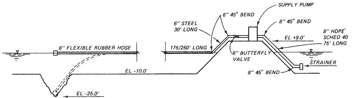
Figure 29. Jet pump supply system (elevation view)
