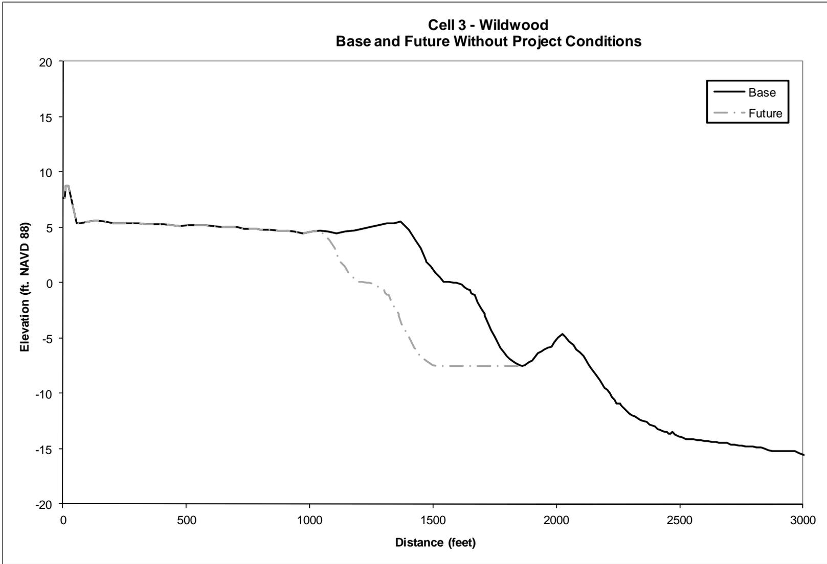
**Figure 24. Base and Future Without Project Conditions for Cell 3**
