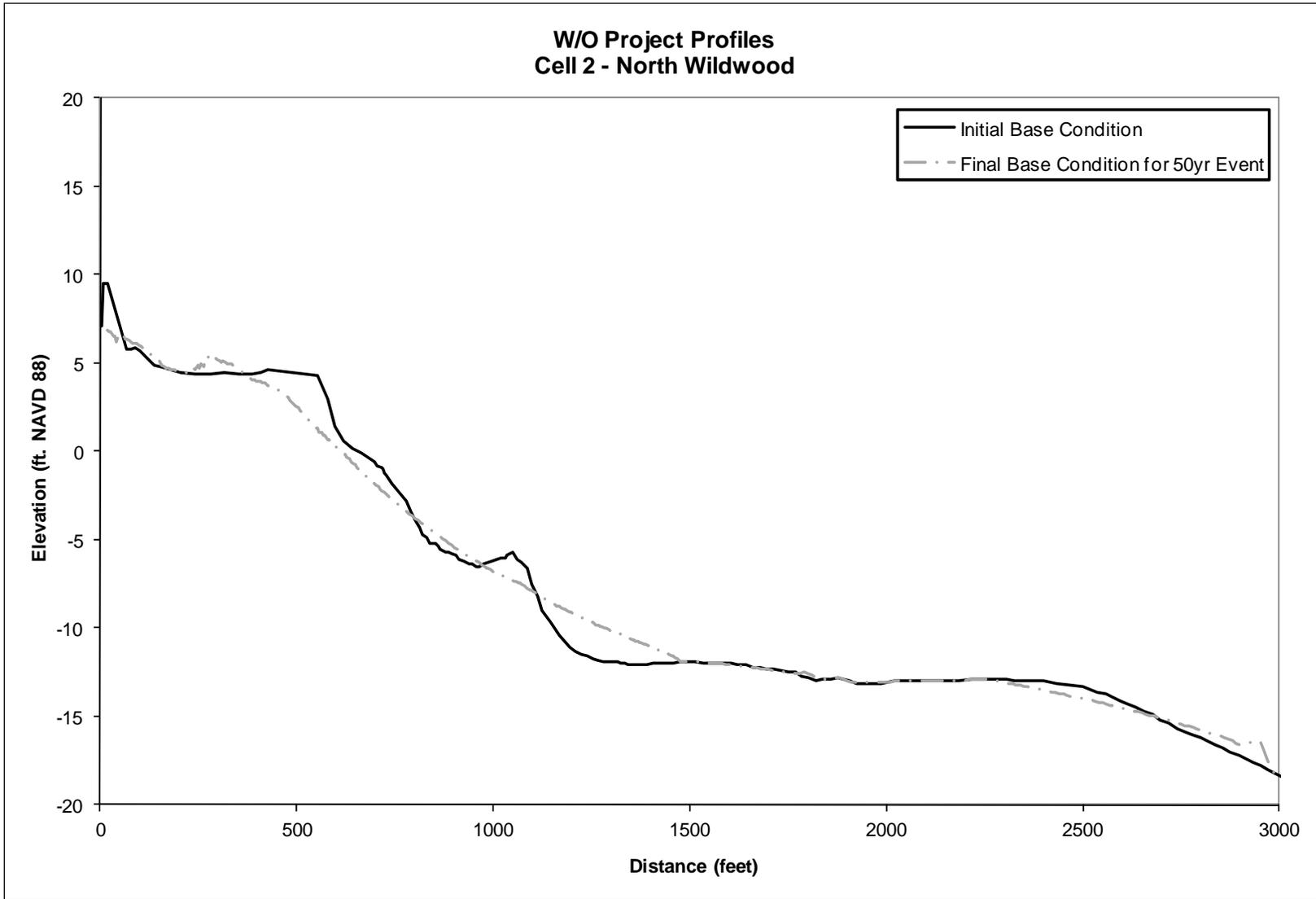
**Figure 37. Pre- and Post “50-yr” Storm Beach Profiles for Without Base Conditions in Cell 2**
