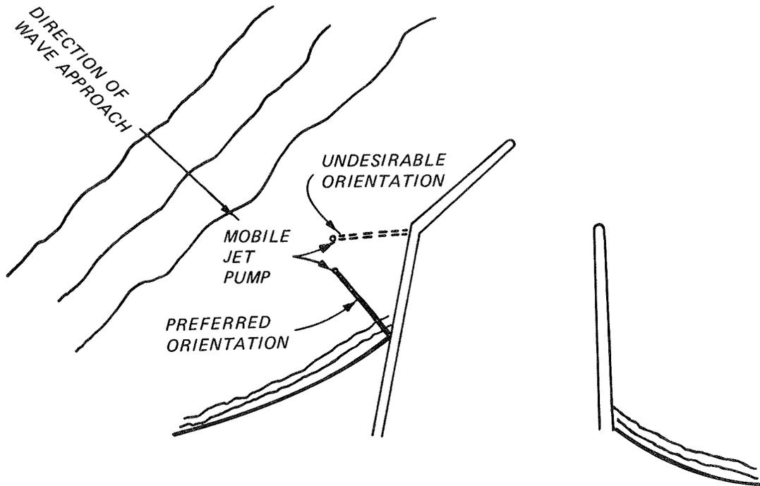
Figure 19. Orientation of mobile jet pump
