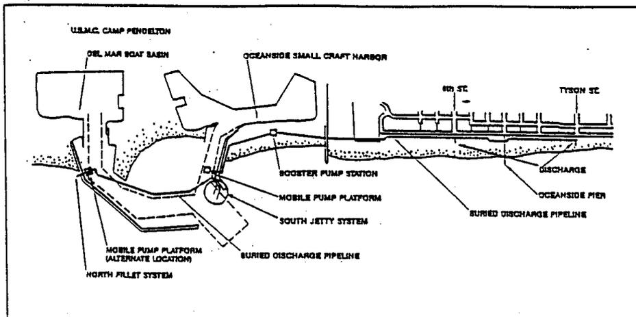
**Figure G2:** Oceanside Harbour Sand Bypassing System, Locality plan ( Weisman et al, 1996).
