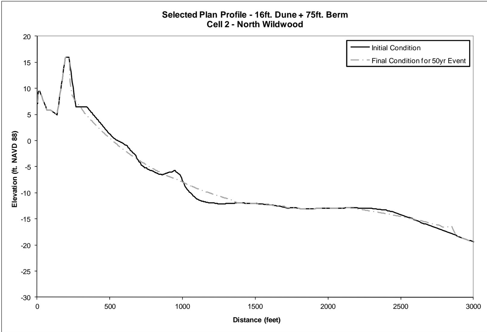
**Figure 53. Pre- and Post “50-yr” Storm Beach Profiles for Selected Plan in Cell 2**
