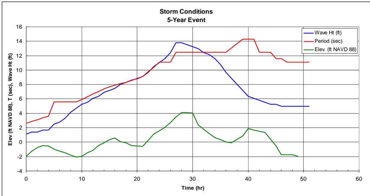
**Figure 29. “5-yr” Storm Conditions used in Storm Damage Analysis**
