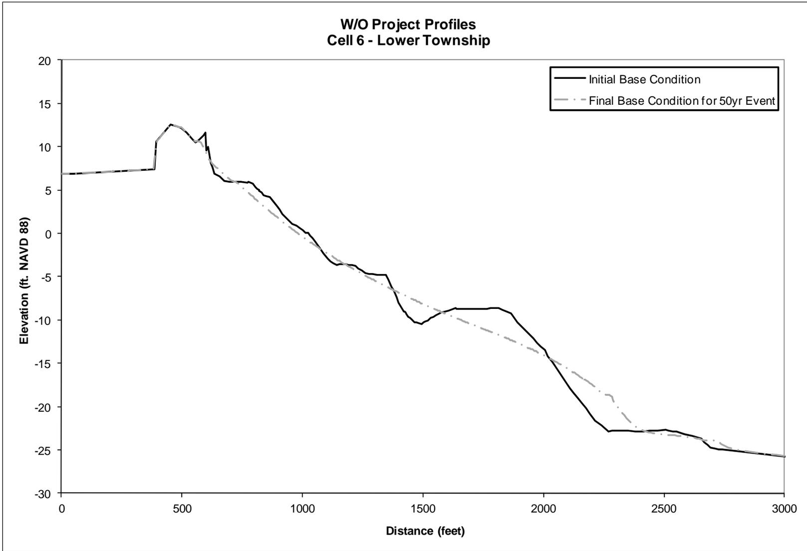
**Figure 41. Pre- and Post “50-yr” Storm Beach Profiles for Without Base Conditions in Cell 6**
