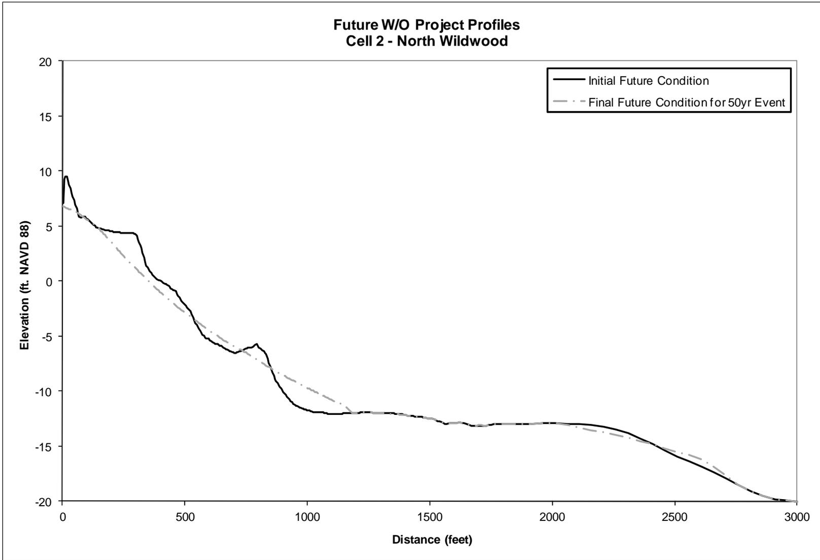
**Figure 44. Pre- and Post “50-yr” Storm Beach Profiles for Without Future Conditions in Cell 2**
