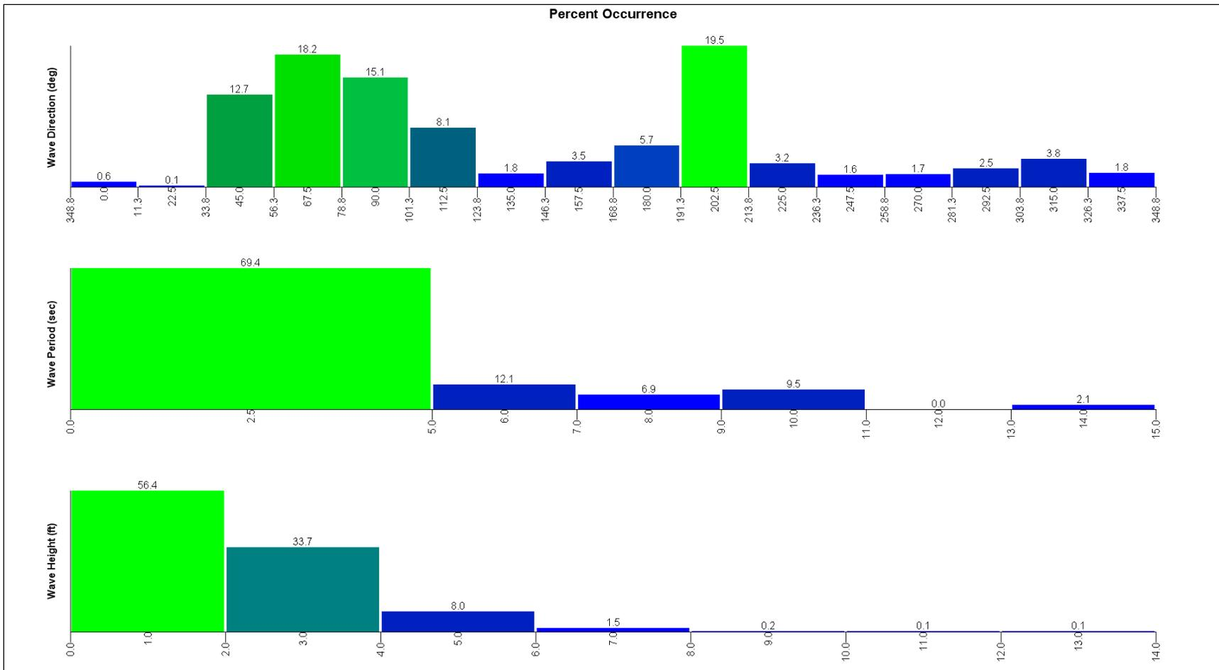
**Figure 4. OCTI Station I19J19 Percent Occurrence Wave Direction, Period, and Height Histograms (1987-1997)**
