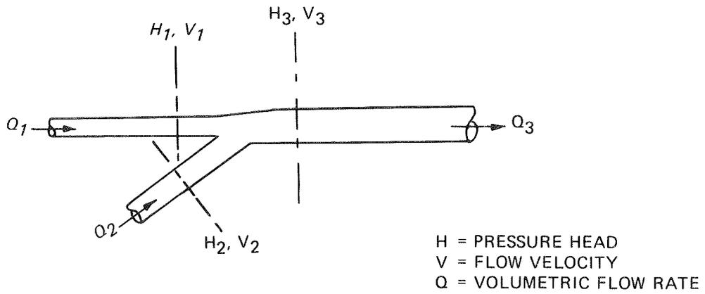
Figure 39. Junction of three pipes
