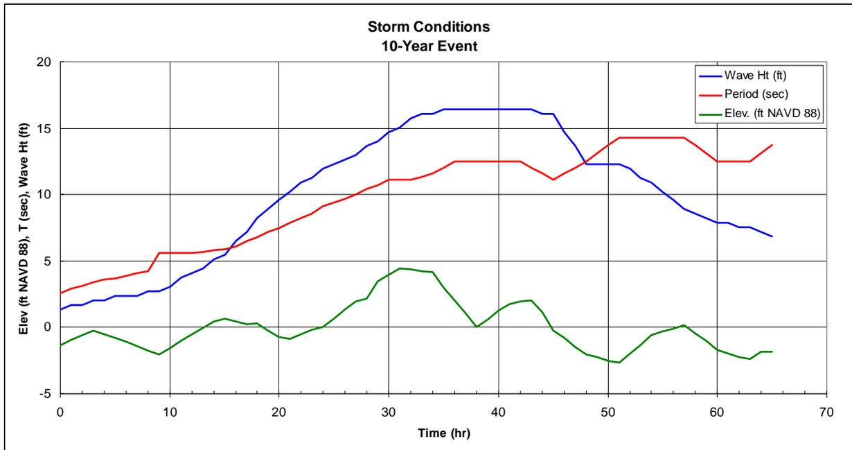
**Figure 30. “10-yr” Storm Conditions used in Storm Damage Analysis**
