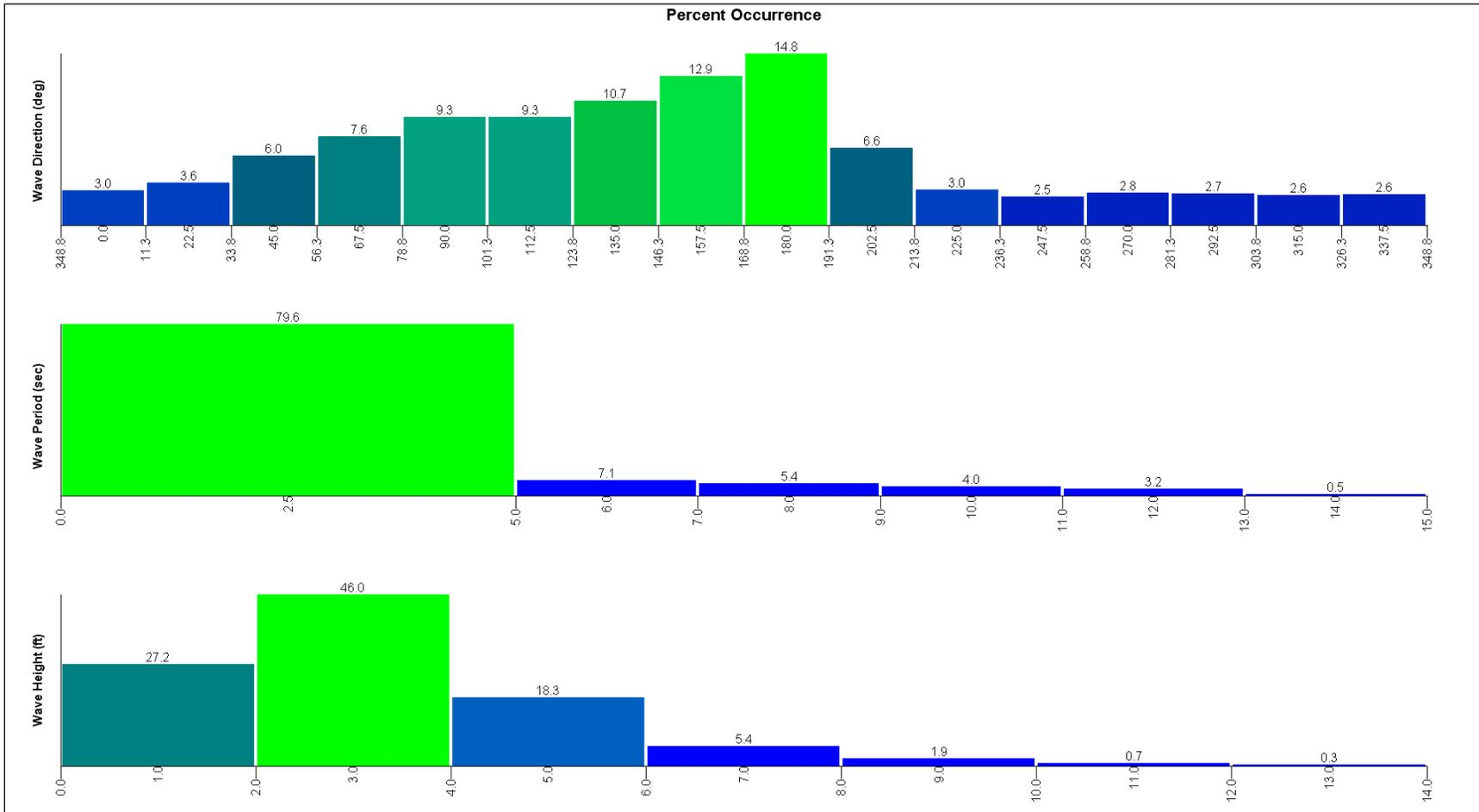
**Figure 2. WIS Station 147 Percent Occurrence Wave Direction, Period, and Height Histograms (1980-2000)**
