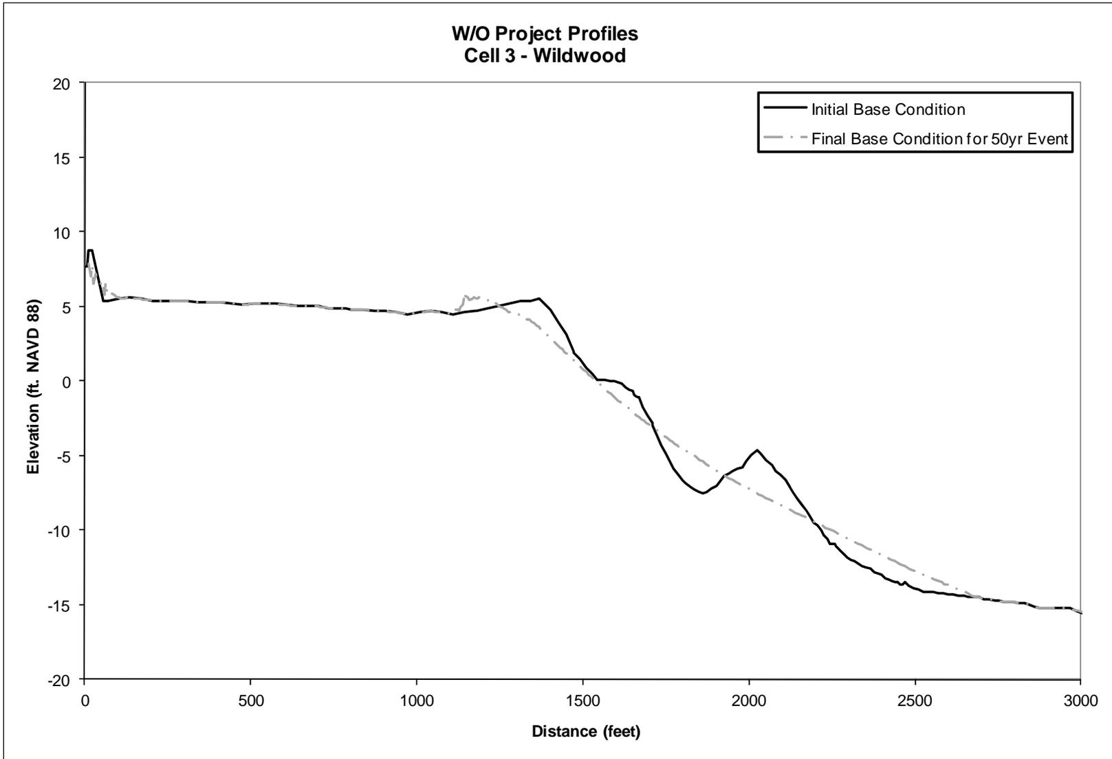
**Figure 38. Pre- and Post “50-yr” Storm Beach Profiles for Without Base Conditions in Cell 3**
