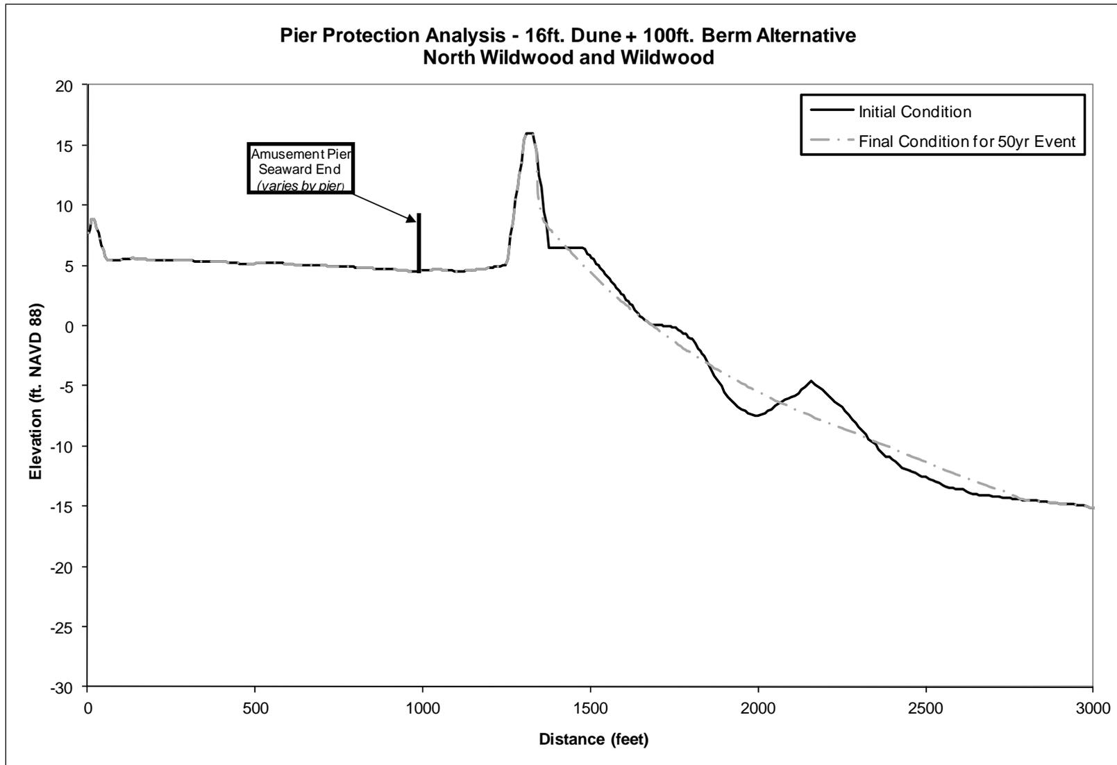
**Figure 50. Pre- and Post “50-yr” Storm Beach Profiles for 16 ft. Dune & 100 ft. Berm Pier Protection Alternative**
