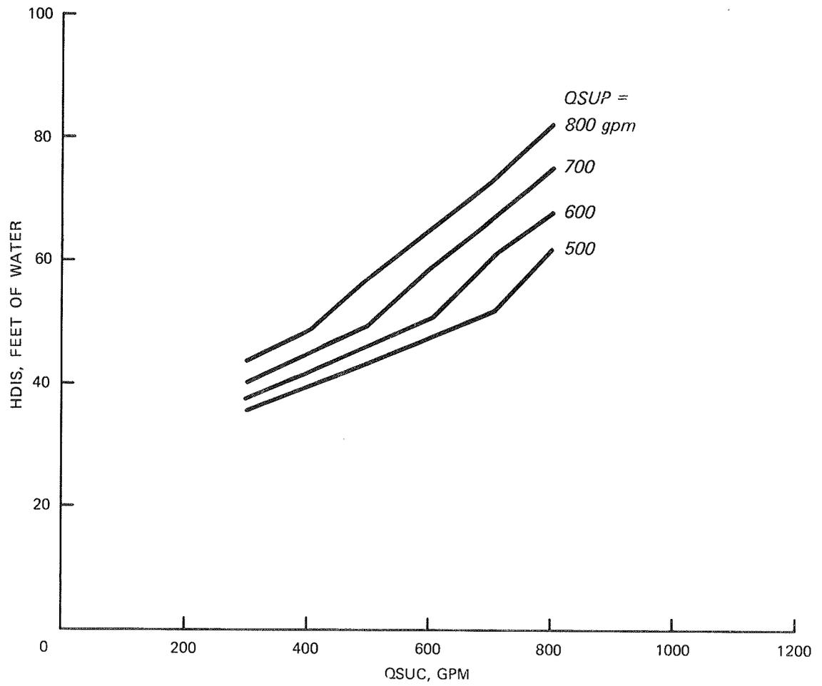
Figure 36. Example jet pump discharge pipeline curves for 6-in. pipe
