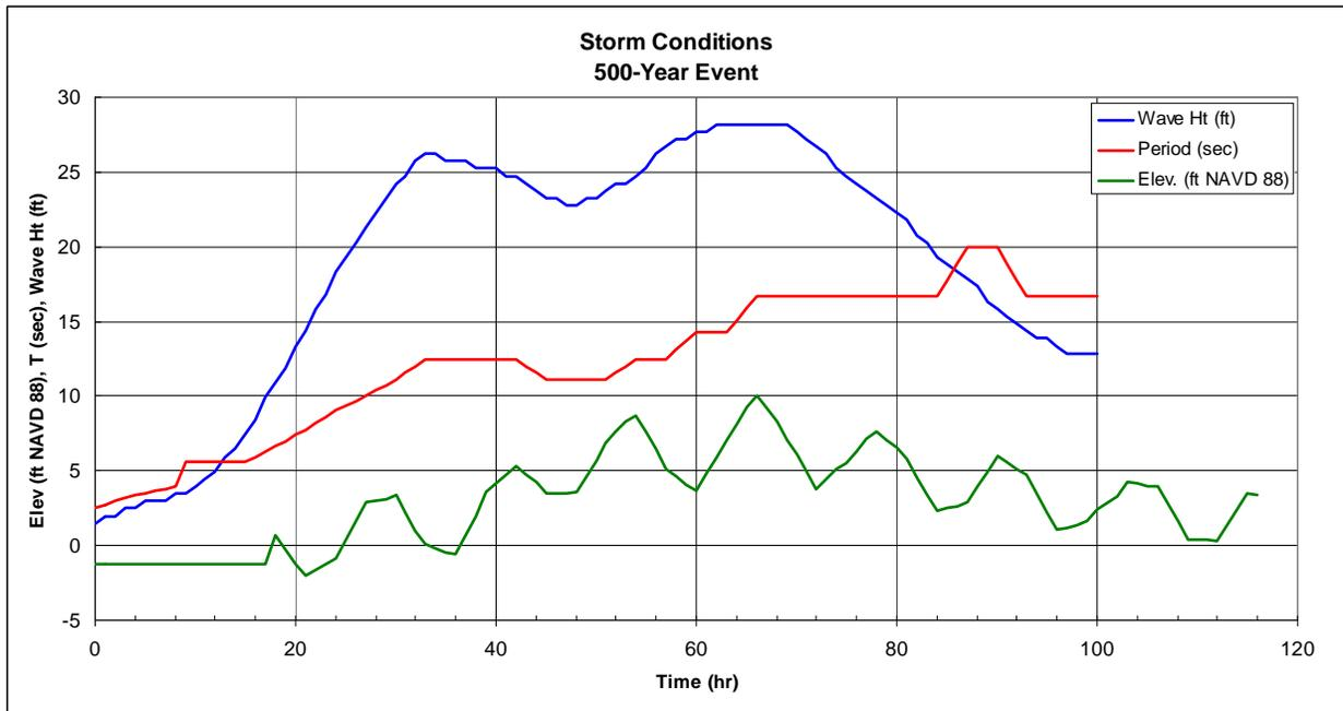
**Figure 35. “500-yr” Storm Conditions used in Storm Damage Analysis**
