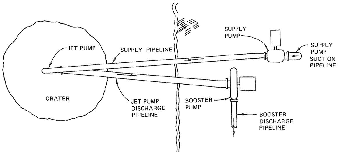
Figure 6. Plan view of simple jet pump system
