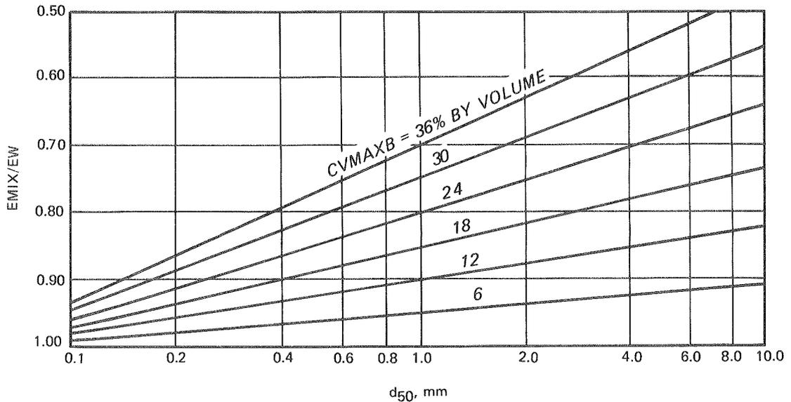
Figure 35. Ratio of efficiency mixture/efficiency water versus grain size (after Stepanoff 1969)
