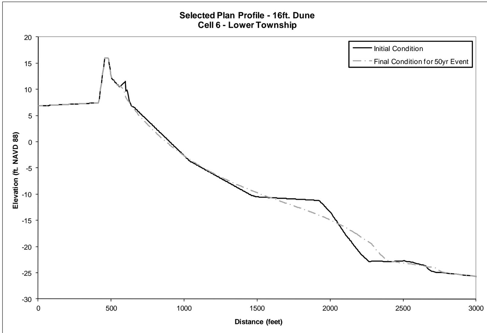
**Figure 57. Pre- and Post “50-yr” Storm Beach Profiles for Selected Plan in Cell 6**
