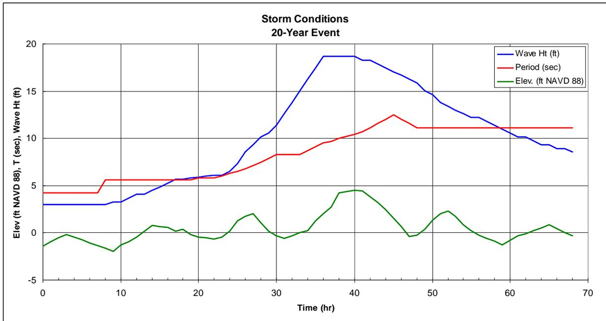
**Figure 31. “20-yr” Storm Conditions used in Storm Damage Analysis**
