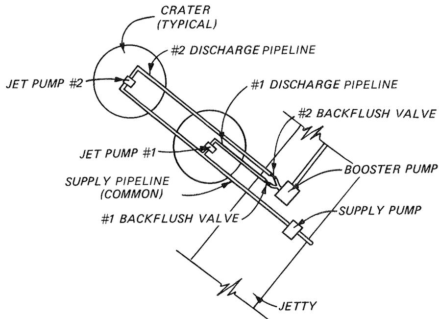
Figure 25. Two jet pumps with separate discharge pipelines
