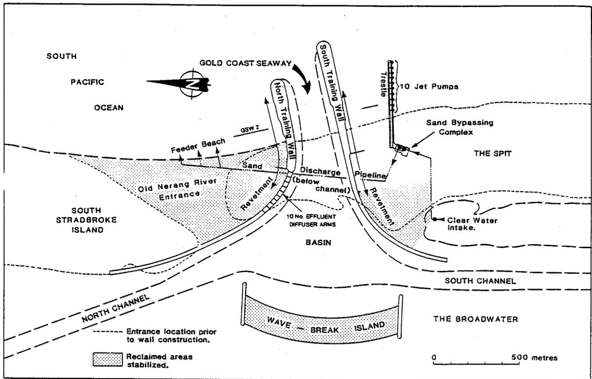
**Figure B3:** Schematic of Nerang River Entrance Sand Bypassing System (Witt and Hill, 1987).
