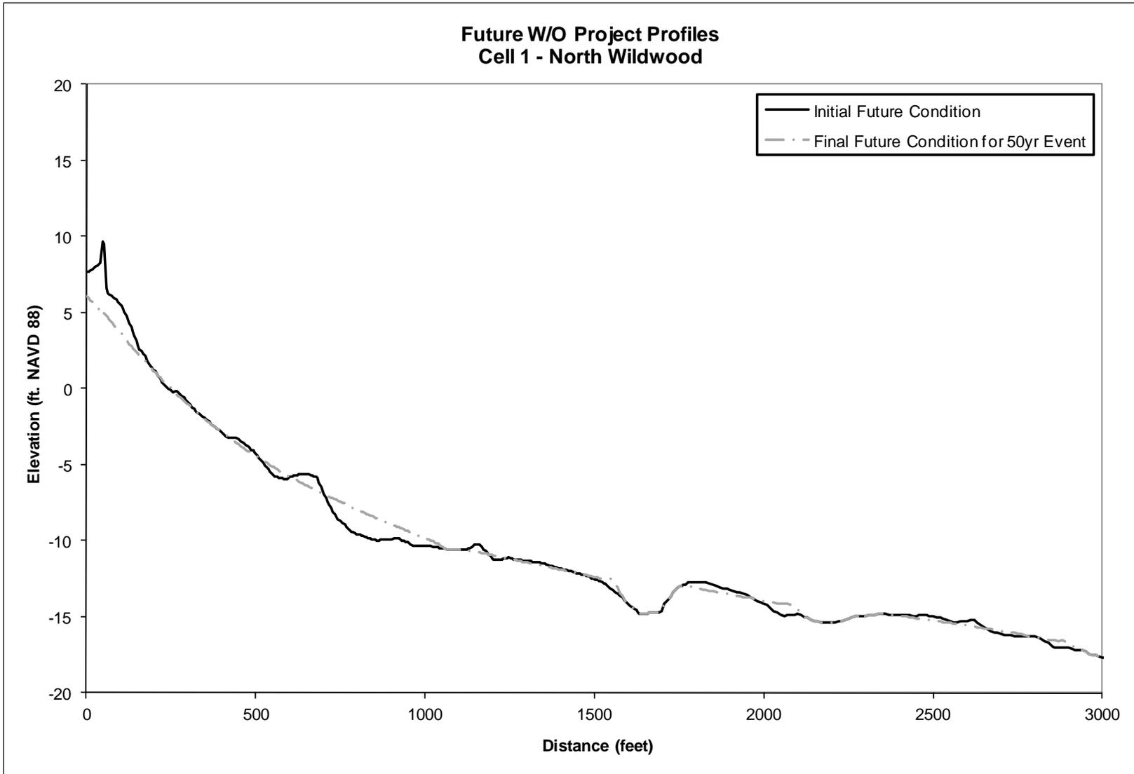
**Figure 43. Pre- and Post “50-yr” Storm Beach Profiles for Without Future Conditions in Cell 1**
