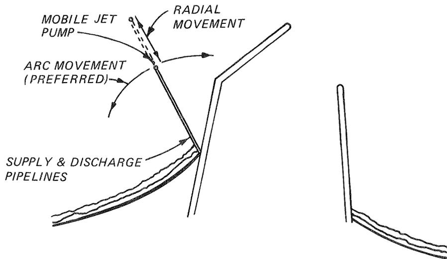
Figure 18. Movement of mobile jet pump
