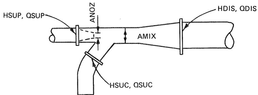
Figure 4. Location of jet pump parameters
