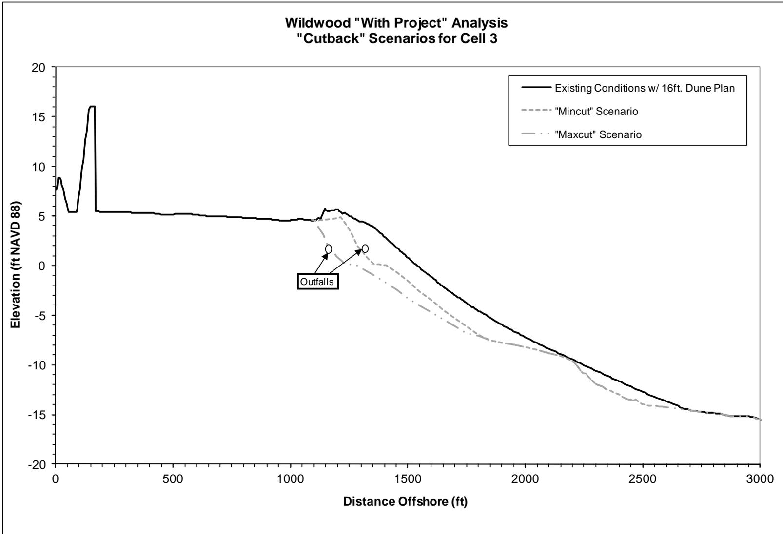
**Figure 51. Berm Cutback Alternatives Examined for With Project Analysis in Cell 3**
