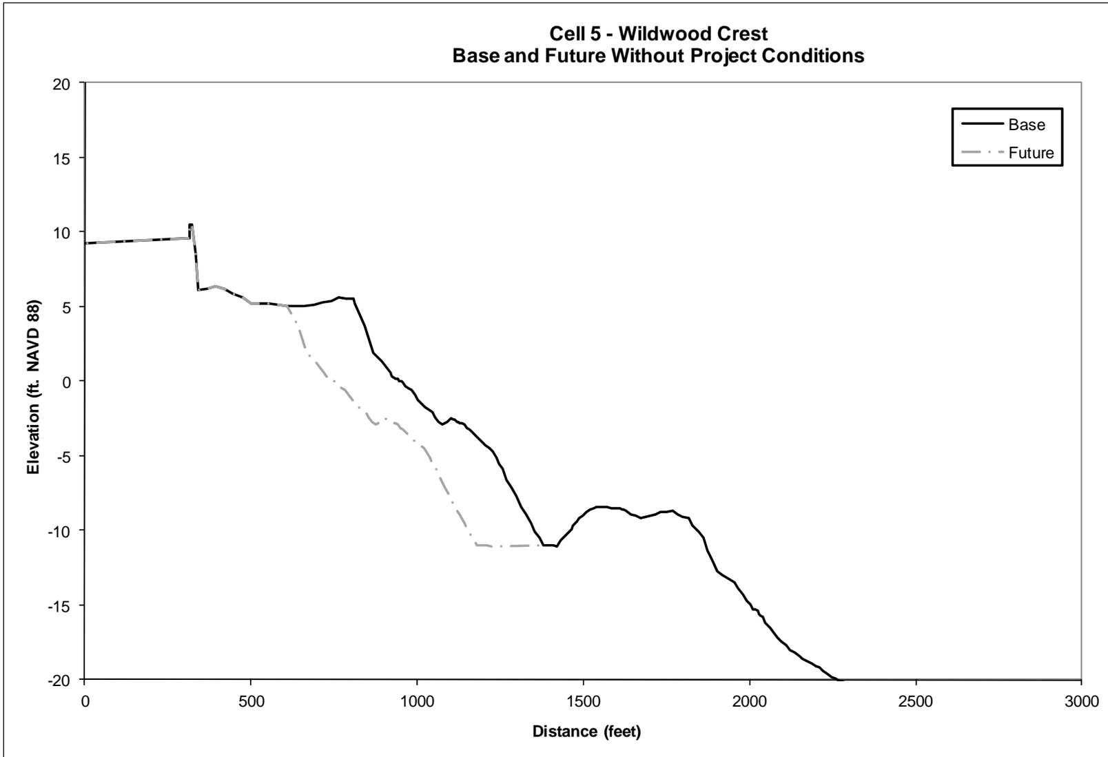
**Figure 26. Base and Future Without Project Conditions for Cell 5**
