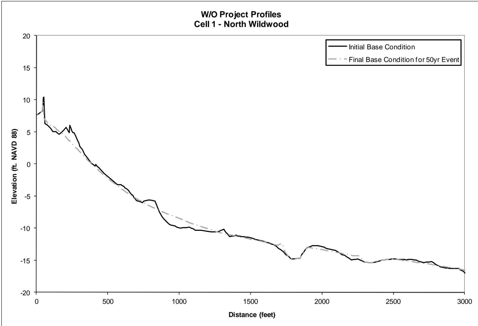
**Figure 36. Pre- and Post “50-yr” Storm Beach Profiles for Without Base Conditions in Cell 1**
