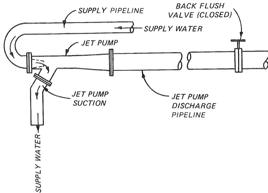
Figure 23. Jet pump backflushing
