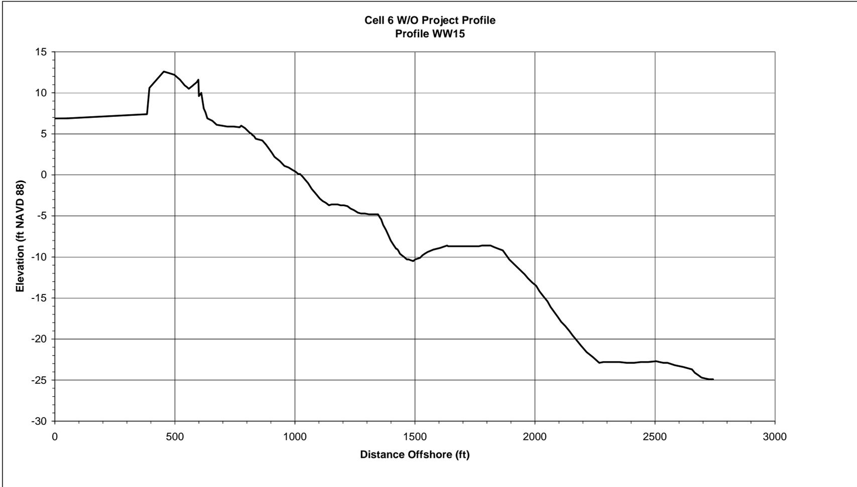
**Figure 19. W/O Project Conditions Profile for Cell 6**
