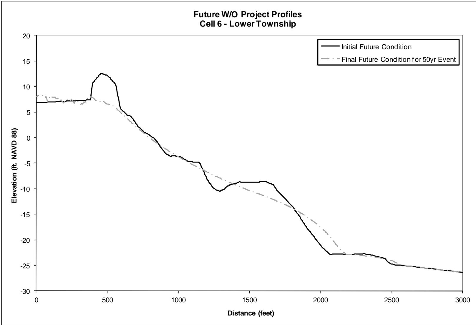
**Figure 48. Pre- and Post “50-yr” Storm Beach Profiles for Without Future Conditions in Cell 6**
