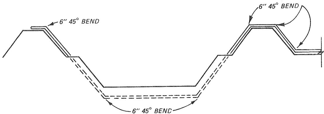
Figure 31. Booster discharge pipeline underchannel crossing (elevation view)
