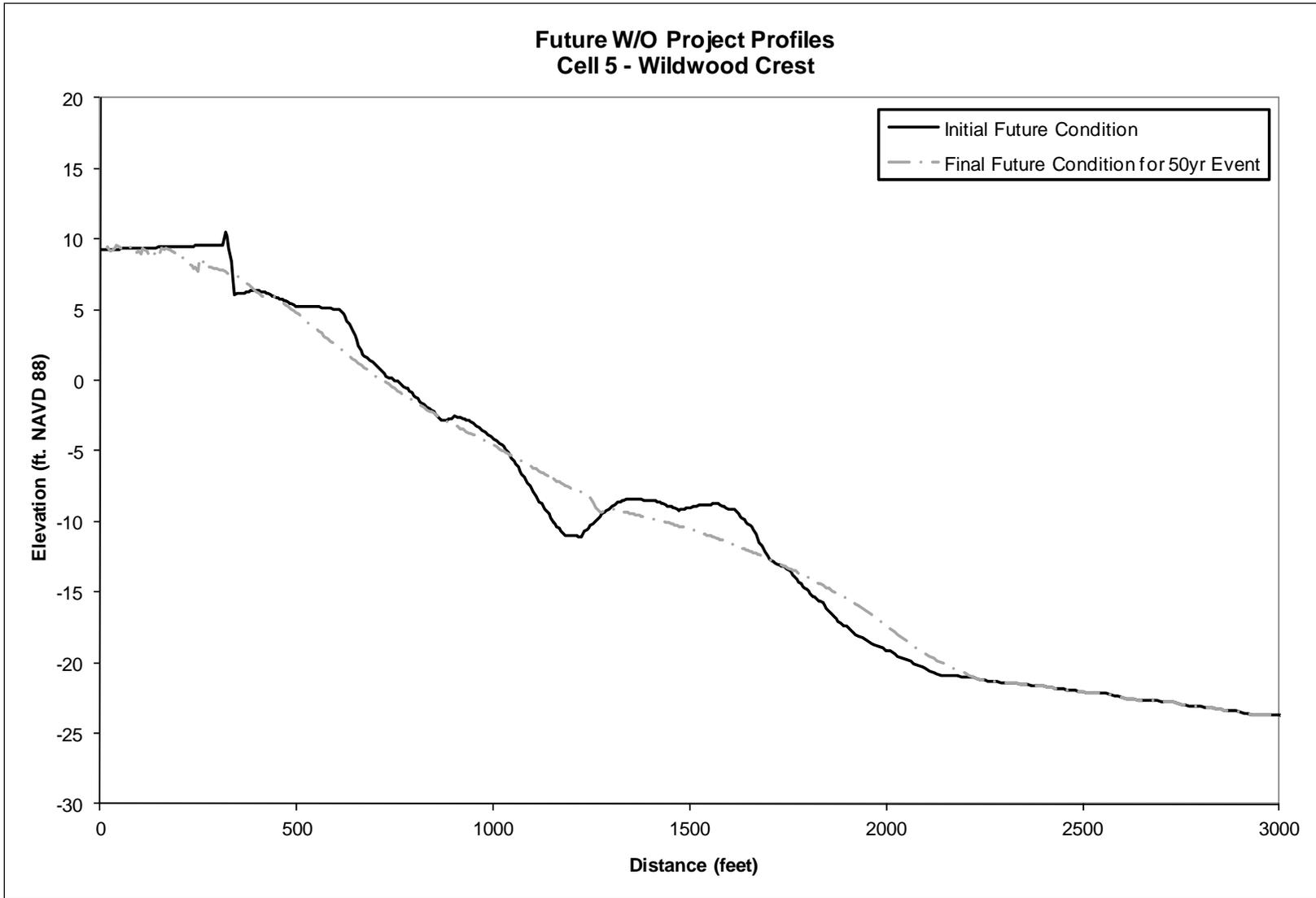
**Figure 47. Pre- and Post “50-yr” Storm Beach Profiles for Without Future Conditions in Cell 5**
