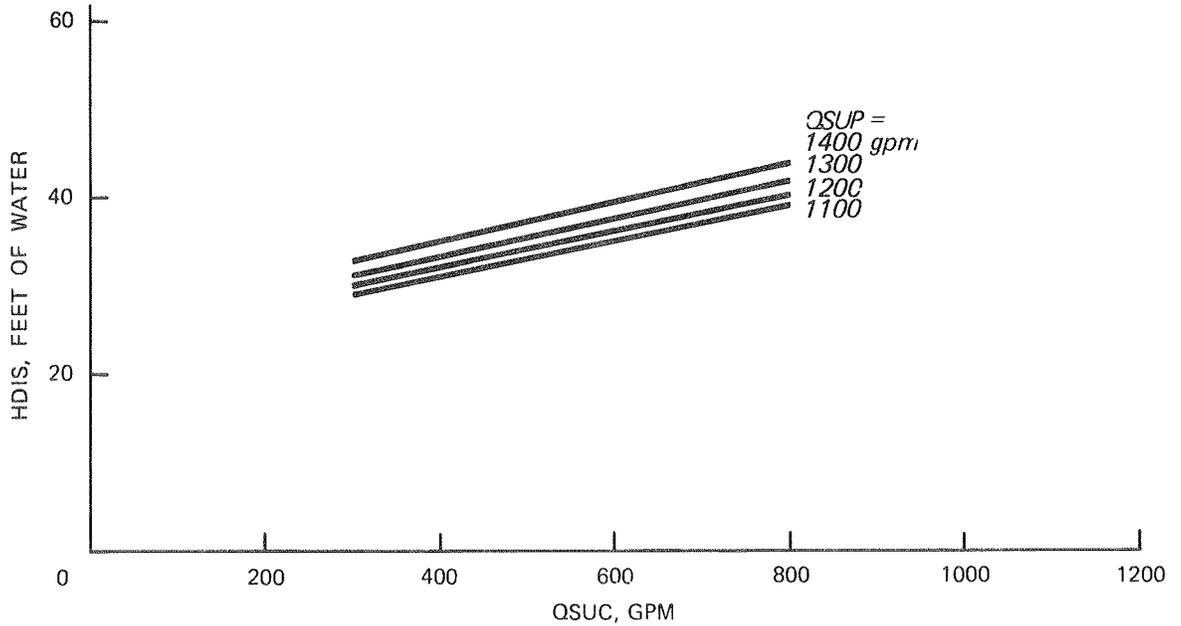
Figure 38. Example jet pump discharge pipeline curves for 8-in. pipe
