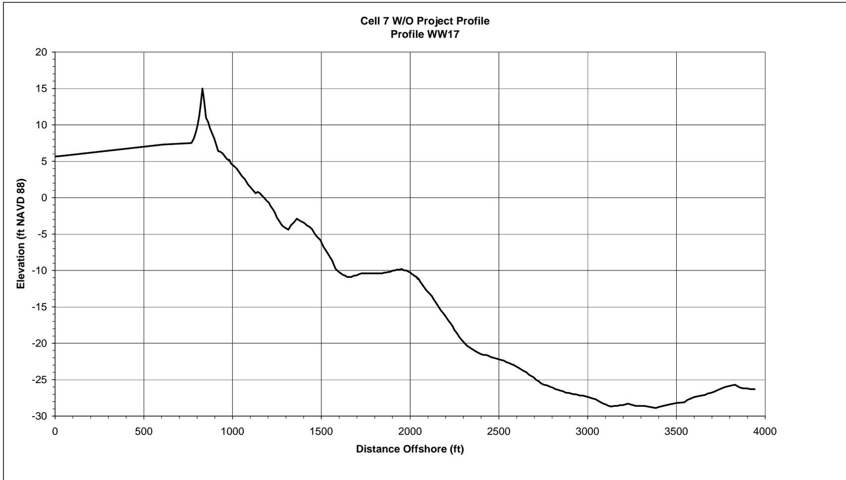
**Figure 20. W/O Project Conditions Profile for Cell 7**
