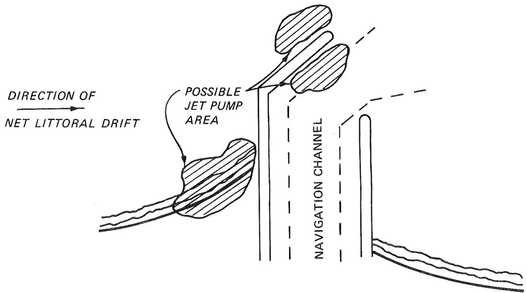
Figure 14. Shore-connected breakwater and jetties
