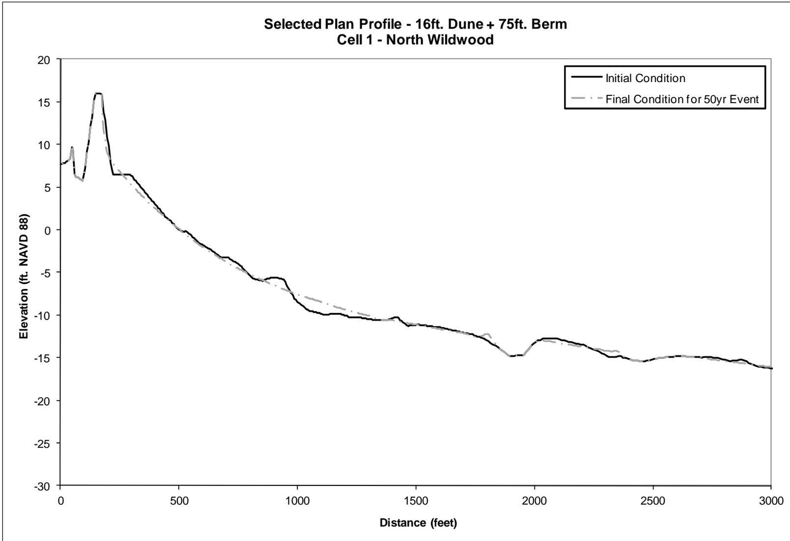
**Figure 52. Pre- and Post “50-yr” Storm Beach Profiles for Selected Plan in Cell 1**
