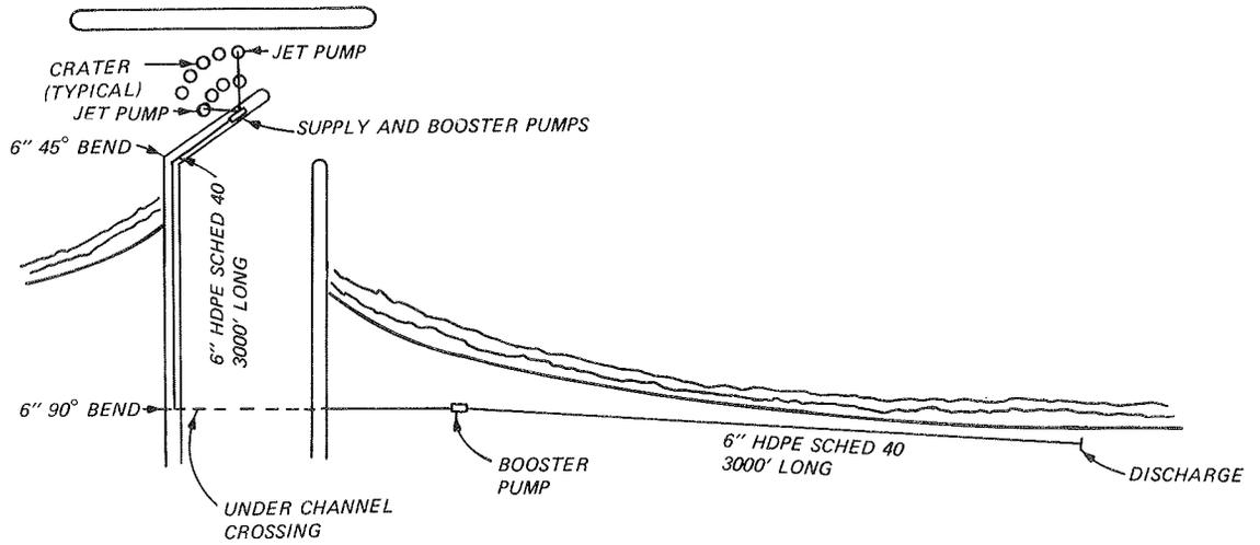
Figure 27. Overall system schematic
