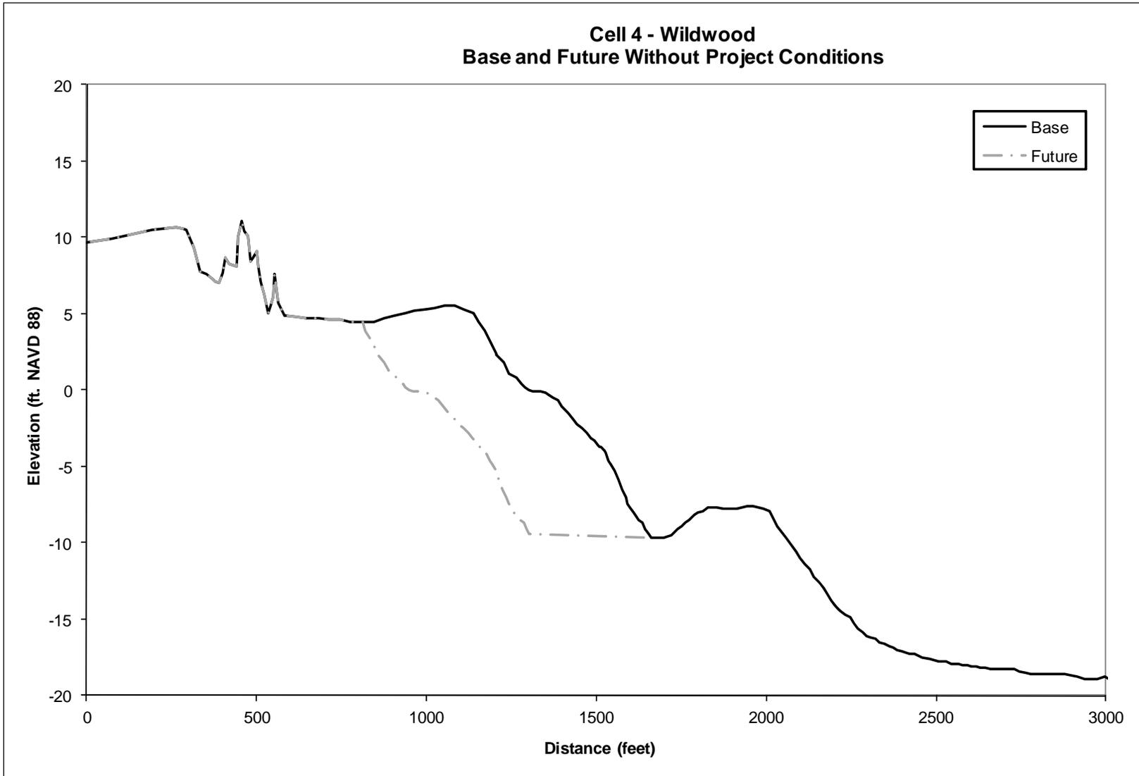
**Figure 25. Base and Future Without Project Conditions for Cell 4**
