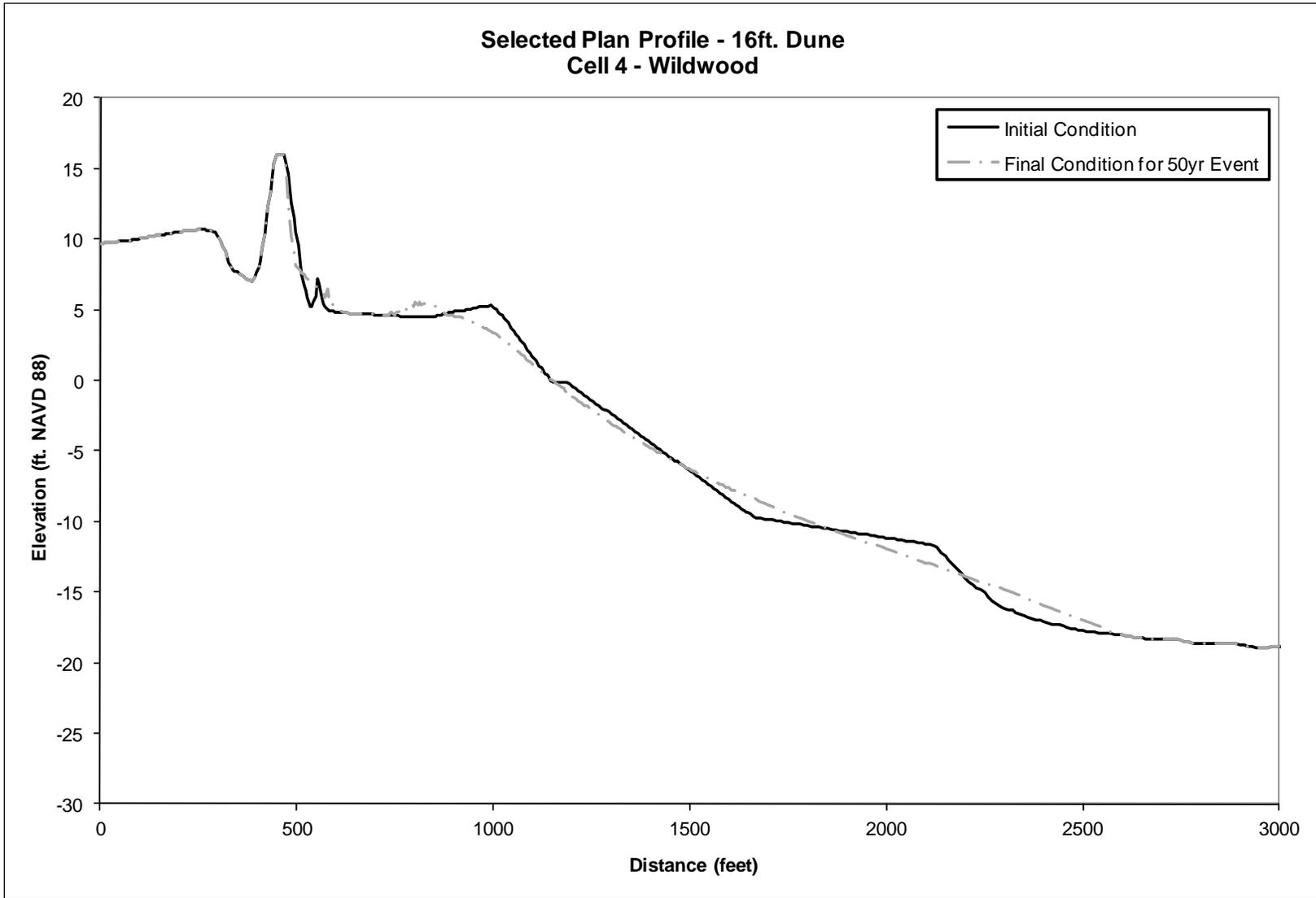
**Figure 55. Pre- and Post “50-yr” Storm Beach Profiles for Selected Plan in Cell 4**
