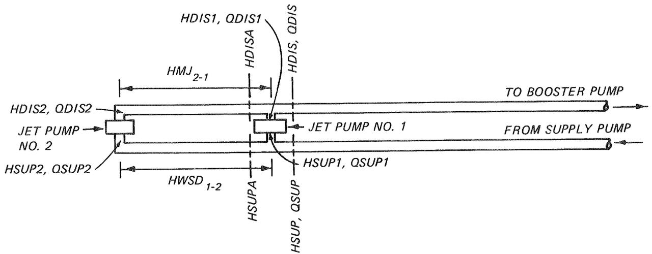
Figure 40. Dual jet pump system
