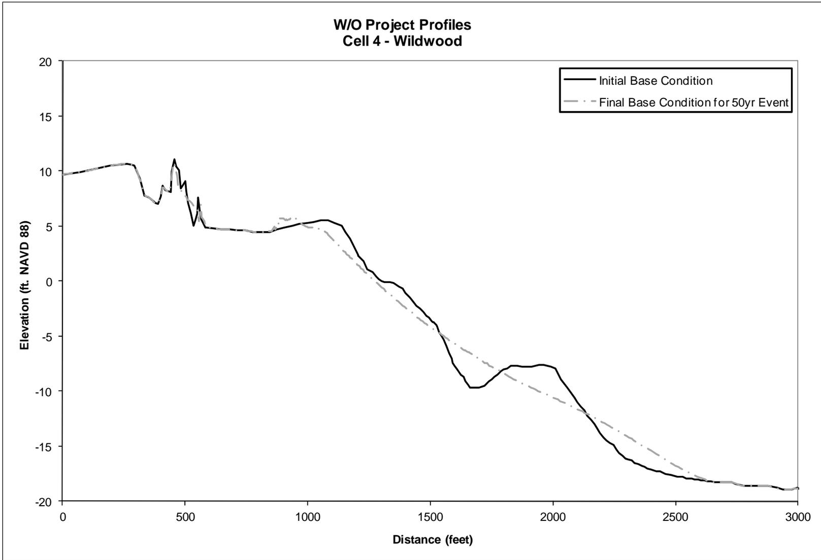
**Figure 39. Pre- and Post “50-yr” Storm Beach Profiles for Without Base Conditions in Cell 4**
