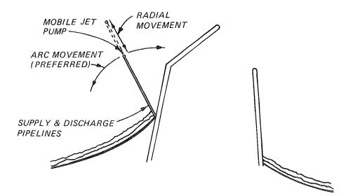
Figure 18. Movement of mobile jet pump
