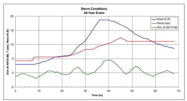
Figure 31. "20-yr" Storm Conditions used in Storm Damage Analysis
