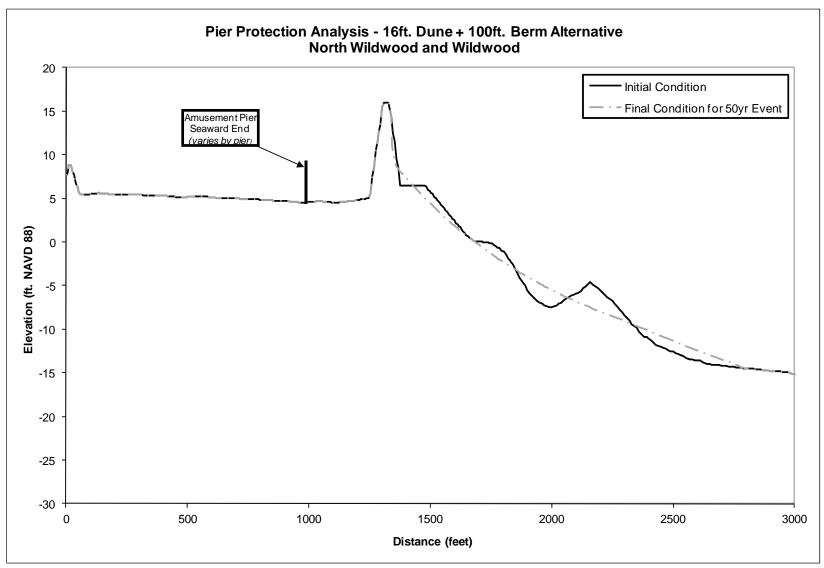
Figure 50. Pre- and Post "50-yr" Storm Beach Profiles for 16 ft. Dune & 100 ft. Berm Pier Protection Alternative
