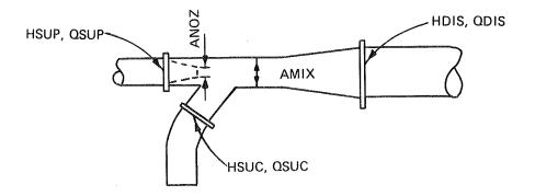
Figure 4. Location of jet pump parameters
