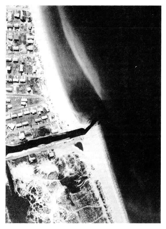
Figure 1. Aerial view of Mexico Beach, Florida, showing updrift accretion, downdrift erosion, and channel shoaling
