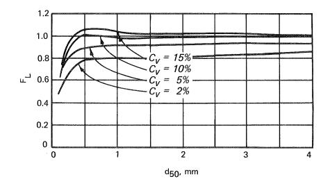
Figure 33. F<sub>L</sub> versus d<sub>50</sub> for Durand relationship (from Hydraulics of Sediment Transport by Graf (1971). C1971 by McGraw-Hill Inc. Used with permission of McGraw-Hill Book Company)
