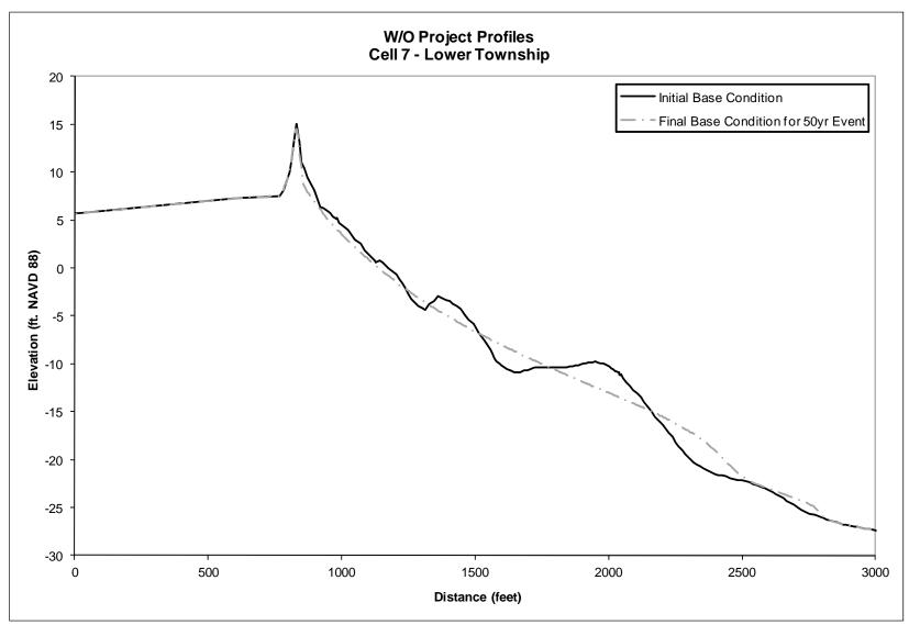
Figure 42. Pre- and Post "50-yr" Storm Beach Profiles for Without Base Conditions in Cell 7
