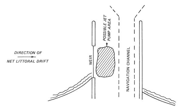
Figure 15. Jetties with weir section
