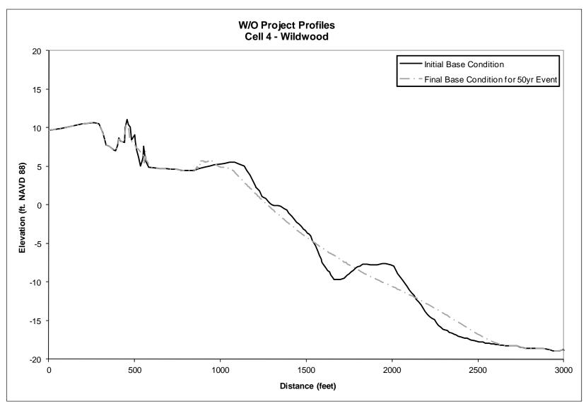
Figure 39. Pre- and Post "50-yr" Storm Beach Profiles for Without Base Conditions in Cell 4
