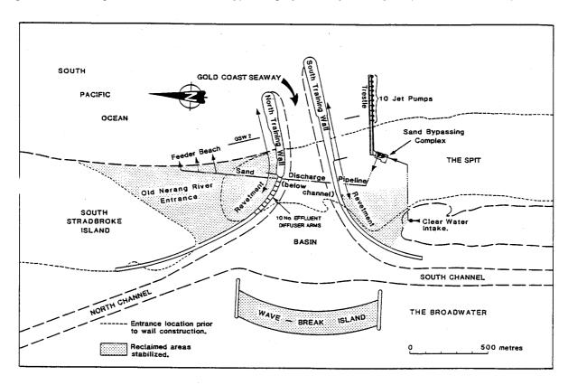
Figure B2: Nerang River Entrance Sand Bypassing System, System layout (Witt and Hill, 1987).
