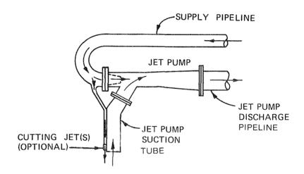
Figure 7. Elevation view of jet pump
