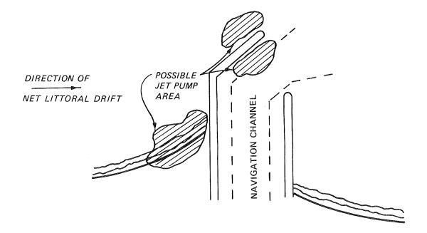
Figure 14. Shore-connected breakwater and jetties
