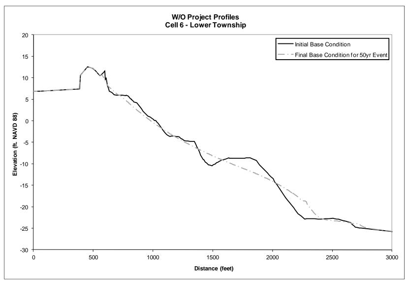
Figure 41. Pre- and Post "50-yr" Storm Beach Profiles for Without Base Conditions in Cell 6
