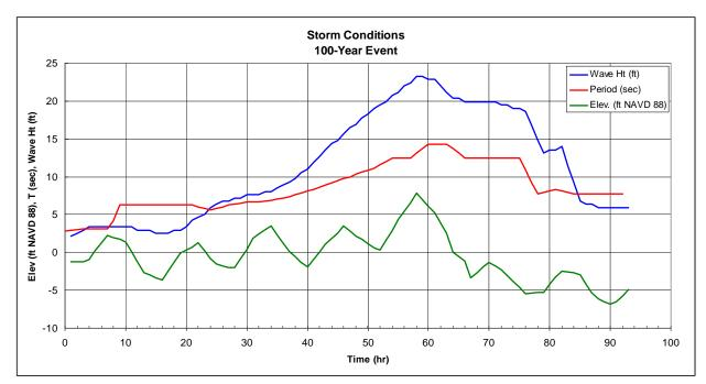
Figure 33. "100-yr" Storm Conditions used in Storm Damage Analysis
