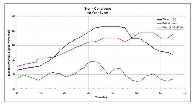
Figure 30. "10-yr" Storm Conditions used in Storm Damage Analysis
