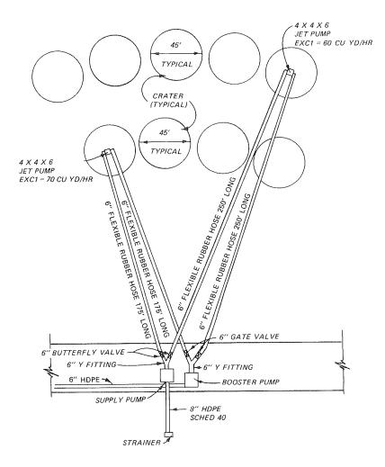
Figure 28. Detailed schematic - jet, supply, and booster pumps (plan view)
