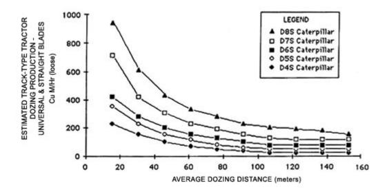
Figure 5. Maximum production rates for different bulldozers equipped with straight blades in relation to haul distance (from Caterpillar Handbook, 1984).
