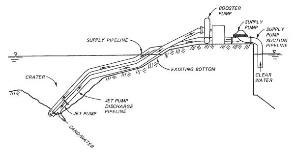
Figure 5. Elevation view of simple jet pump system
