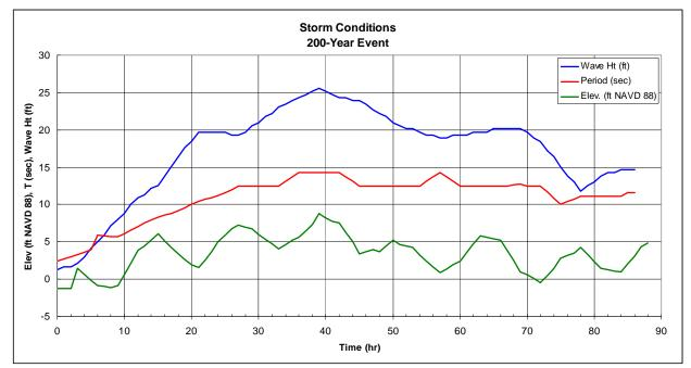
Figure 34. "200-yr" Storm Conditions used in Storm Damage Analysis
