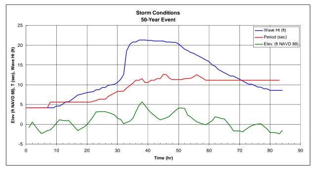
Figure 32. "50-yr" Storm Conditions used in Storm Damage Analysis
