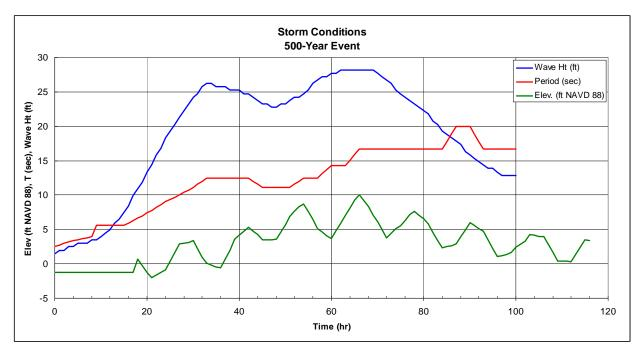
Figure 35. "500-yr" Storm Conditions used in Storm Damage Analysis
