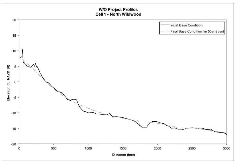
Figure 36. Pre- and Post "50-yr" Storm Beach Profiles for Without Base Conditions in Cell 1
