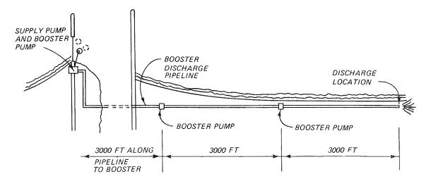
Figure 21. Example arrangement of multiple boosters on 9000-ft-long discharge line for 0.20-mm sand
