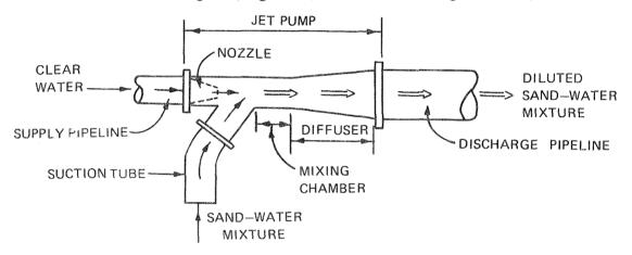
Figure 3. Jet pump principles of operation
