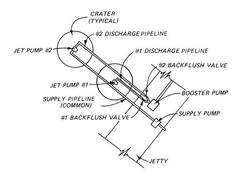
Figure 25. Two jet pumps with separate discharge pipelines
