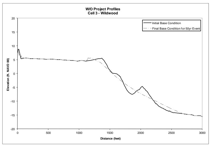
Figure 38. Pre- and Post "50-yr" Storm Beach Profiles for Without Base Conditions in Cell 3
