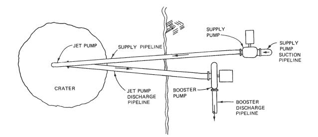
Figure 6. Plan view of simple jet pump system
