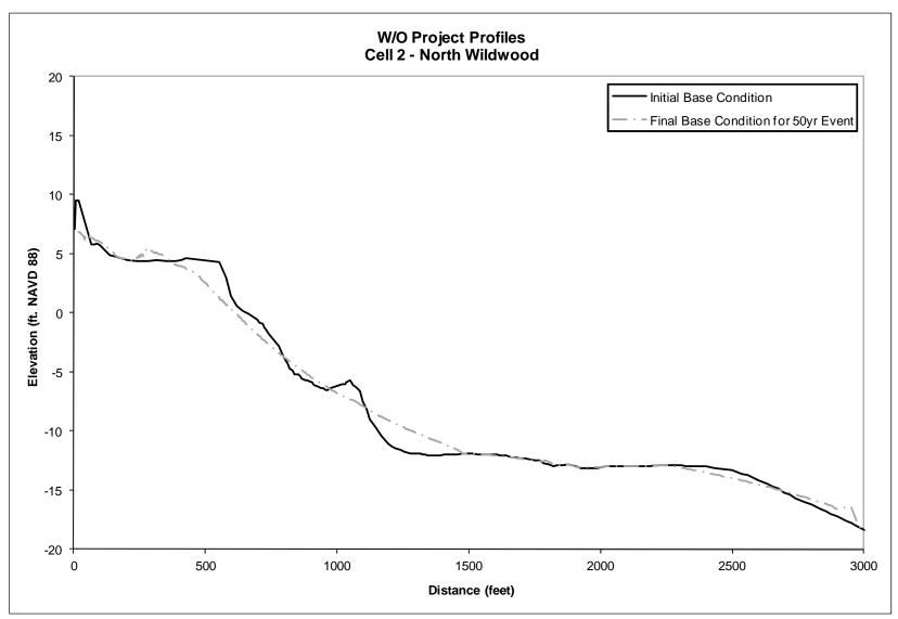
Figure 37. Pre- and Post "50-yr" Storm Beach Profiles for Without Base Conditions in Cell 2
