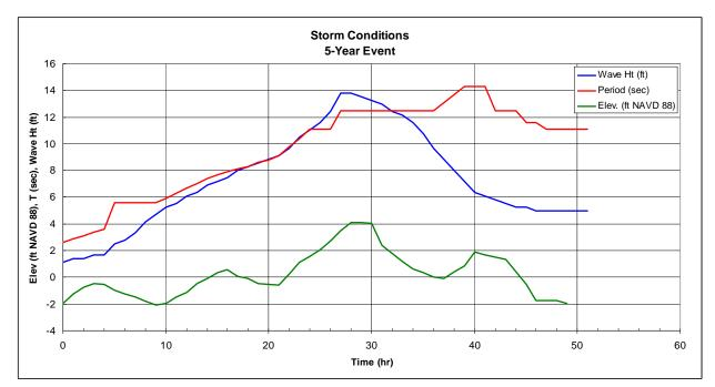
Figure 29. "5-yr" Storm Conditions used in Storm Damage Analysis
