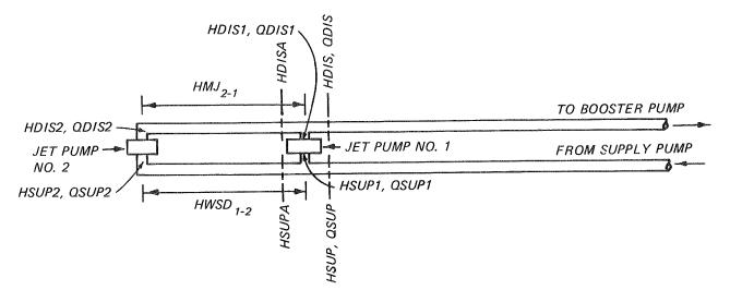
Figure 40. Dual jet pump system
