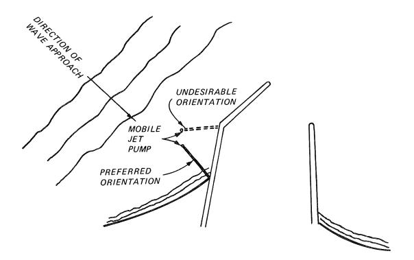
Figure 19. Orientation of mobile jet pump
