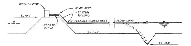
Figure 30. Jet pump discharge system (elevation view)
