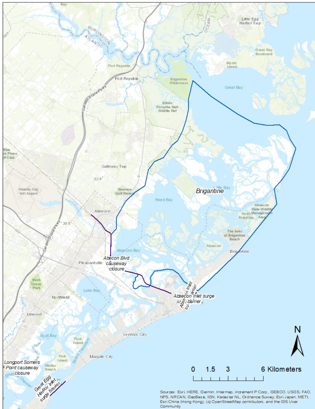
Figure 7 Configuration 5 included NNBF within the Brigantine NNBF area as well as a surge barrier at Absecon Inlet
