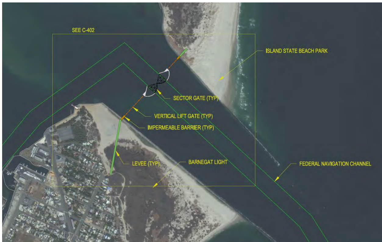
Figure 22: Storm Surge Barrier Example Design – Barnegat Inlet
