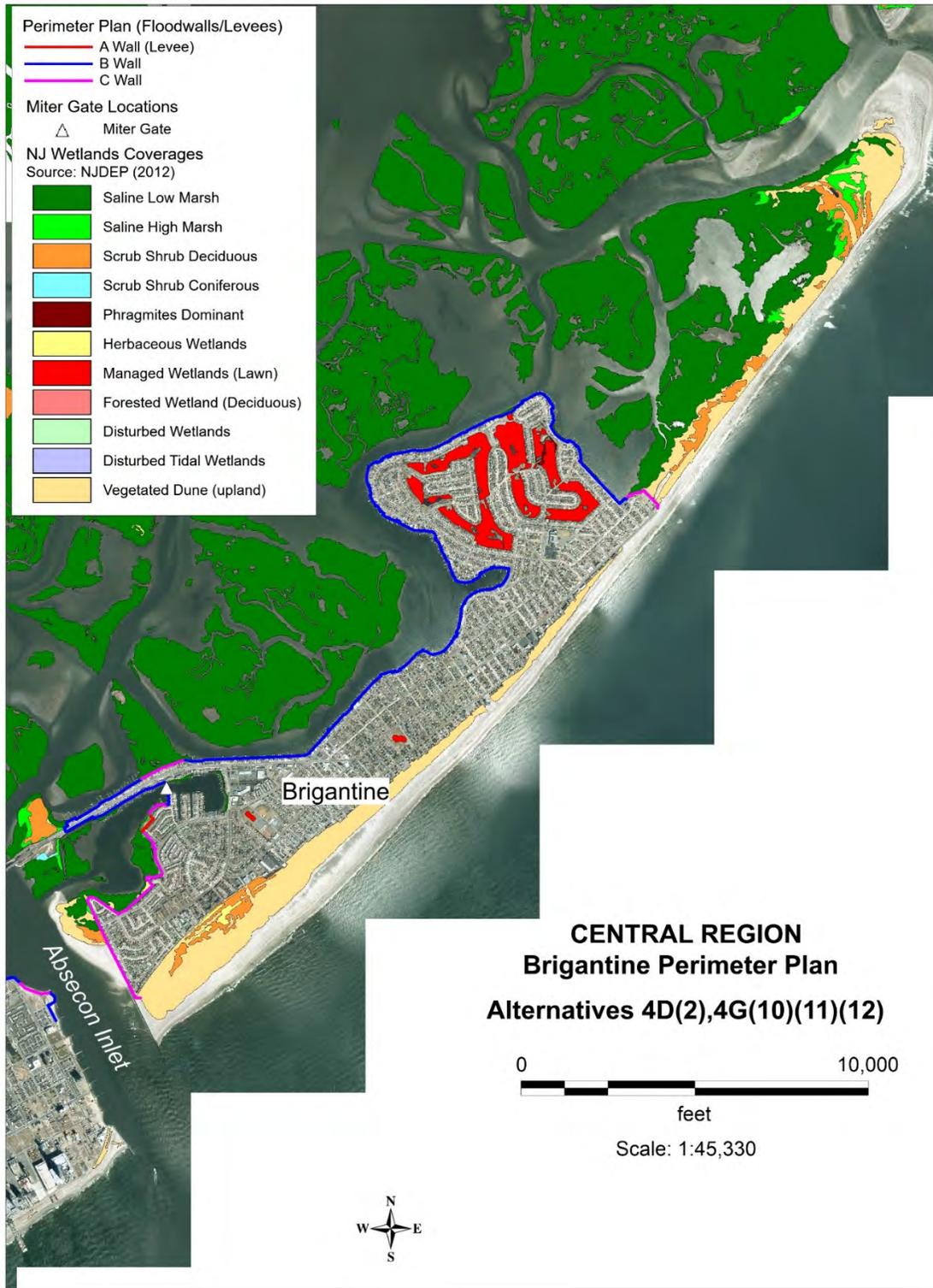
Figure 37: Perimeter Plan Overlay with Wetland Habitats along Brigantine Alignment in Alternatives 4D(2), 4G(10), 4G(11), and 4G(12)
