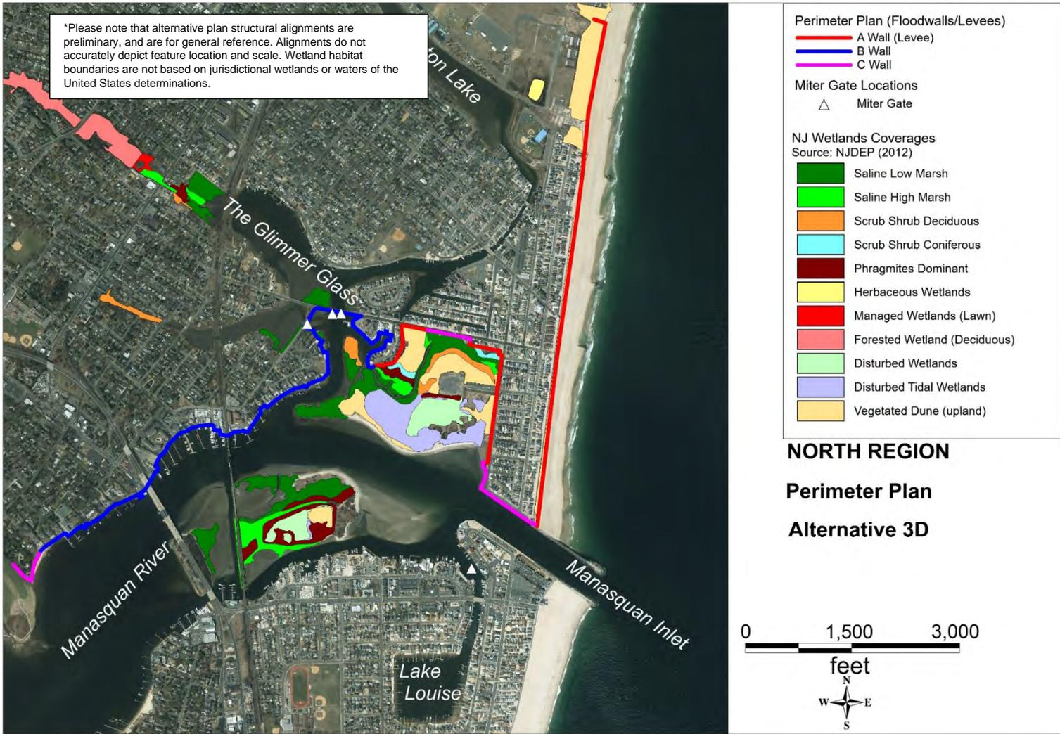
Figure 26: Perimeter Plan Overlay with Wetland Habitats along Manasquan Perimeter Plan Alignment in Alternative 3D
