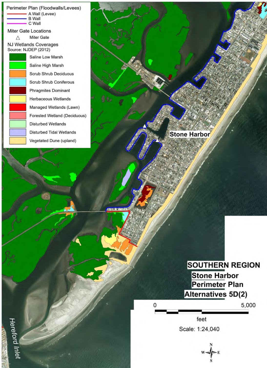
Figure 57: Perimeter Plan Overlay with Wetland Habitats along Stone Harbor Alignment in Alternatives 5D(2)
