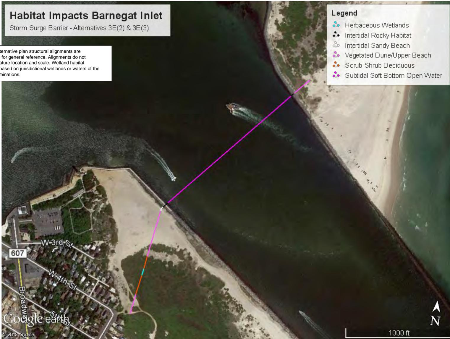
Figure 31: Habitat Impacts along Barnegat Inlet Storm Surge Barrier Plan Alignment in Alternatives 3E(2) and 3E(3)
