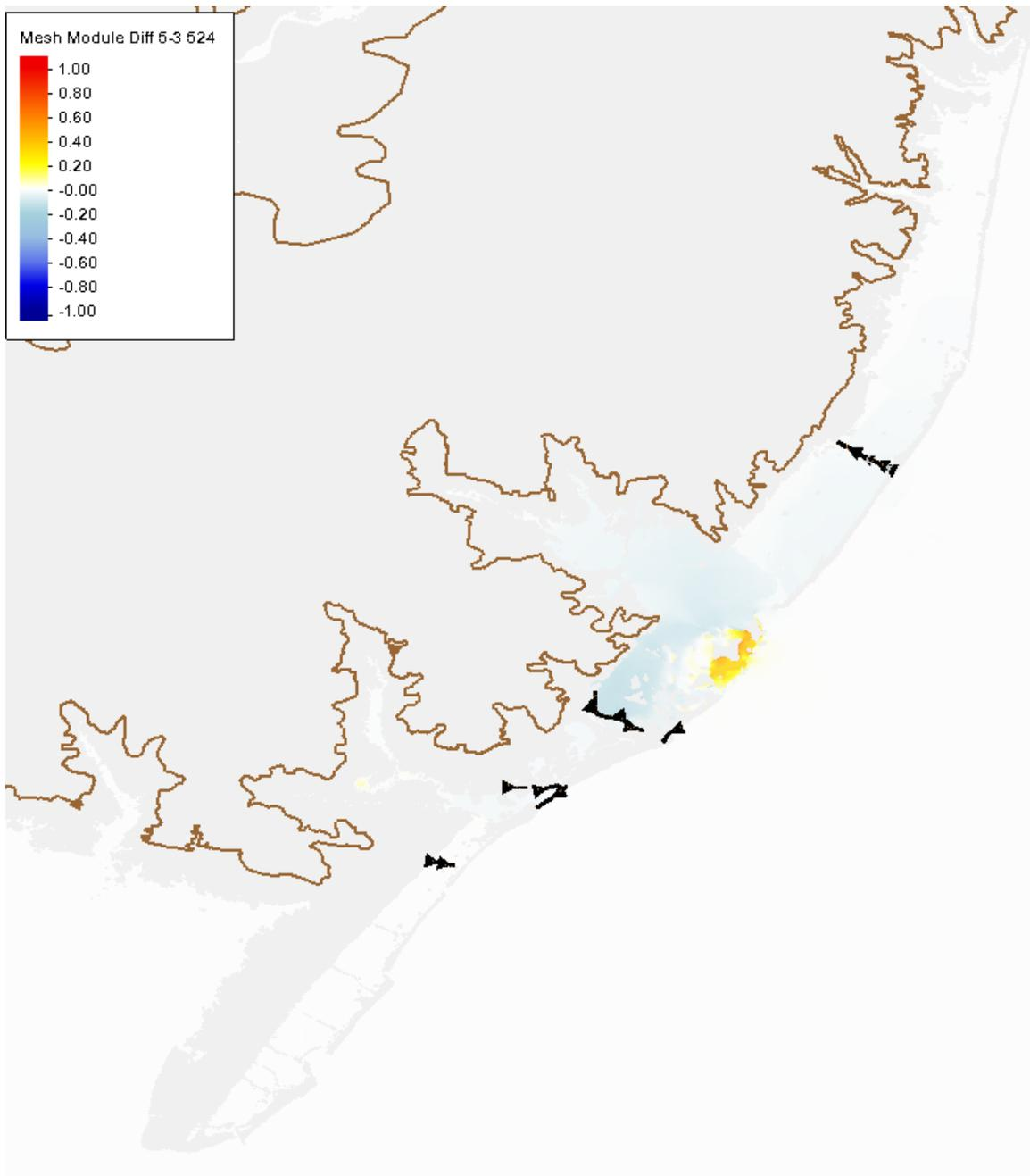
**Figure 47 Peak water level differences between Configuration 5 (Brigantine area NNBF) and Configuration 3 (structural only) for storm 524**
