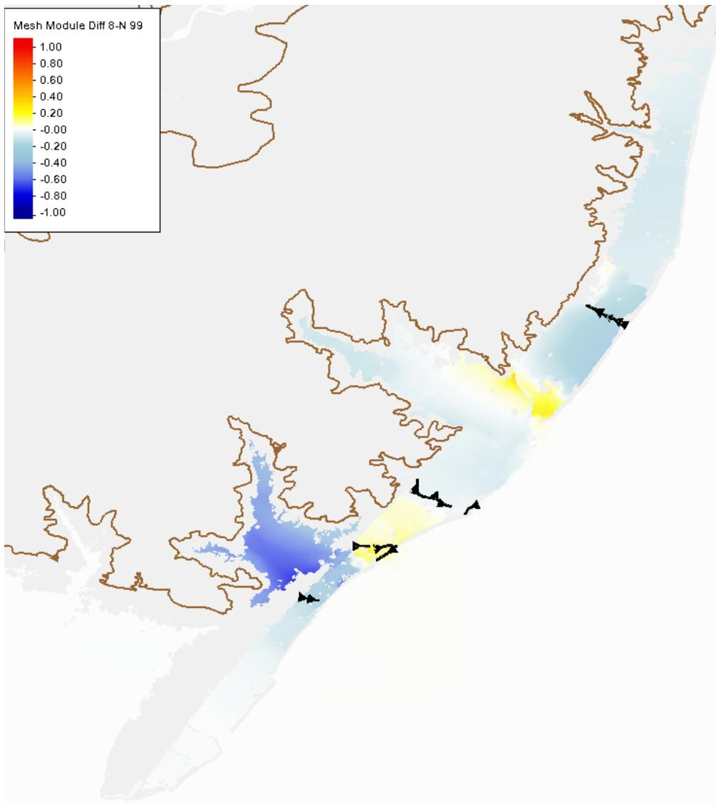
**Figure 50 Peak water level differences between Configuration 8 (Holgate and Great Egg Harbor area NNBF) and North Configuration (structural only) for storm 99**
