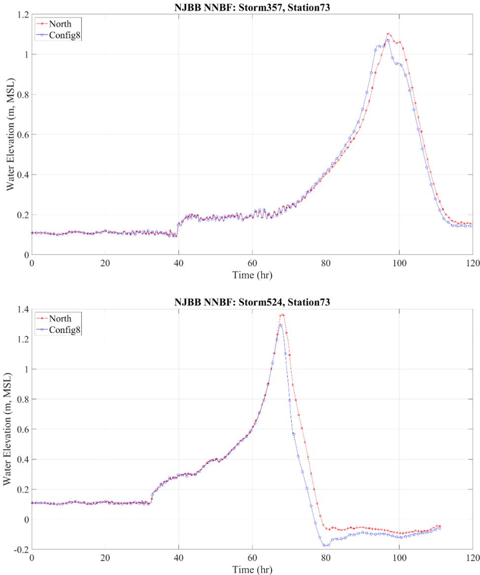
**Figure 20 Holgate NNBF effects on hydrographs at save point 73 for two high annual exceedance probability storms. The blue hydrograph represents the configuration with NNBF and structural measures and the red hydrograph represents the configuration with structural measures only**
