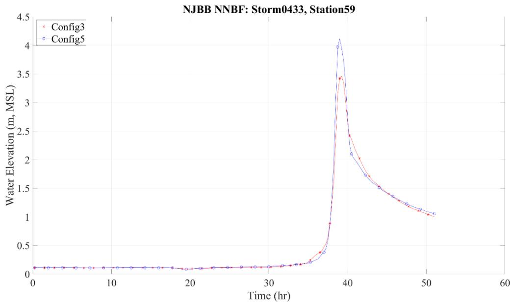
Figure 85 Storm 433 hydrograph for save point 59 "in front of" Brigantine area with and without NNBF
