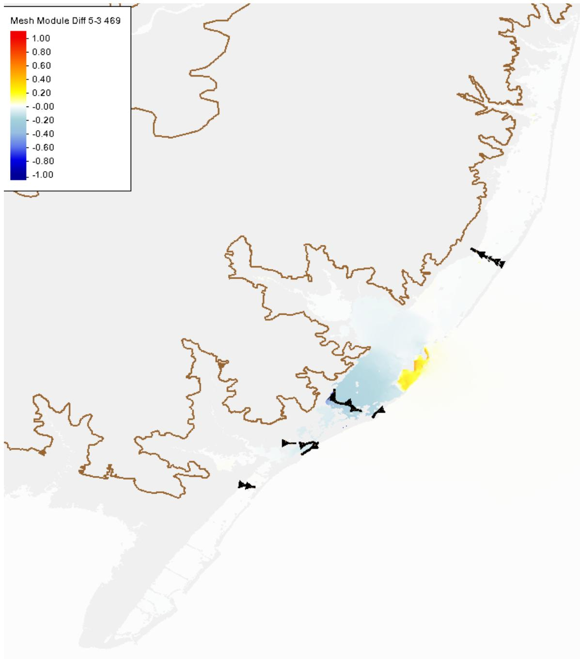
**Figure 46 Peak water level differences between Configuration 5 (Brigantine area NNBF) and Configuration 3 (structural only) for storm 469**
