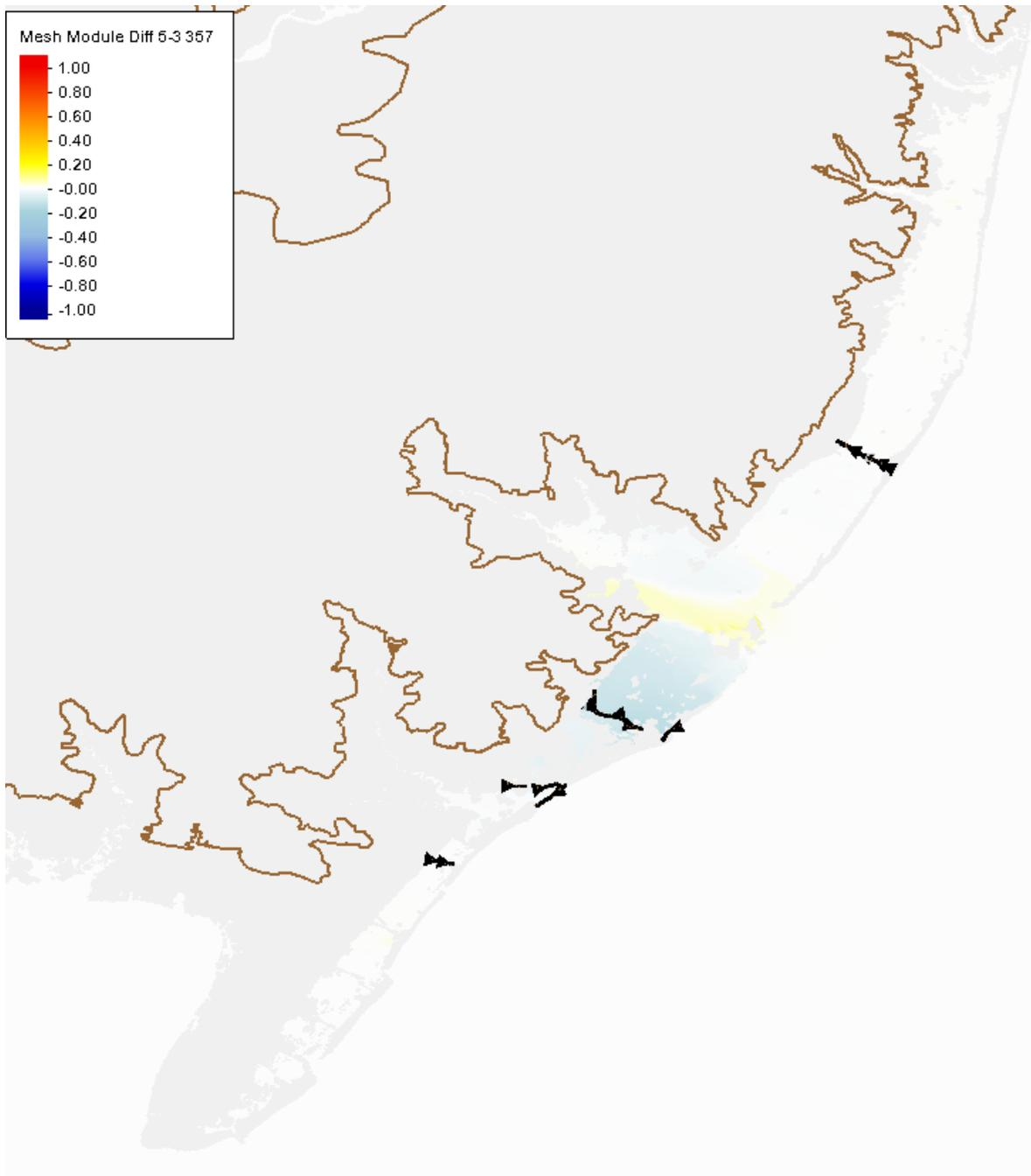
**Figure 43 Peak water level differences between Configuration 5 (Brigantine area NNBF) and Configuration 3 (structural only) for storm 357**
