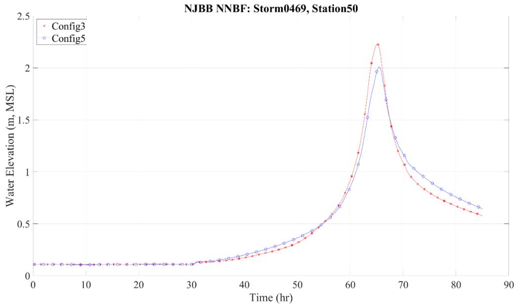
Figure 95 Storm 469 hydrograph for save point 50 "behind" Brigantine area with and without NNBF
