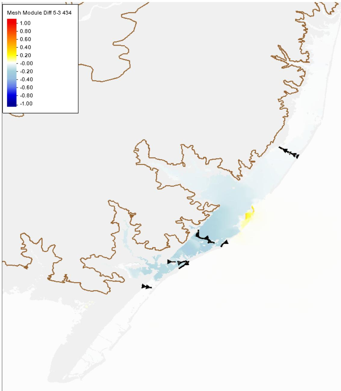
**Figure 45 Peak water level differences between Configuration 5 (Brigantine area NNBF) and Configuration 3 (structural only) for storm 434**
