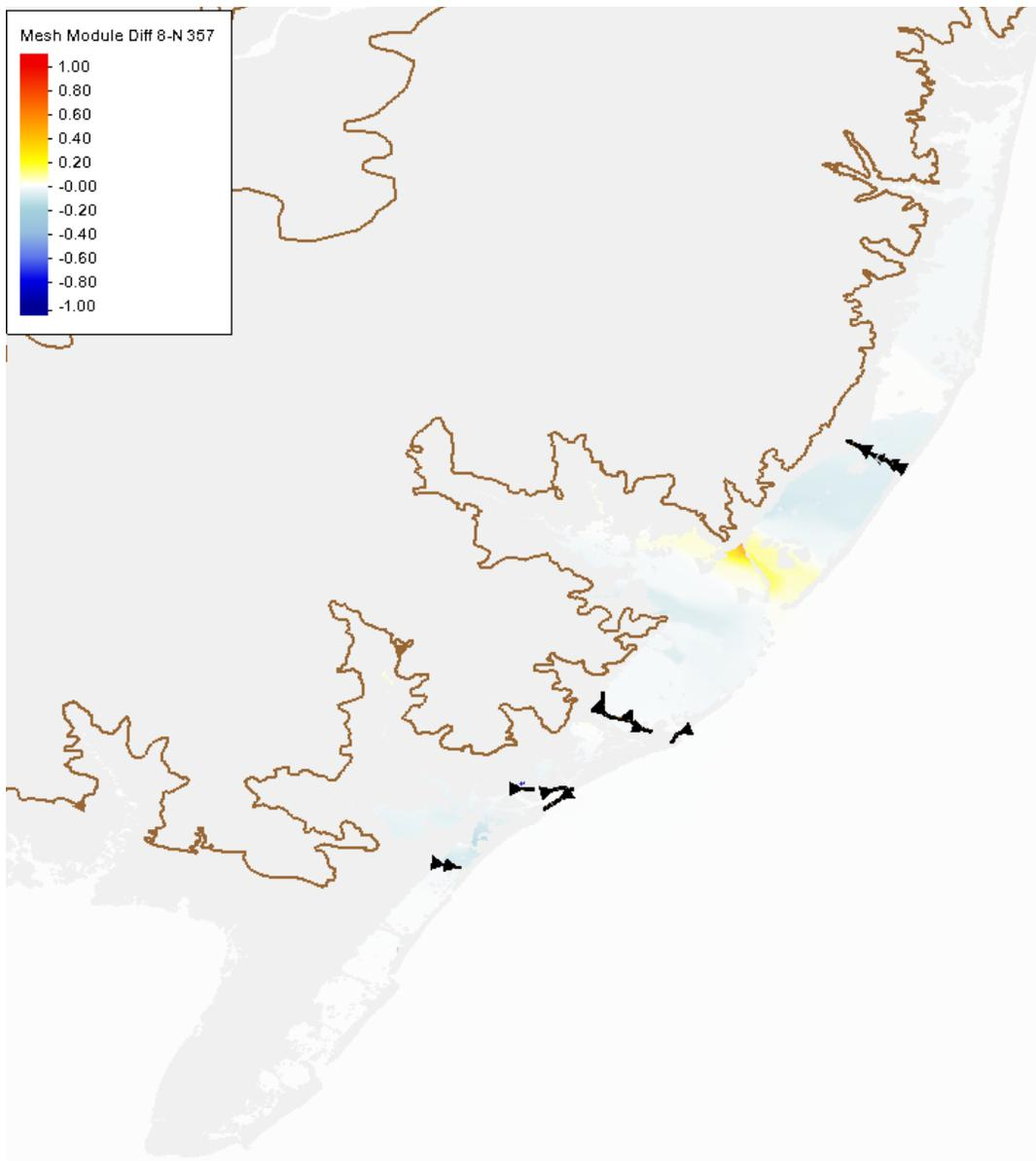
**Figure 53 Peak water level differences between Configuration 8 (Holgate and Great Egg Harbor area NNBF) and North Configuration (structural only) for storm 357**
