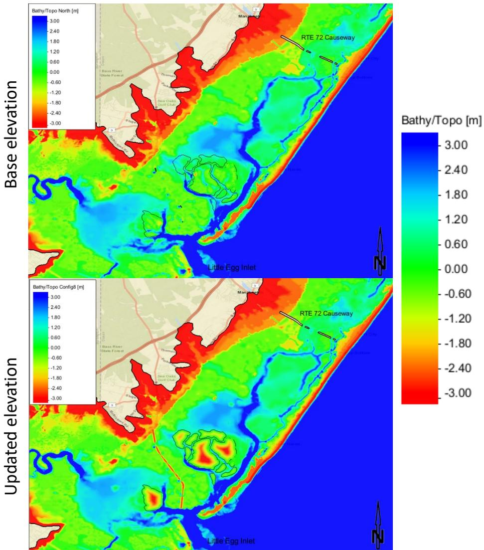
Figure 33 Updated ADCIRC elevation for Holgate area
