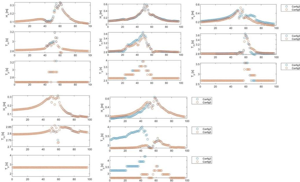
**Figure 149: Time series of significant wave height, peak period, and mean period for Storm 524. Top row, from left to right is station 49, 50, 59. Bottom row, from left to right is station 111, 117. Configuration 3 is shown in blue, Configuration 5 in orange.**
