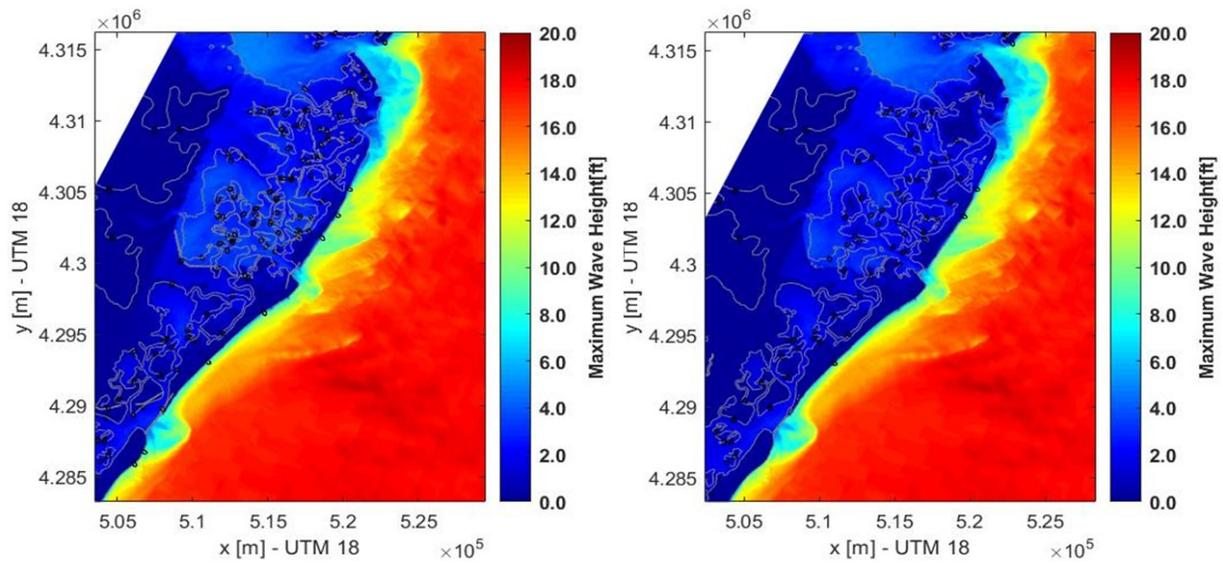
**Figure 26 Max Wave Height (ft) of Storm 636 for Configuration 3 (left) and Configuration 5 (right).**
