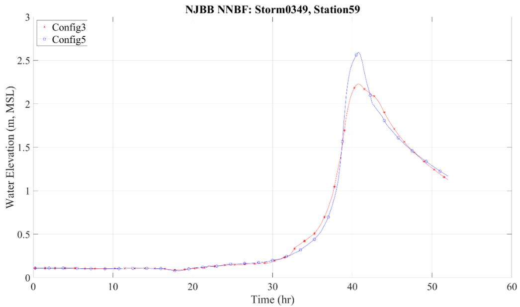
**Figure 83 Storm 349 hydrograph for save point 59 "in front of" Brigantine area with and without NNBF**
