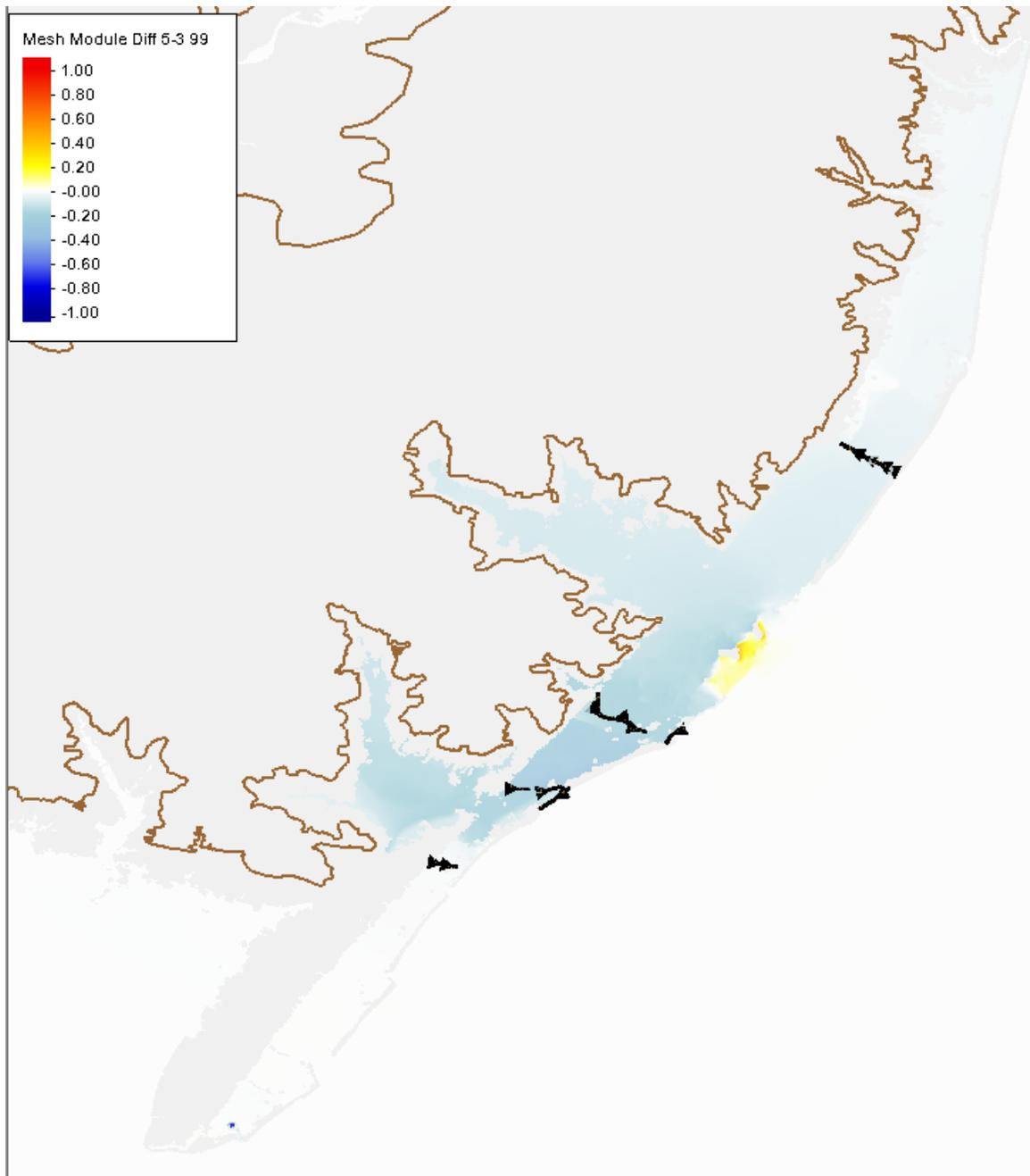
**Figure 40 Peak water level differences between Configuration 5 (Brigantine area NNBF) and Configuration 3 (structural only) for storm 99**
