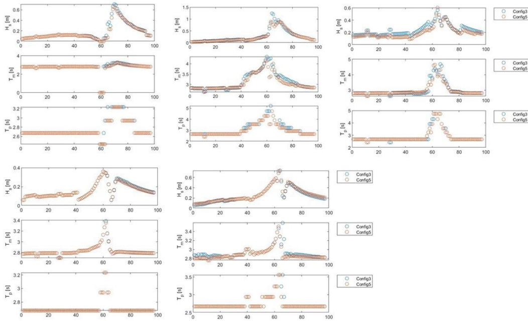
**Figure 29** Time series of significant wave height, peak period, and mean period for Storm 350. Top row, from left to right is station 49, 50, 59. Bottom row, from left to right is station 111, 117. Configuration 3 is shown in blue, Configuration 5 in orange.
