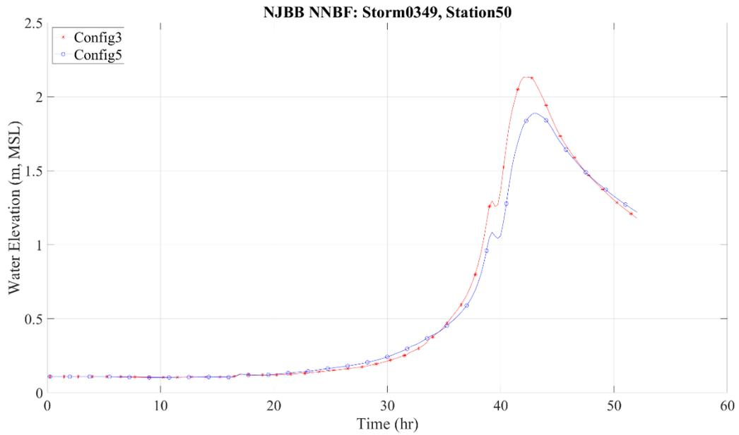
Figure 91 Storm 349 hydrograph for save point 50 "behind" Brigantine area with and without NNBF
