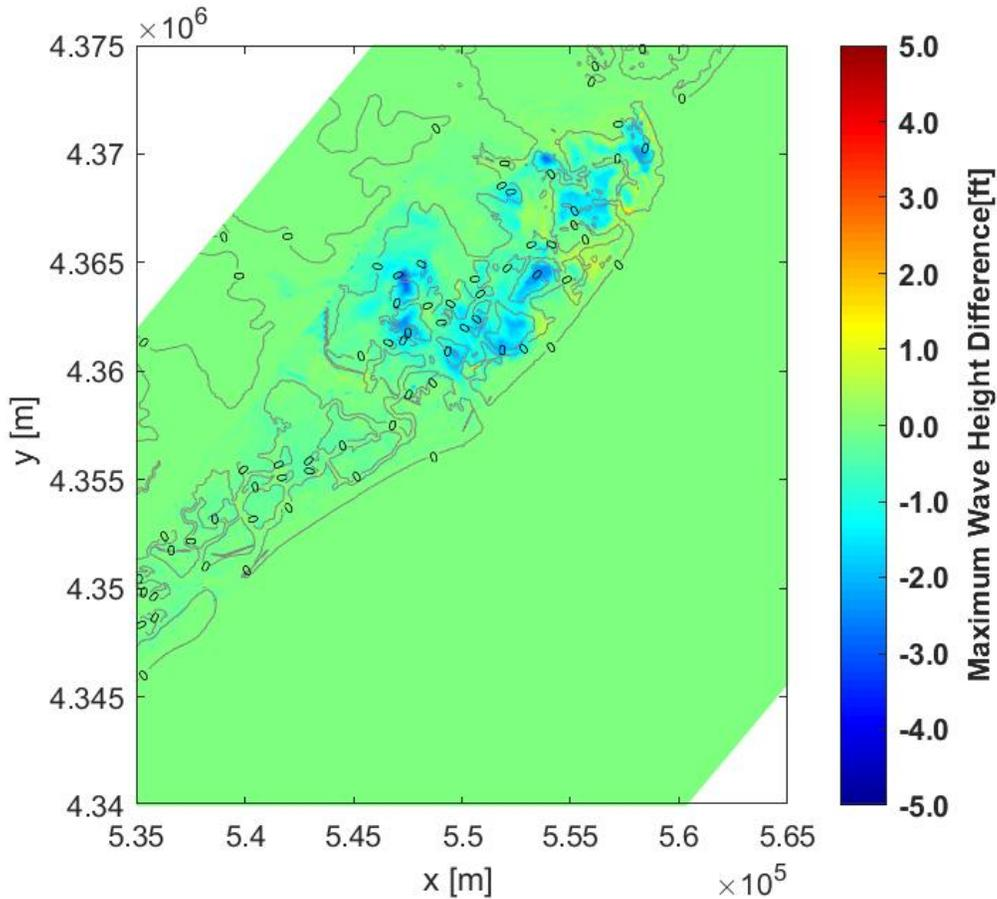
**Figure 28 Maximum wave height difference for storm 636 between Configuration 3 and Configuration 5. Cool tones indicate reductions in wave height due to NNBFs and warmer tones indicate wave height increases due to NNBFs.**
