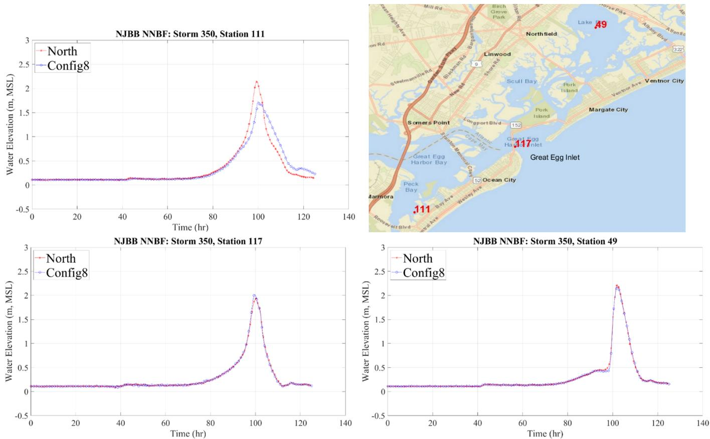
**Figure 24 Great Egg Harbor save points and examples of storm hydrograph effects for storm 350. The blue hydrograph represents the configuration with NNBF and structural measures and the red hydrograph represents the configuration with structural measures only**
