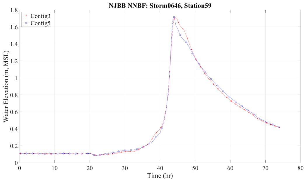
**Figure 89 Storm 646 hydrograph for save point 59 "in front of" Brigantine area with and without NNBF**
