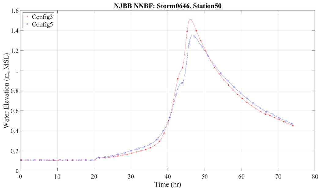
Figure 97 Storm 646 hydrograph for save point 50 "behind" Brigantine area with and without NNBF
