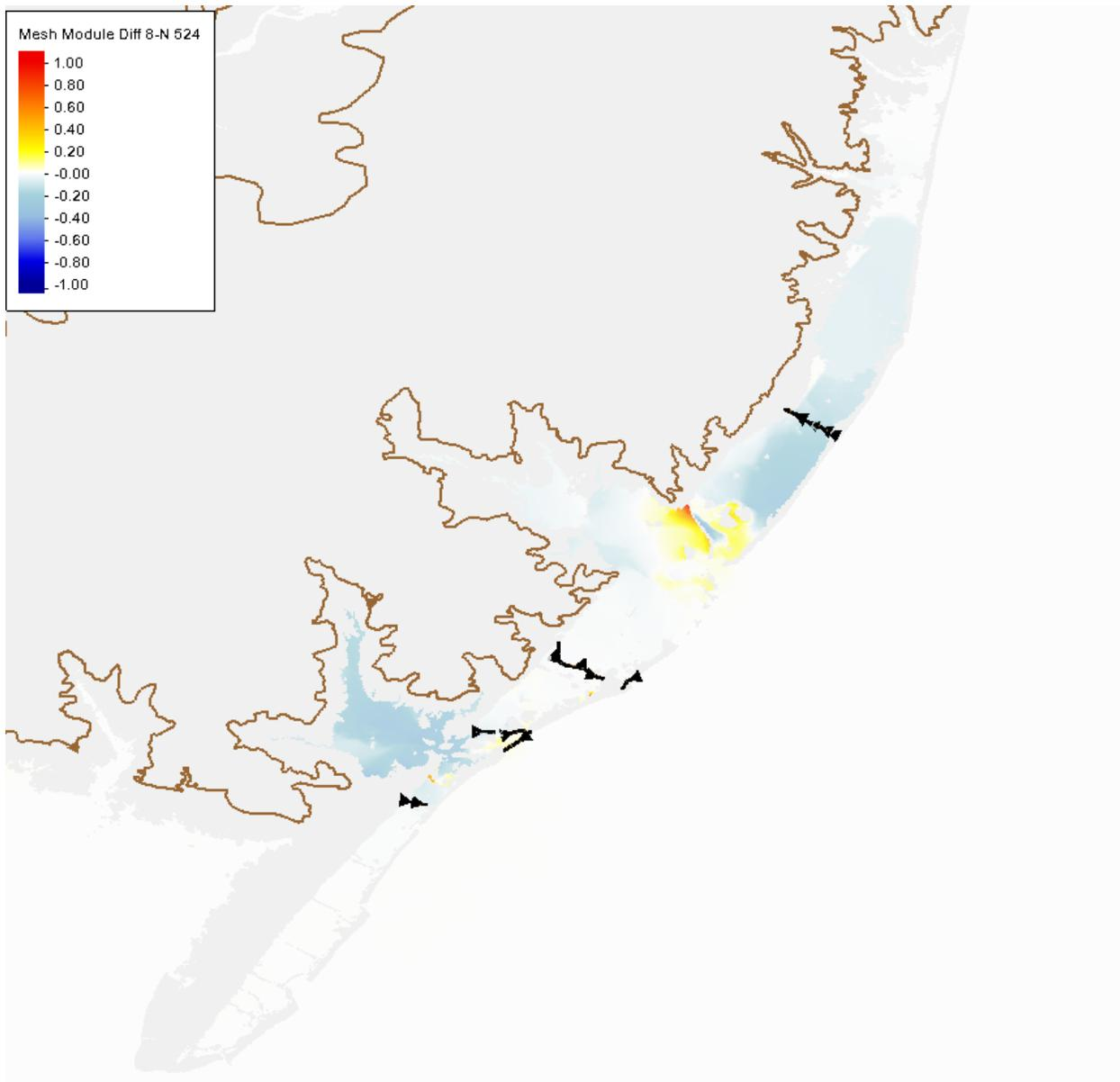
**Figure 57 Peak water level differences between Configuration 8 (Holgate and Great Egg Harbor area NNBF) and North Configuration (structural only) for storm 524**
