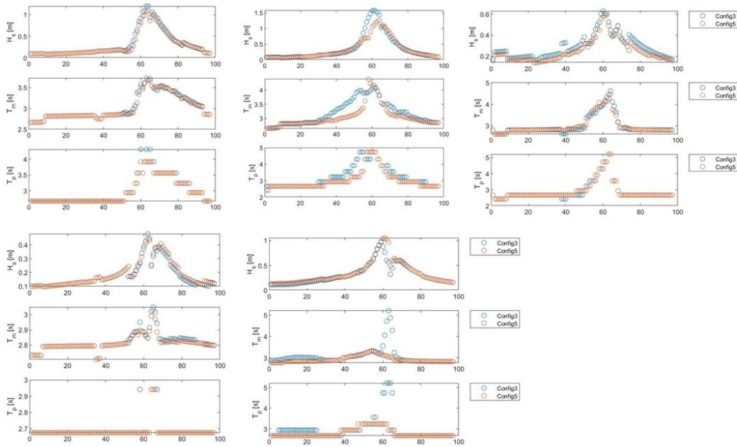
**Figure 142: Time series of significant wave height, peak period, and mean period for Storm 99. Top row, from left to right is station 49, 50, 59. Bottom row, from left to right is station 111, 117. Configuration 3 is shown in blue, Configuration 5 in orange.**
