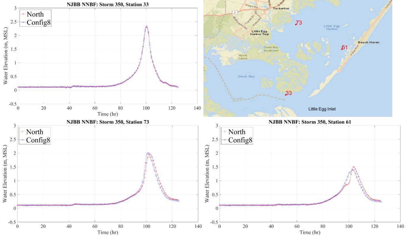
**Figure 19 Holgate save points and examples of storm hydrograph effects for storm 350. The blue hydrograph represents the configuration with NNBF and structural measures and the red hydrograph represents the configuration with structural measures only**
