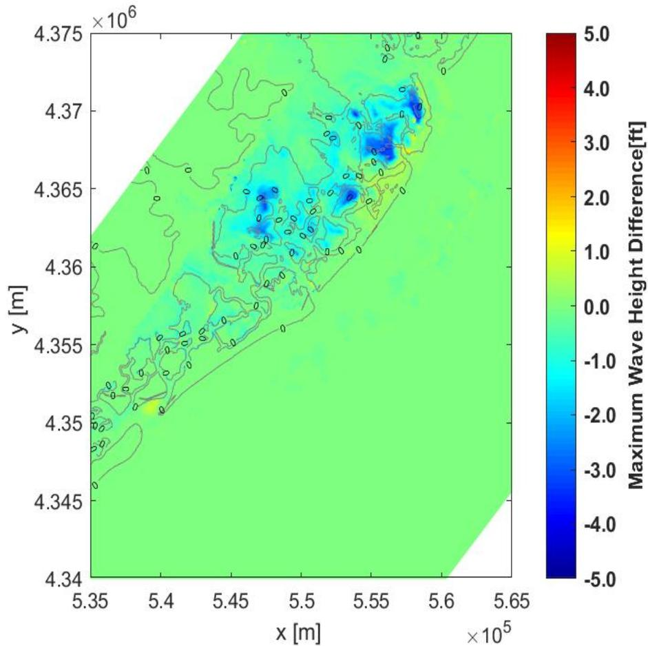
**Figure 27 Maximum wave height difference for storm 350 between Configuration 3 and Configuration 5. Cool tones indicate reductions in wave height due to NNBFs and warmer tones indicate wave height increases due to NNBFs.**
