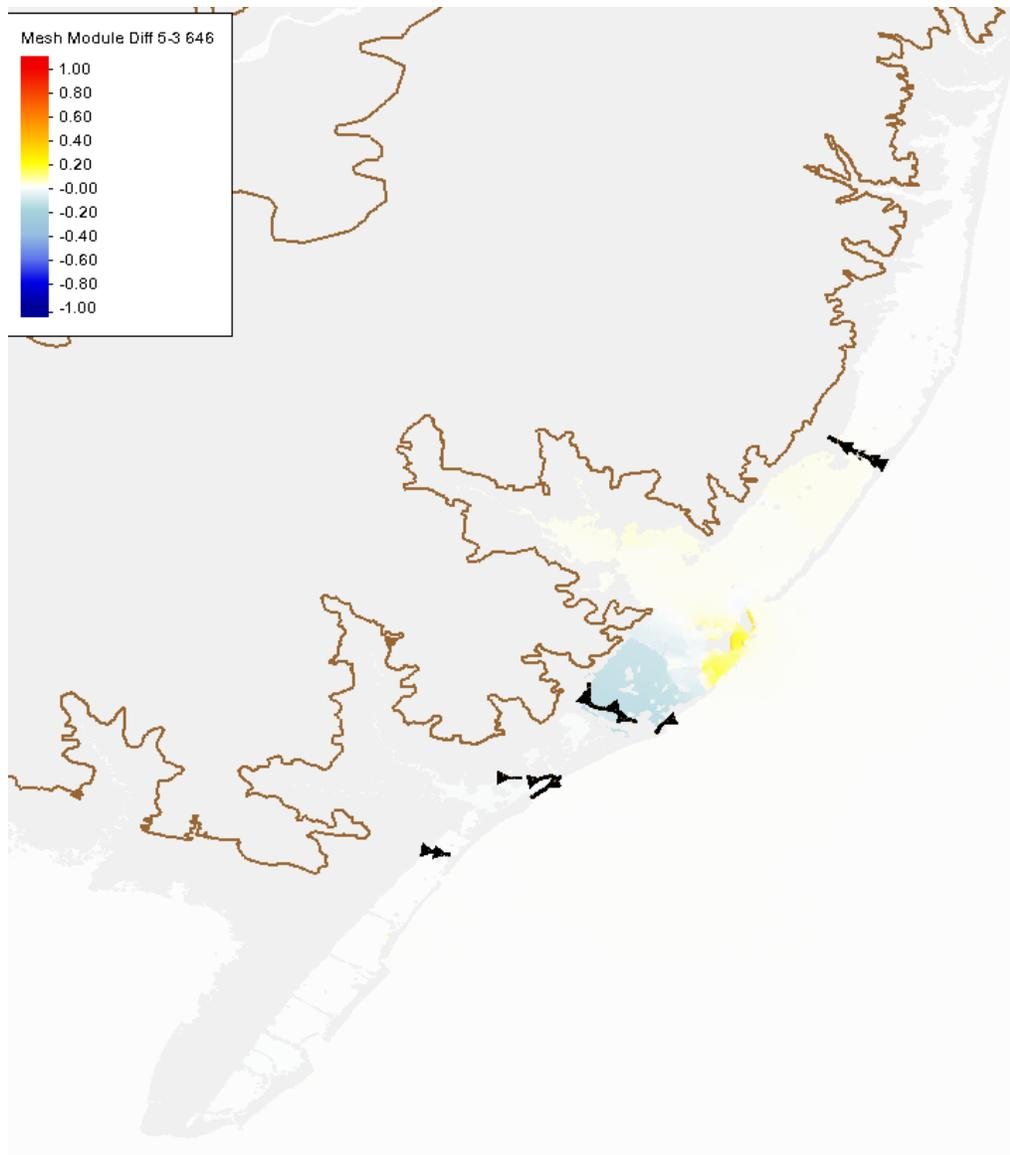
**Figure 49 Peak water level differences between Configuration 5 (Brigantine area NNBF) and Configuration 3 (structural only) for storm 646**
