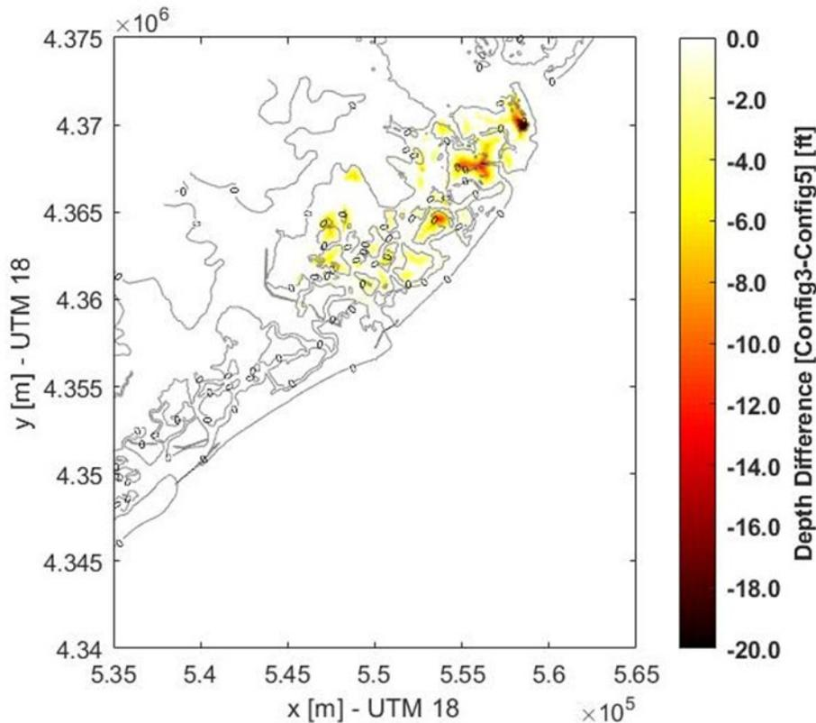
**Figure 12 Implemented NNBF features and storm surge barrier included in the STWAVE child domains for Configuration 5. The NNBF are depicted as a difference between the bathymetry of Configuration 3 (no NNBF) and Configuration 5 (with NNBF.)**
