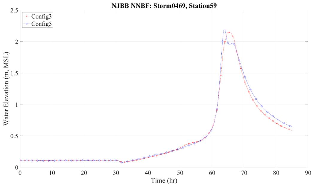
Figure 87 Storm 469 hydrograph for save point 59 "in front of" Brigantine area with and without NNBF
