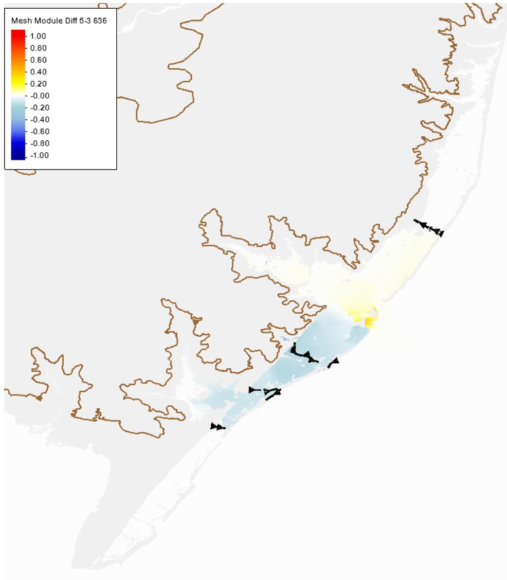
**Figure 48 Peak water level differences between Configuration 5 (Brigantine area NNBF) and Configuration 3 (structural only) for storm 636**
