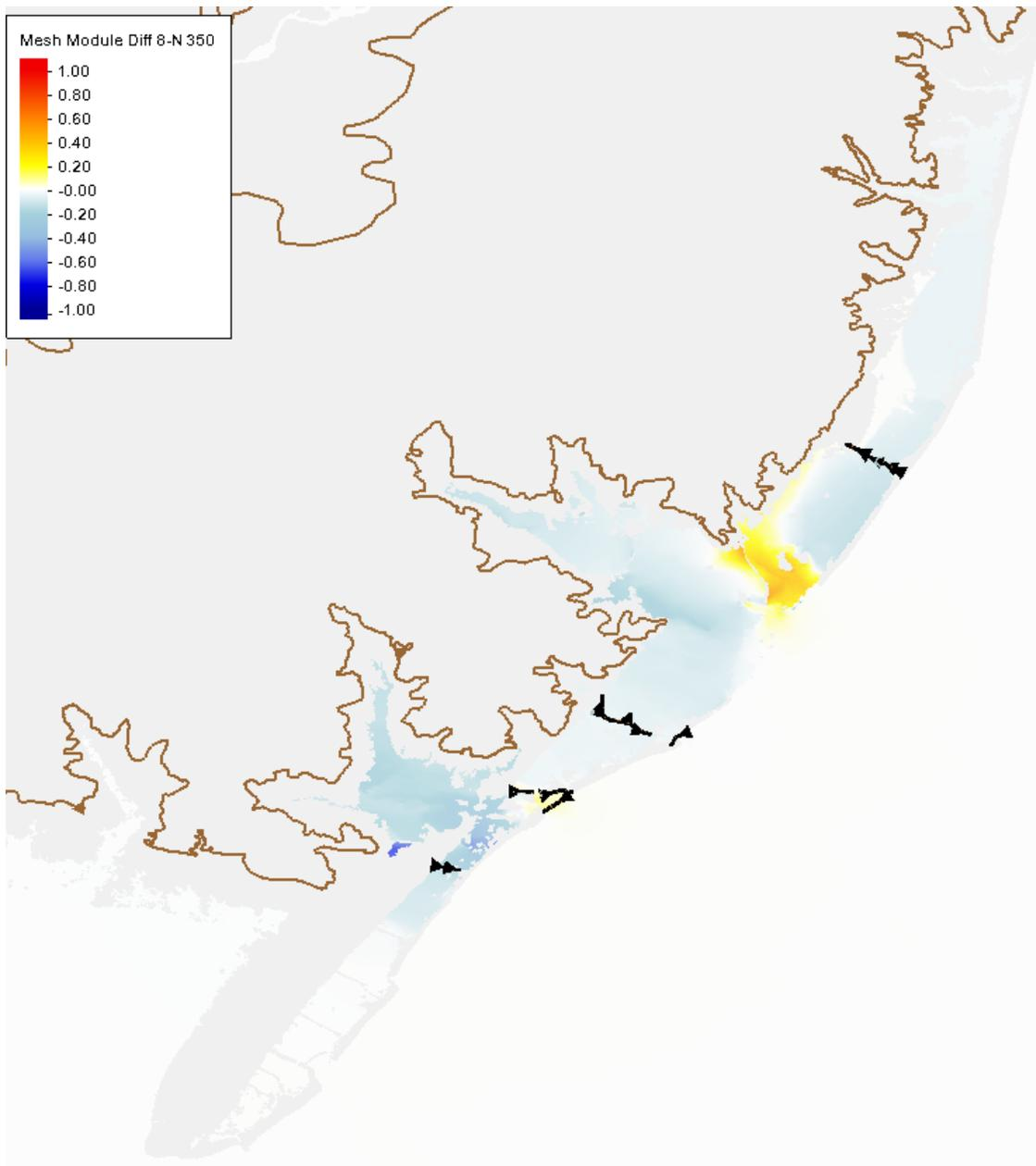
**Figure 52 Peak water level differences between Configuration 8 (Holgate and Great Egg Harbor area NNBF) and North Configuration (structural only) for storm 350**
