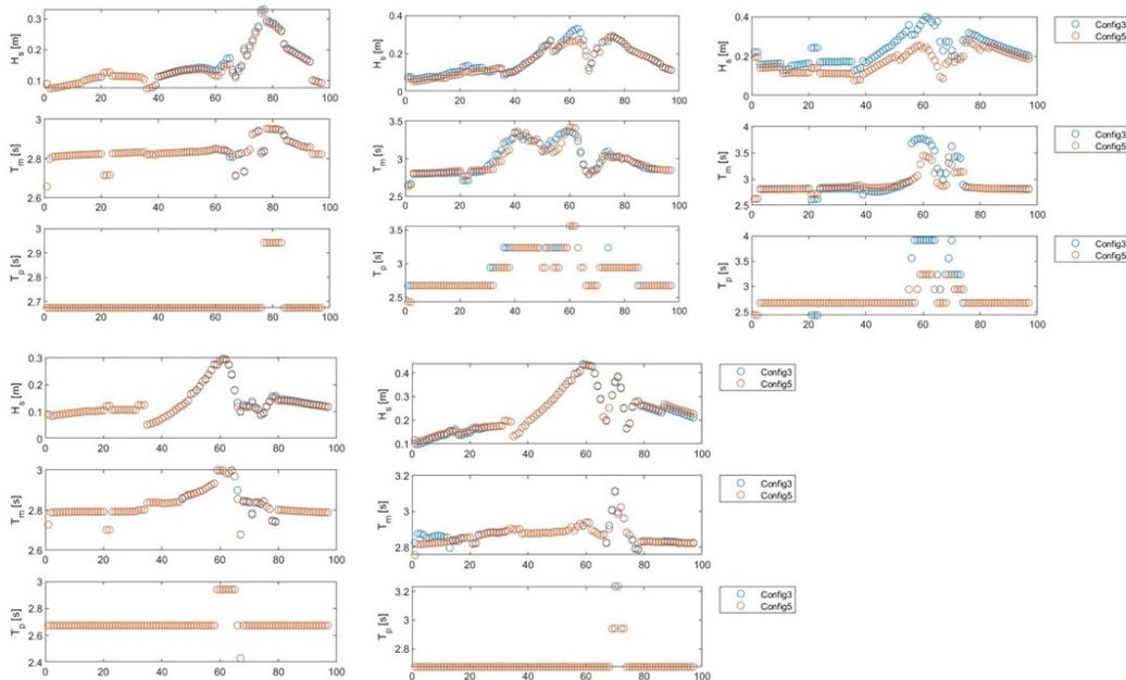
**Figure 145: Time series of significant wave height, peak period, and mean period for Storm 357. Top row, from left to right is station 49, 50, 59. Bottom row, from left to right is station 111, 117. Configuration 3 is shown in blue, Configuration 5 in orange.**
