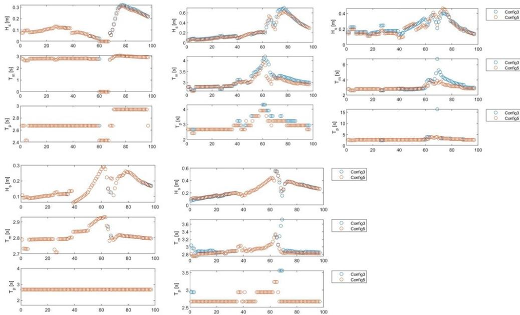
**Figure 143:** Time series of significant wave height, peak period, and mean period for Storm 349. Top row, from left to right is station 49, 50, 59. Bottom row, from left to right is station 111, 117. Configuration 3 is shown in blue, Configuration 5 in orange.
