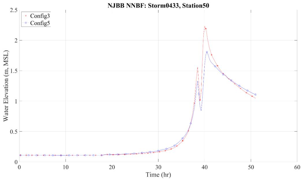
Figure 93 Storm 433 hydrograph for save point 50 "behind" Brigantine area with and without NNBF
