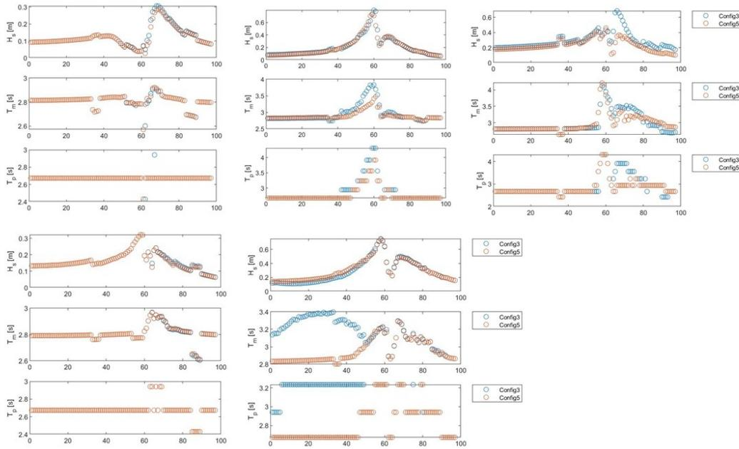
**Figure 148: Time series of significant wave height, peak period, and mean period for Storm 469. Top row, from left to right is station 49, 50, 59. Bottom row, from left to right is station 111, 117. Configuration 3 is shown in blue, Configuration 5 in orange.**
