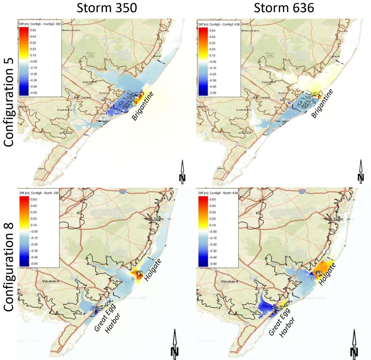
**Figure 17 Difference in maximum water level elevation for storms 350 and 636 under modeling configuration 5 (Brigantine NNBF) and configuration 8 (Holgate and Great Egg Harbor NNBF) compared to the non-NNBF (structural protection only) configurations**
