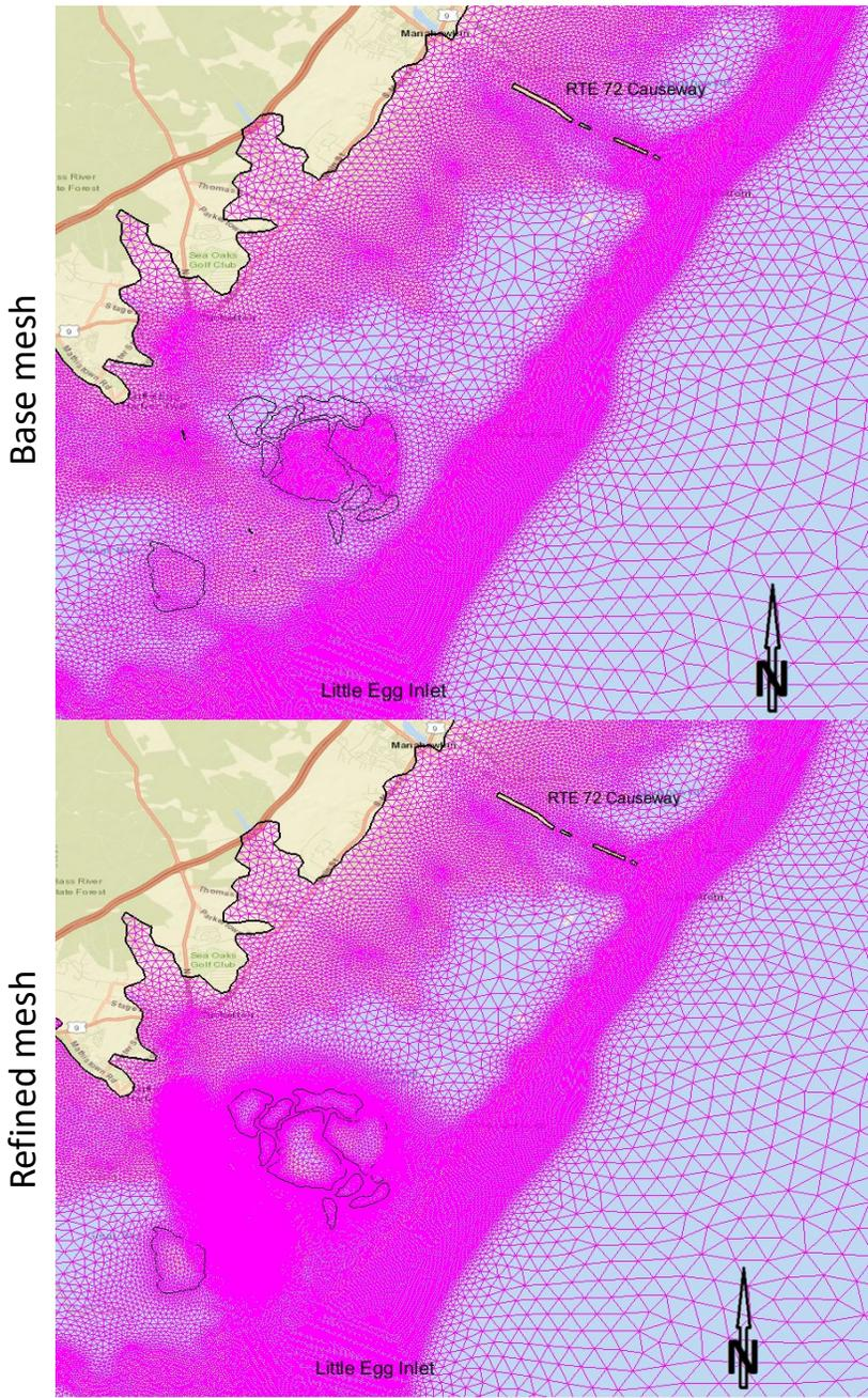
Figure 31 Change in mesh resolution in the Holgate area to accommodate the NNB
