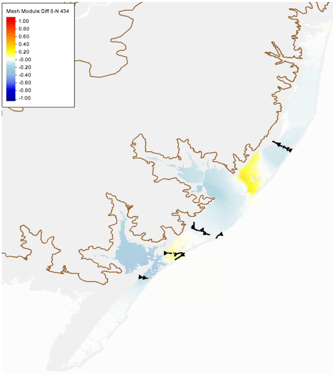
**Figure 55 Peak water level differences between Configuration 8 (Holgate and Great Egg Harbor area NNBf) and North Configuration (structural only) for storm 434**
