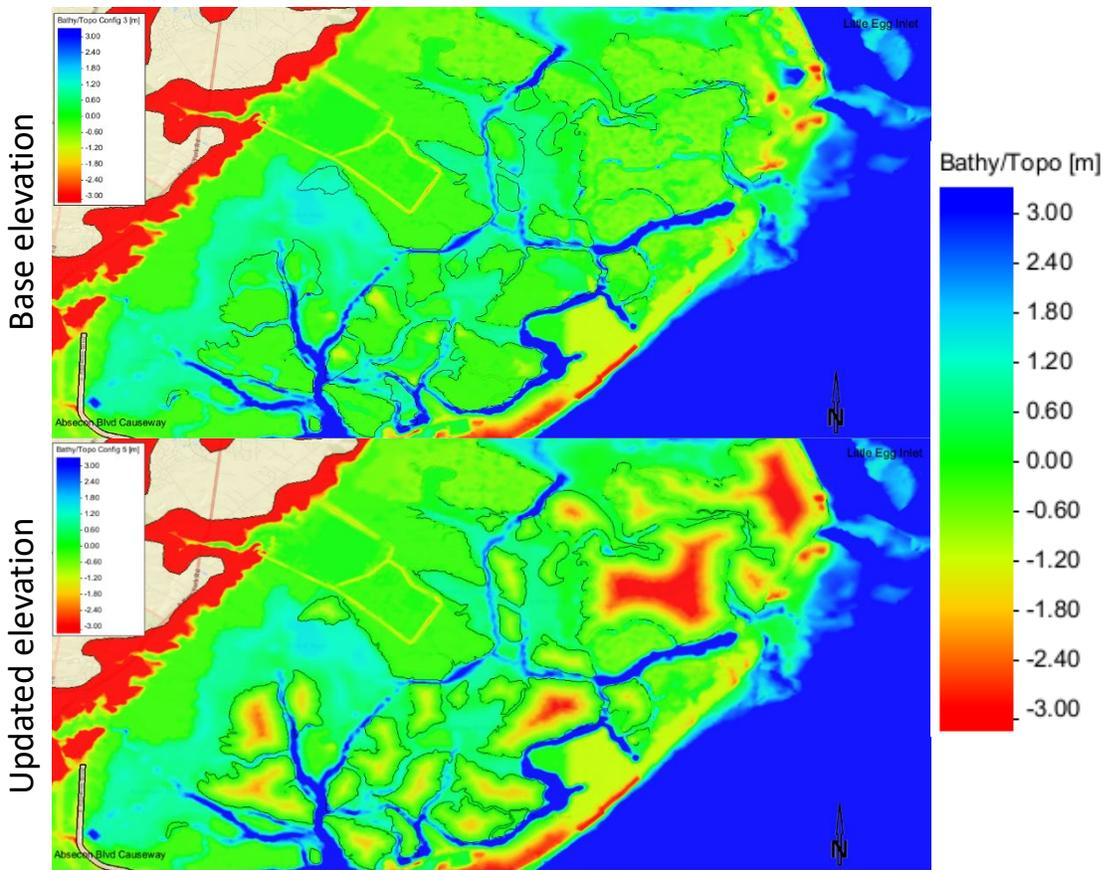
Figure 34 Updated ADCIRC elevation for Brigantine area
