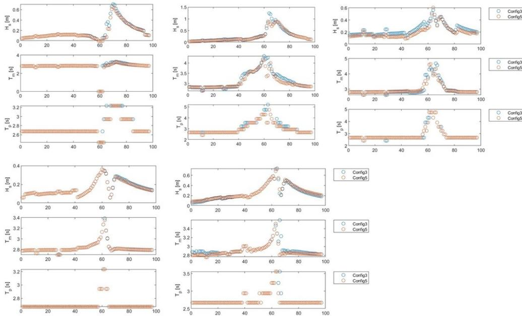
**Figure 144:** Time series of significant wave height, peak period, and mean period for Storm 350. Top row, from left to right is station 49, 50, 59. Bottom row, from left to right is station 111, 117. Configuration 3 is shown in blue, Configuration 5 in orange.
