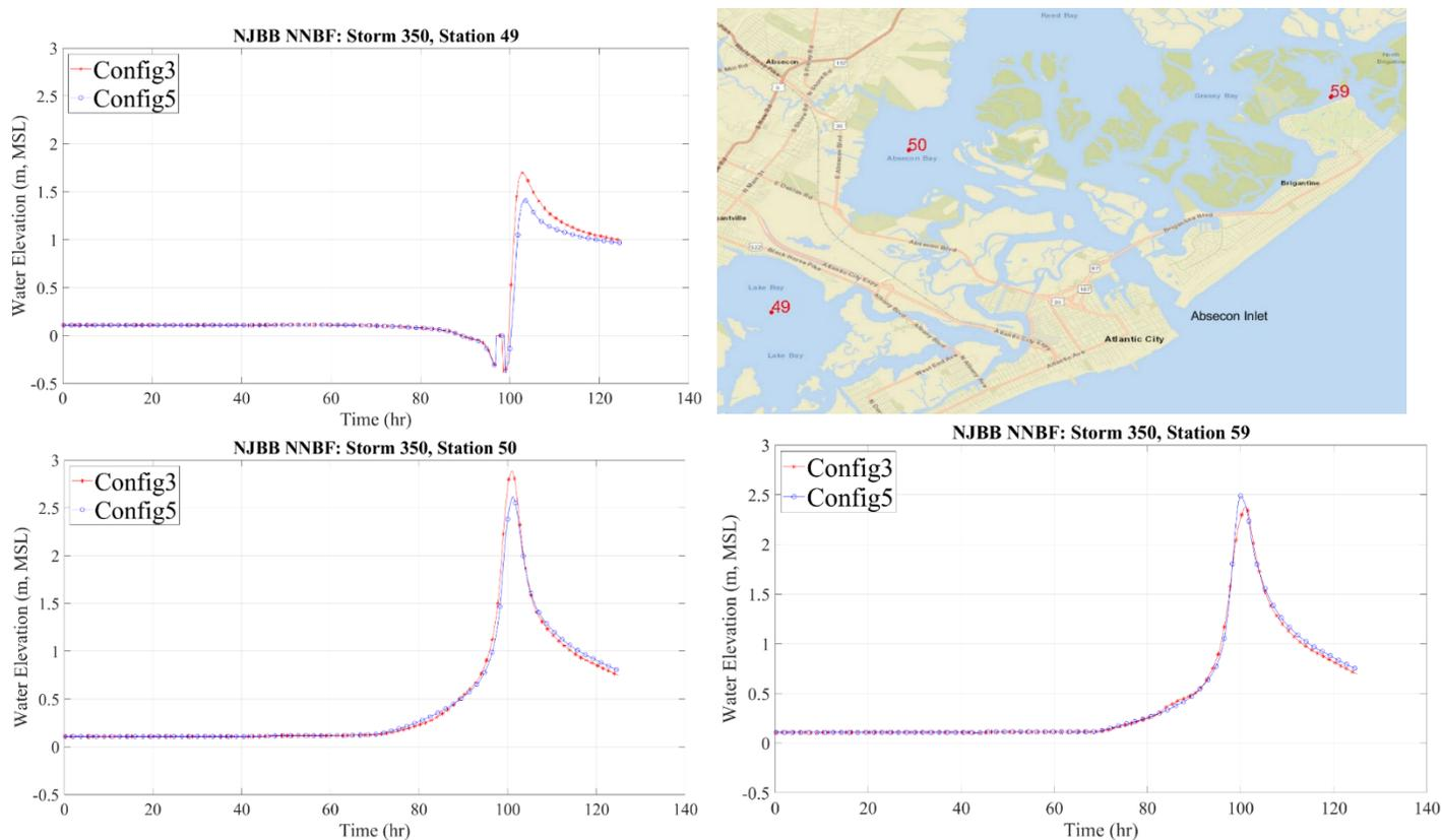
**Figure 22 Brigantine save points and examples of storm hydrograph effects for storm 350. The blue hydrograph represents the configuration with NNBF and structural measures and the red hydrograph represents the configuration with structural measures only**
