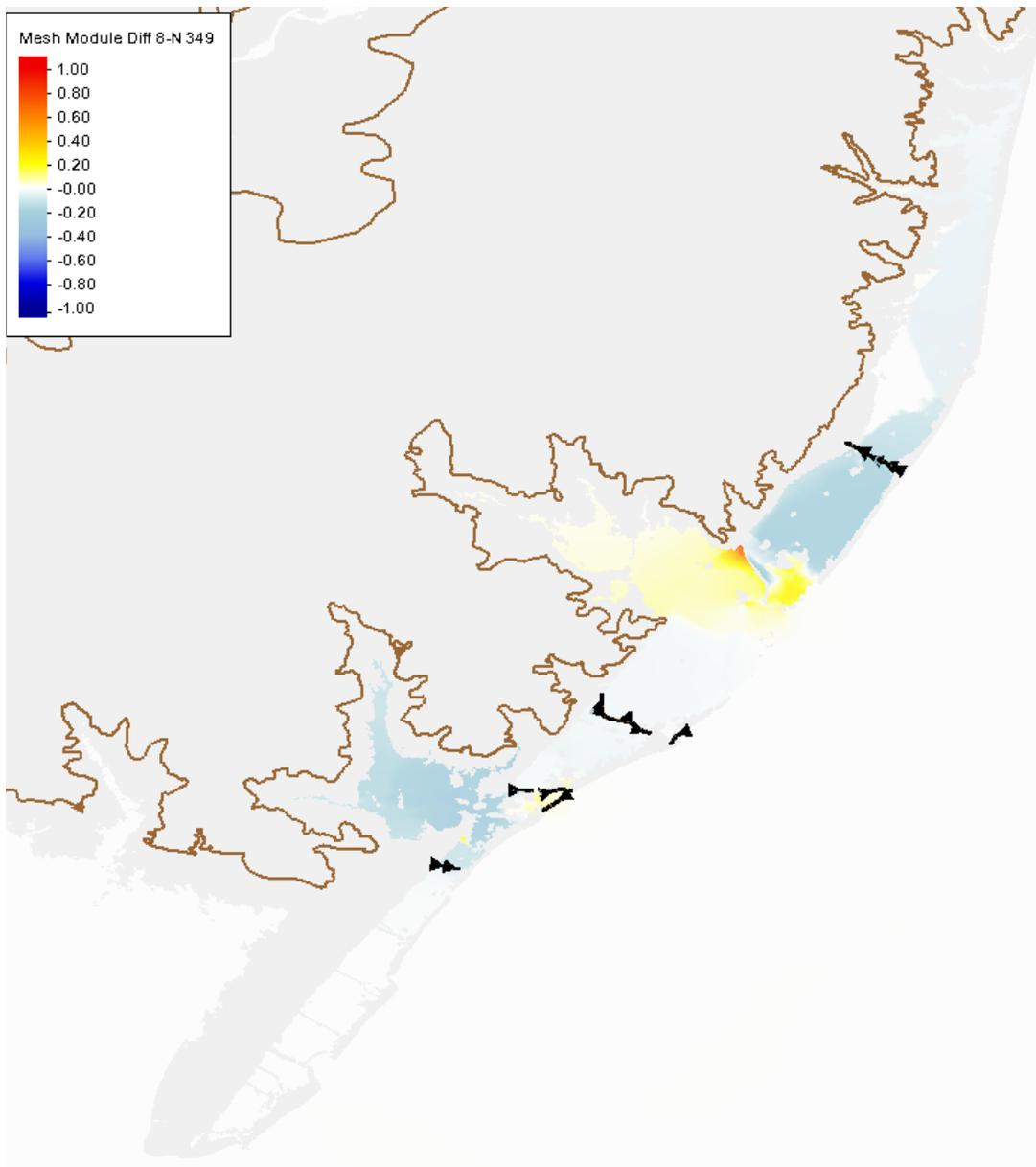
**Figure 51 Peak water level differences between Configuration 8 (Holgate and Great Egg Harbor area NNBF) and North Configuration (structural only) for storm 349**
