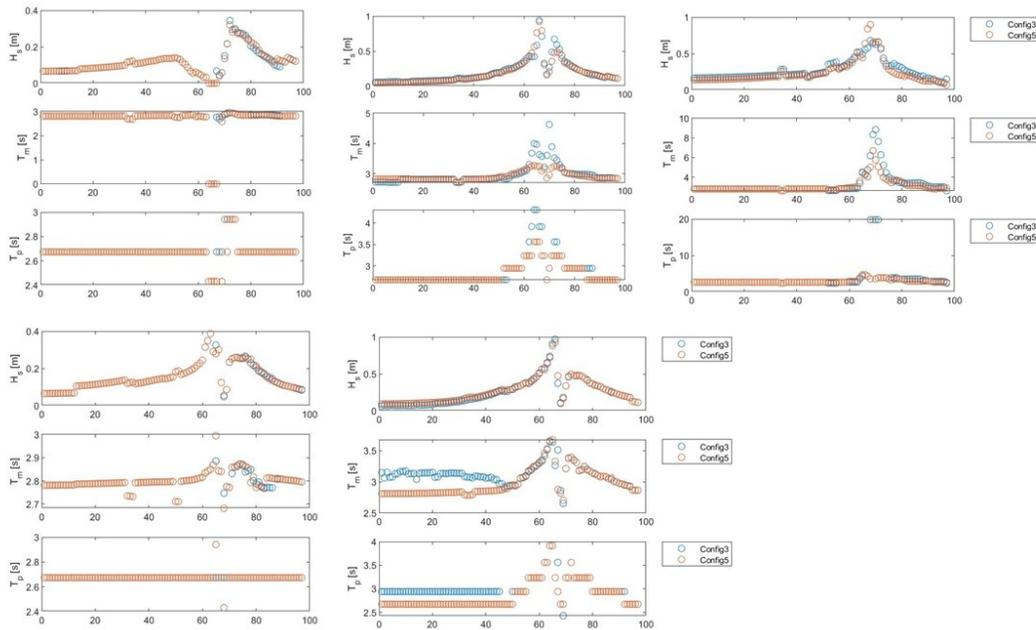
**Figure 146: Time series of significant wave height, peak period, and mean period for Storm 433. Top row, from left to right is station 49, 50, 59. Bottom row, from left to right is station 111, 117. Configuration 3 is shown in blue, Configuration 5 in orange.**
