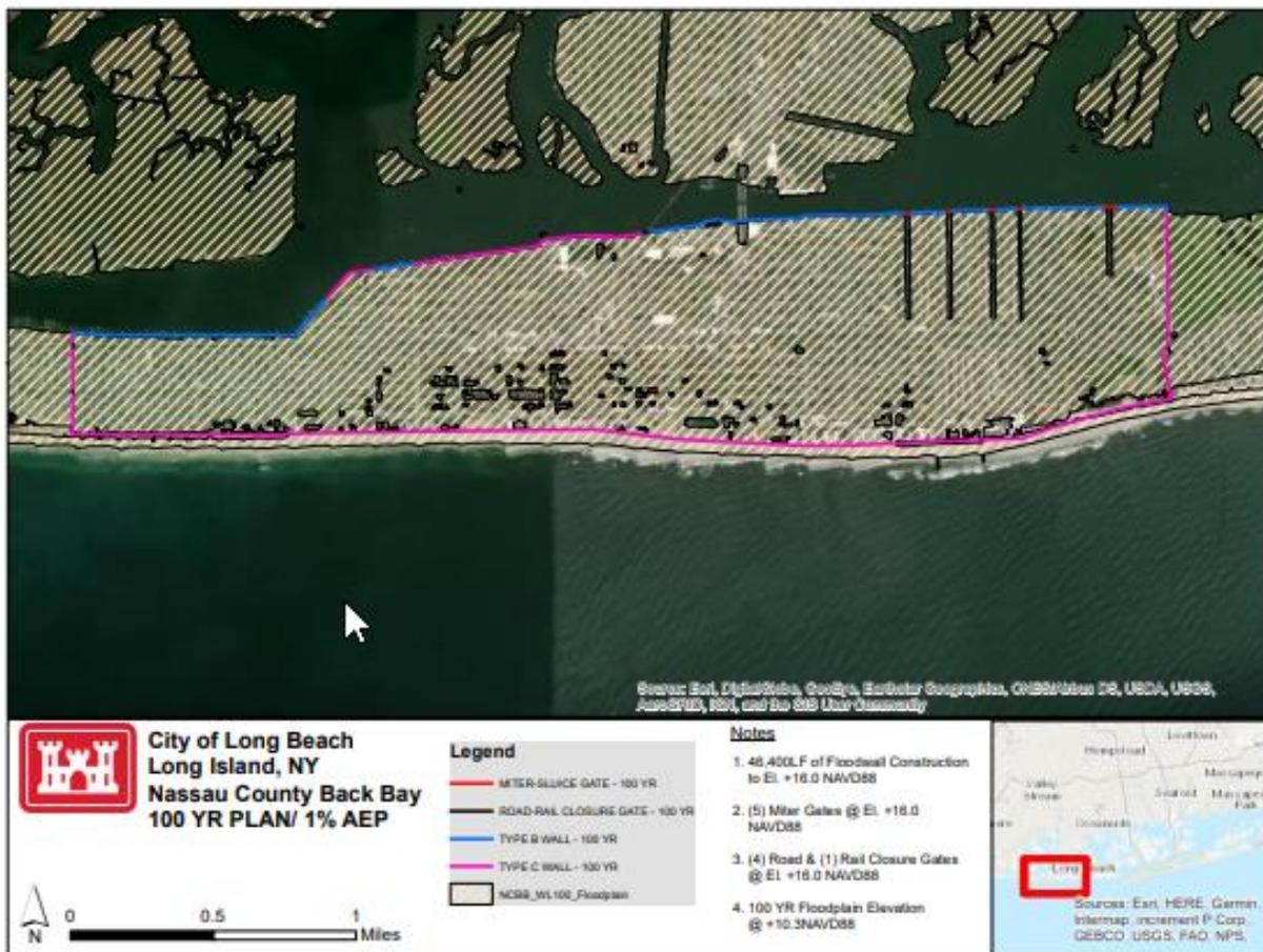
Figure 38 - Comprehensive Floodwall for the City of Long Beach (1% AEP Alignment)
