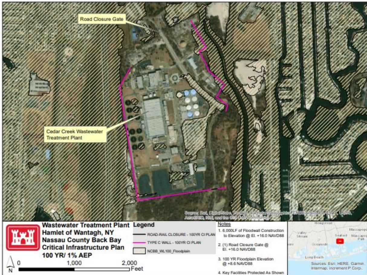
Figure 49 - Localized Floodwall for Cedar Creek Wastewater Treatment Plant
