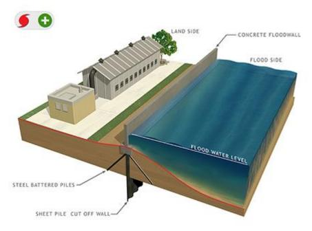
Figure 2.3.2.7 – Example of a Type B/C Floodwall (NACCS)
