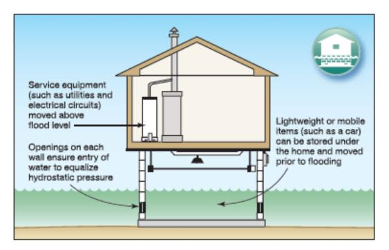
Figure 5.1.1 – Home Elevation Concept Diagram (Courtesy of Google Images)
