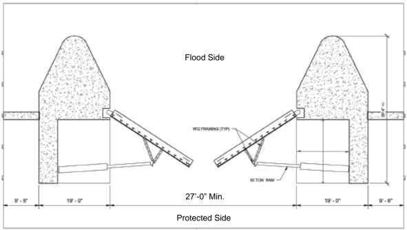
Figure 2.3.3.8 NCBB Miter Gate Design (Courtesy of USACE-NAP)
