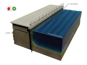
Figure 2.3.2.9 – Example of a Type D Floodwall (NACCS)
