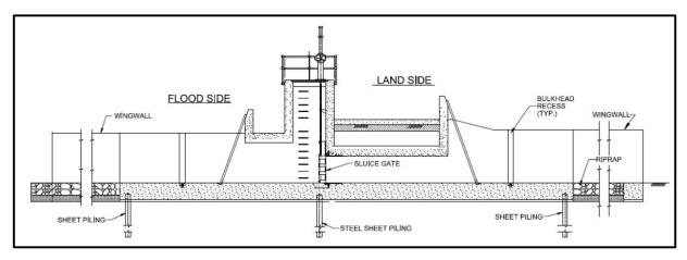
Figure 2.3.3.12 – Sluice Gate Typical Section (Courtesy of USACE-NAO)
