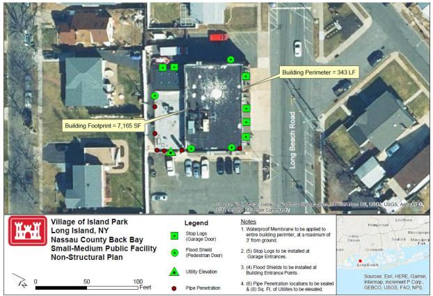
Figure 5.3.1 – Island Park FD Dry-Floodproofing Concept Plan (Courtesy of USACE-NAP)
