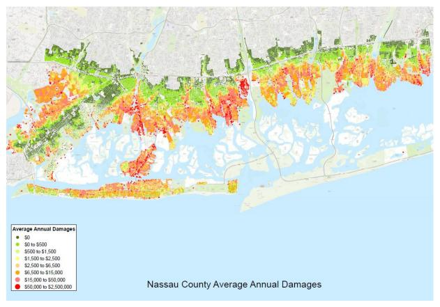
Figure 2.2.1 – NCBB Average Annual Damages (Courtesy of USACE-NAP)
