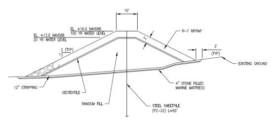
Figure 2.3.2.2 – Typical Section - Levee - Type A
