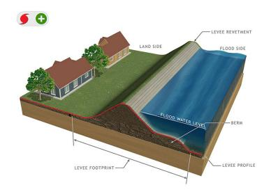
Figure 2.3.2.6 – Example of a Type A Levee (NACCS)
