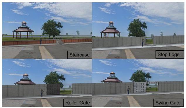
Figure 2.3.4.6 – Additional Access Measures (Courtesy of USACE-NAP)
