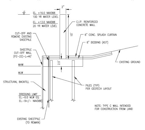
Figure 2.3.2.4 – Typical Section – Concrete Cantilever Wall on Piles – Type C
