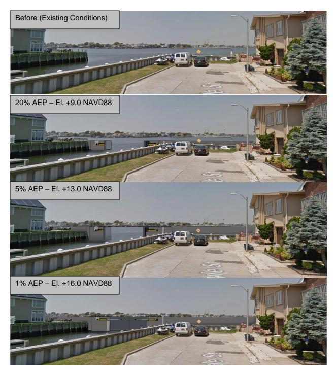
Figure 2.3.5.6 – Street View of Floodwall Alignment (Courtesy of USACE-NAP)
