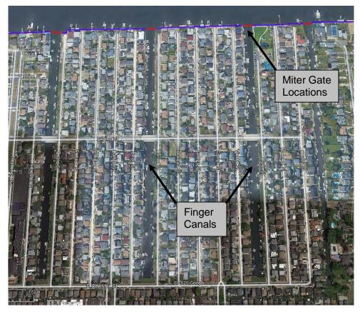
Figure 2.3.5.4 – Miter Gate Placement Example (Courtesy of Google Earth)
