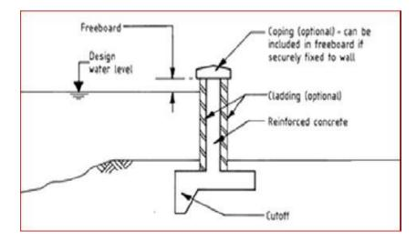
Figure 2.3.2.1 – NACCS Floodwall Cross Section (Concrete T-Wall)
