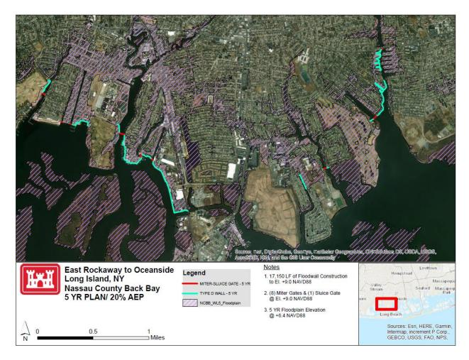
Figure 2.3.2.10: East Rockaway to Oceanside 20% AEP Plan – C2 (Courtesy of USACE-NAP)
