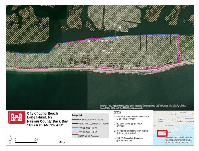
Figure 2.3.5.8 – City of Long Beach 1% AEP Plan (Courtesy of USACE-NAP)
