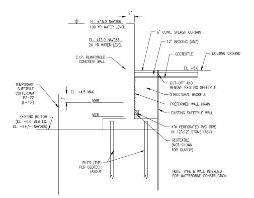
Figure 2.1.2.3 – Typical Section - Concrete Cantilever Wall on Piles - Type B
