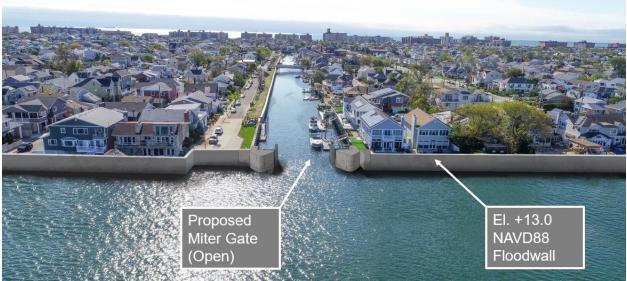
Figure 2.3.3.10 – NCBB Miter Gate – 5% AEP Plan (Courtesy of USACE-NAP)
