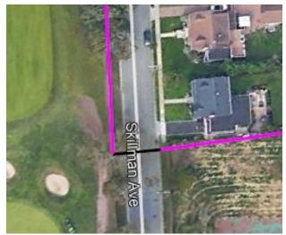
Figure 2.3.3.3: Road Closure Gate Alignment Example (Courtesy of Google Earth)
