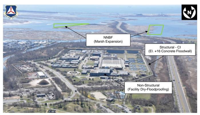
Figure 8.1.2 – Wantagh Treatment Plant Conceptual Critical Infrastructure Plan (Courtesy of Civil Air Patrol/USACE-NAP)
