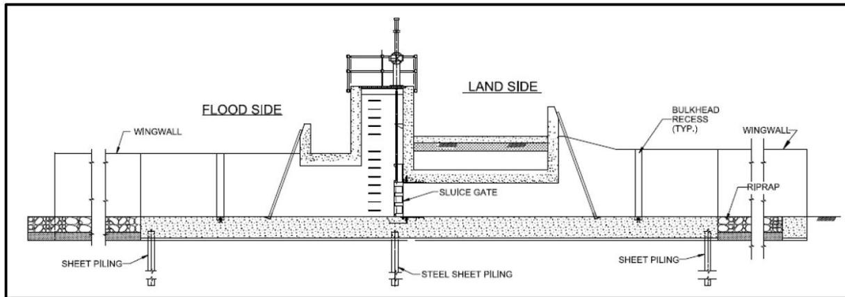
Figure 2.3.3.12 – Sluice Gate Typical Section (Courtesy of USACE-NAO)
