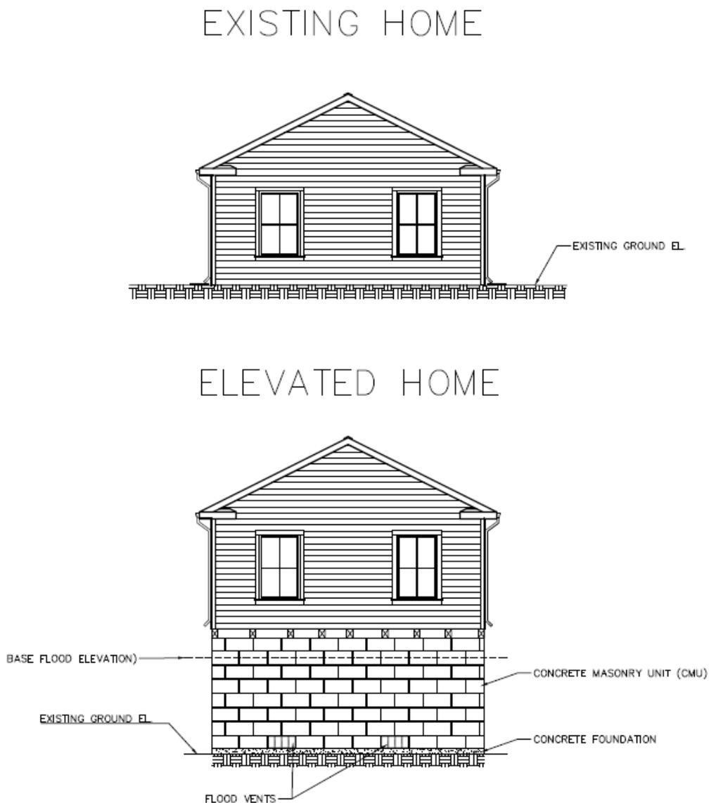
Figure 5.2.1 – Extended Foundation Concept Drawing (Courtesy of USACE-NAP)
