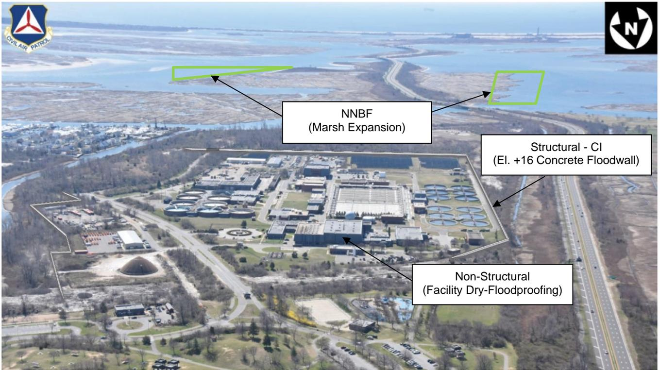
Figure 8.1.2 – Wantagh Treatment Plant Conceptual Critical Infrastructure Plan
