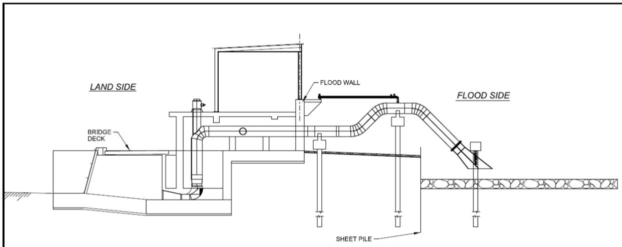
Figure 2.3.5.9 – Pump Station Typical Section (Courtesy of USACE-NAO)
