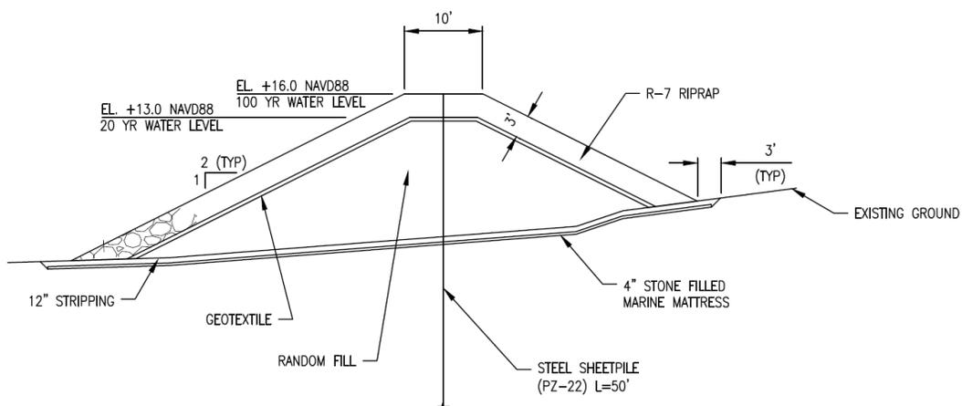
Figure 2.3.2.2 – Typical Section - Levee - Type A
