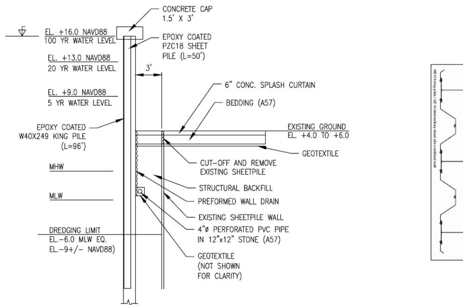
Figure 2.3.2.5 – Typical Section – King Pile/Sheet Pile Combi-Wall - Type D
