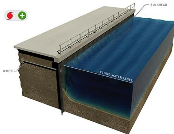
Figure 2.3.2.9 – Example of a Type D Floodwall (NACCS)
