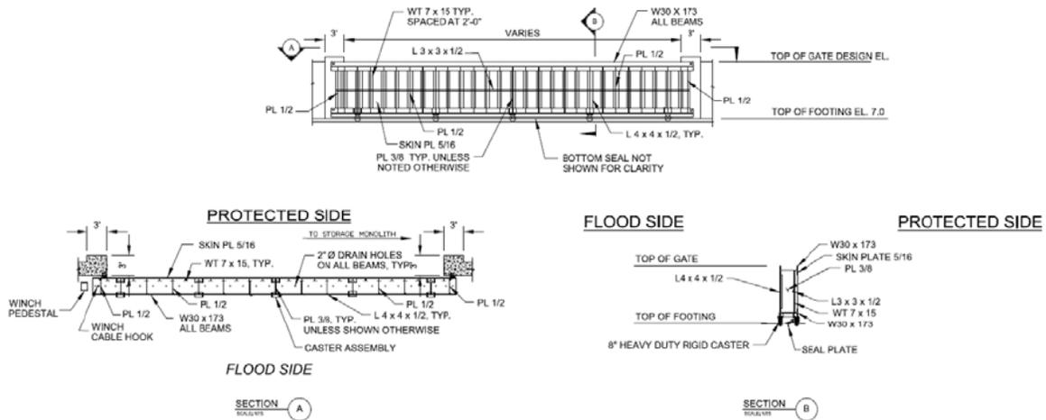
Figure 2.3.3.2 – Roller Gate Typical Section (Moffat & Nichol, 2018)
