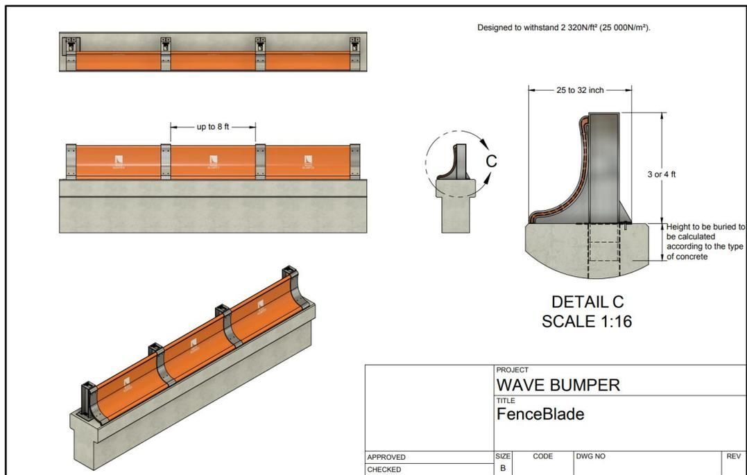
Figure 6.2.3 – Wave Bumper FenceBlade Rendering (Courtesy of USACE-NAP)
