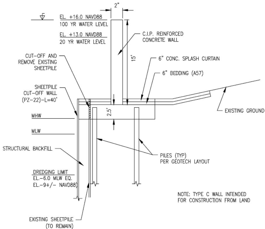
Figure 2.3.2.4 – Typical Section – Concrete Cantilever Wall on Piles – Type C
