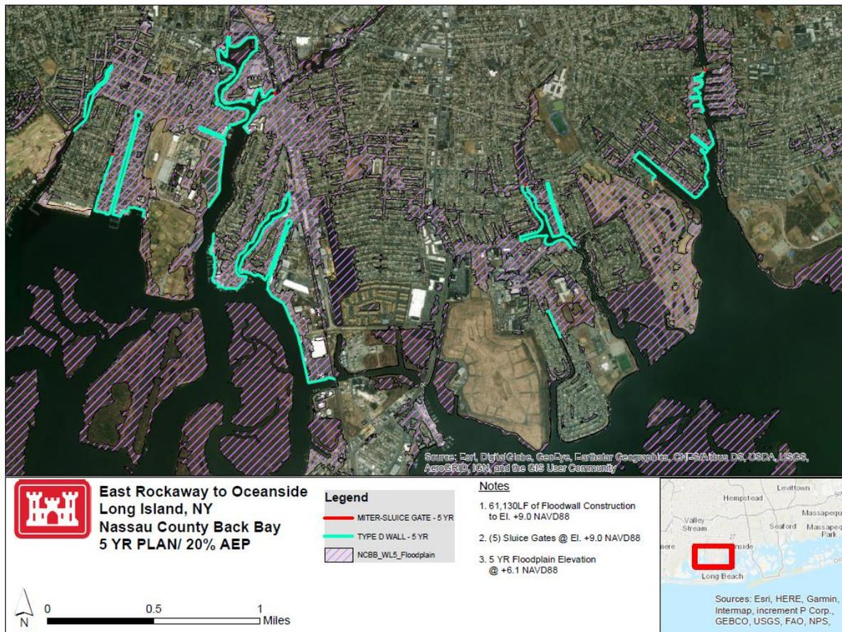
Figure 2.3.2.10: East Rockaway to Oceanside 20% AEP Plan – C1 (Courtesy of USACE-NAP)
