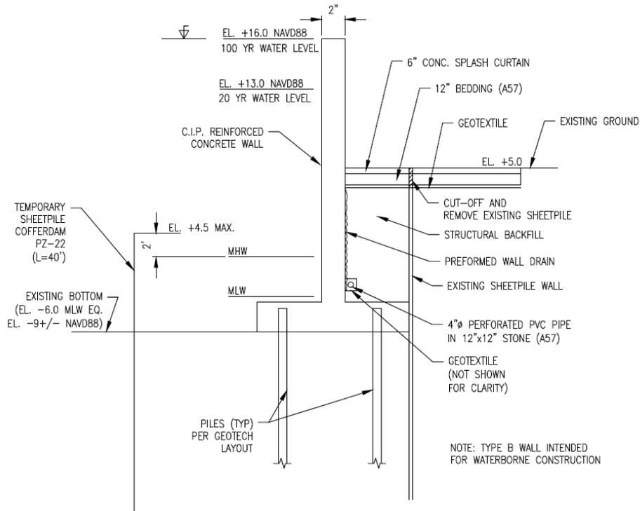
Figure 2.1.2.3 – Typical Section - Concrete Cantilever Wall on Piles - Type B
