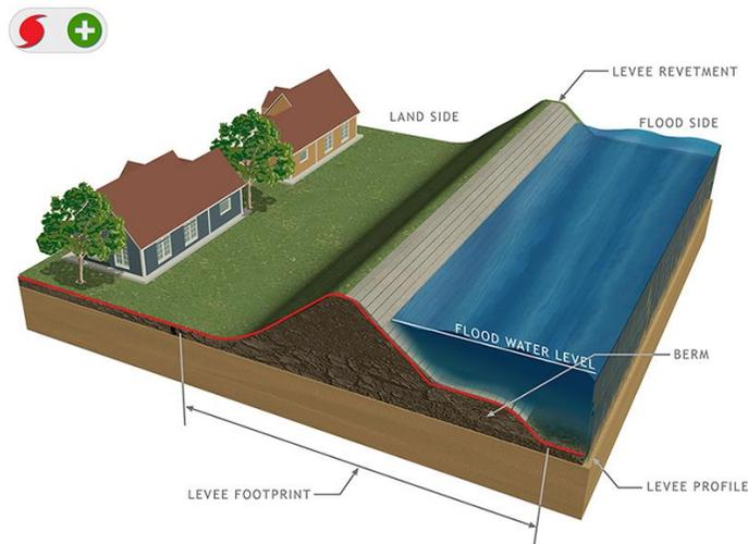
Figure 2.3.2.6 – Example of a Type A Levee (NACCS)
