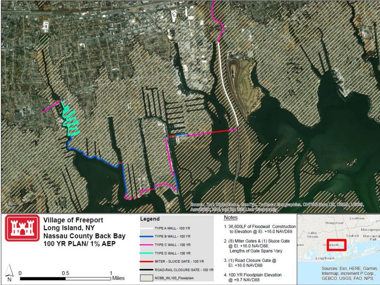
Figure 2.3.1.3 Village of Freeport 1% AEP Plan (Courtesy of USACE-NAP)
