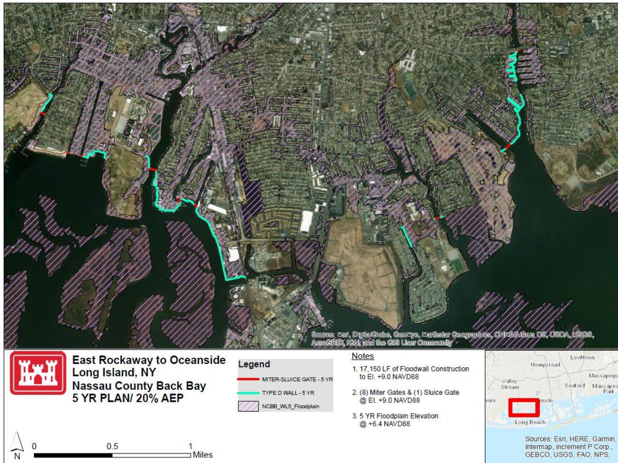
Figure 2.3.2.10: East Rockaway to Oceanside 20% AEP Plan – C2 (Courtesy of USACE-NAP)
