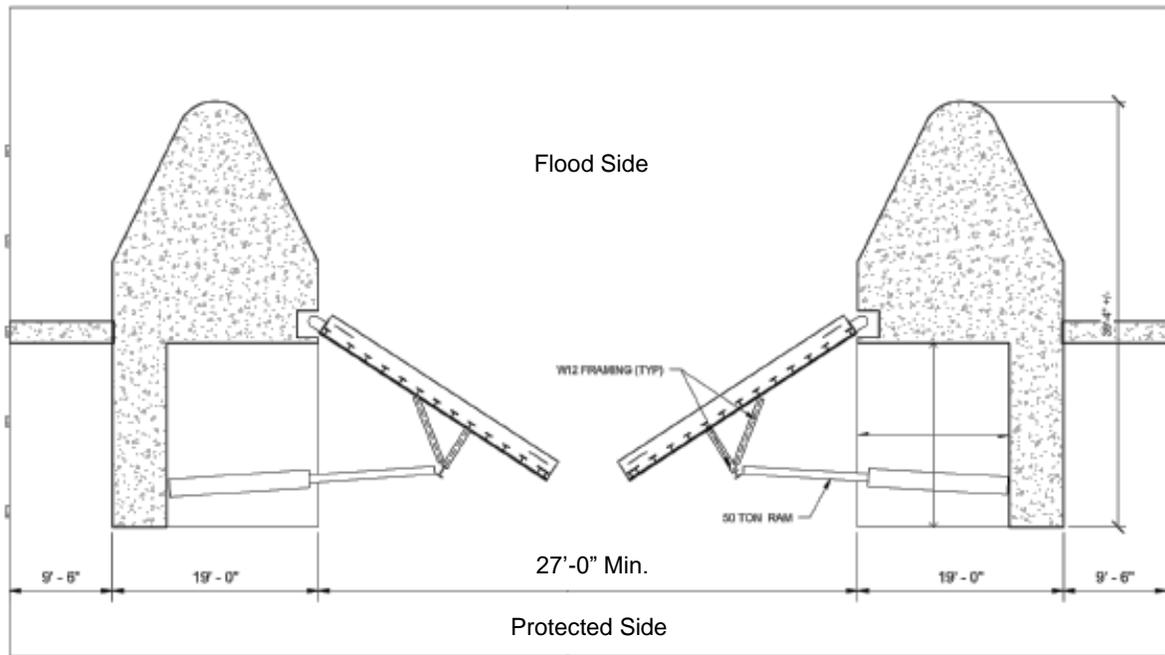
Figure 2.3.3.8 NCBB Miter Gate Design (Courtesy of USACE-NAP)
