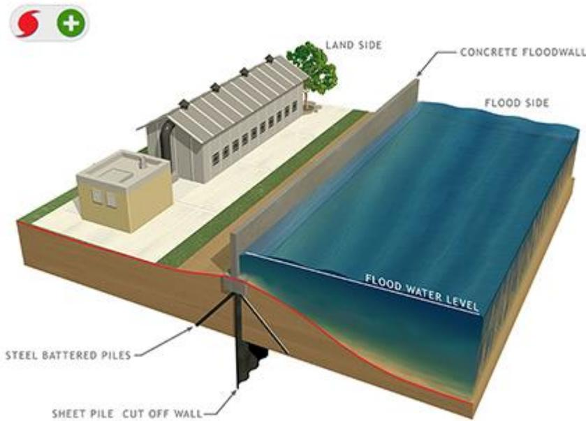
Figure 2.3.2.7 – Example of a Type B/C Floodwall (NACCS)
