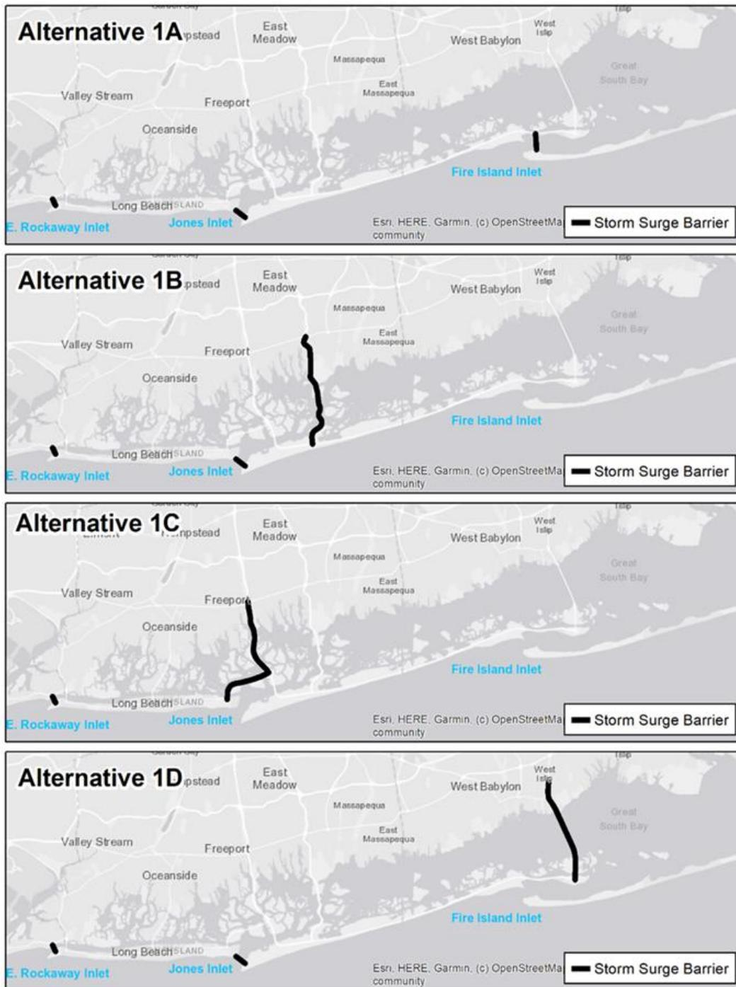
Figure 4.1.3 – USACE-NAP SSB Alternatives (Courtesy of USACE-NAP)
