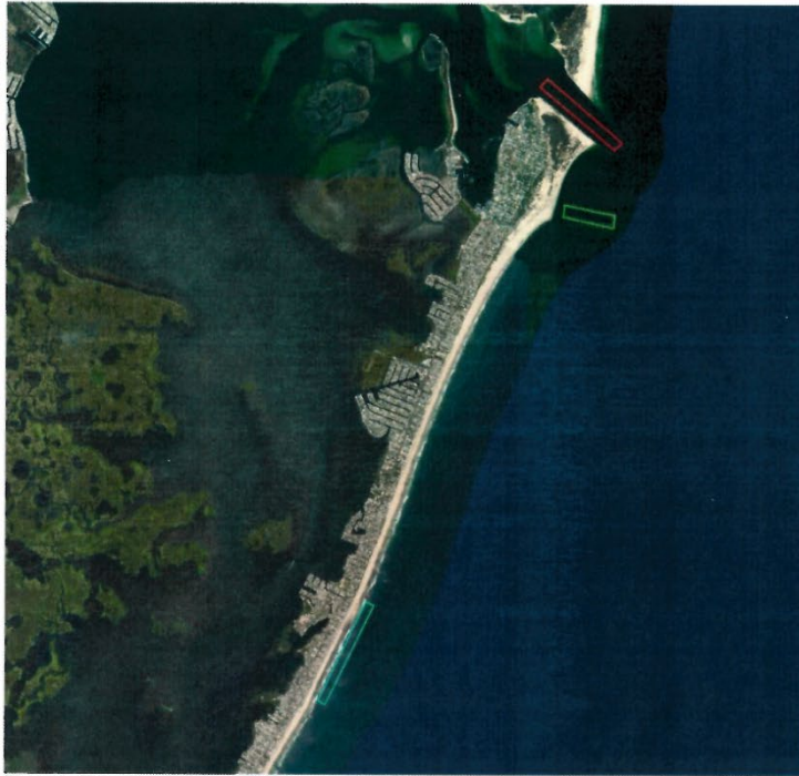
Figure 1. The red area is the existing Barnegat Inlet Federal Navigation Channel (sand source). The green area indicates one of the approved sand placement areas for the authorized Coastal Storm Management Project (LBI). The light blue rectangle is the proposed one-mile long nearshore beneficial use placement area adjacent to Harvey Cedars.
