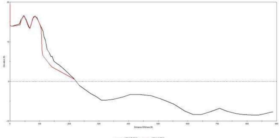
Figure 4. The cross section shows the erosion into the seaward toe of the dune with the post-storm beach slope meeting the pre-storm line at a much lower slope angle. Sand was transported offshore at the expense of the existing beach and dune.
