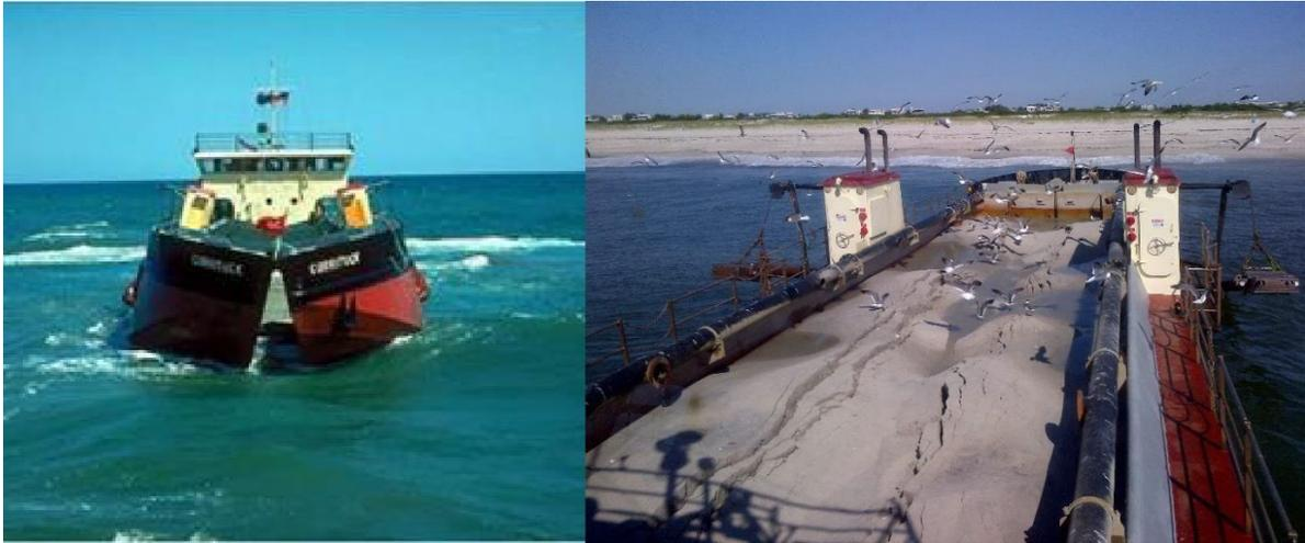
Figure 4. The Currituck placing sand in the nearshore zone of Barnegat Light during maintenance dredging operations (July 2015). This photo depicts the typical placement operation within the red box shown in Figure 3.
