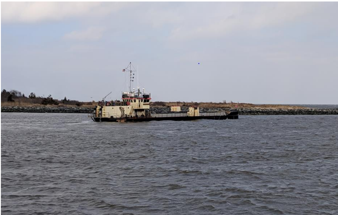
Figure 6: Government-owned small split-hull hopper Dredge Currituck.
