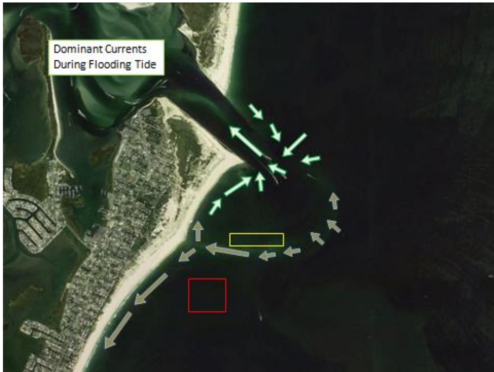
Figure 3. Current placement areas for dredging of Barnegat Inlet for routine maintenance dredging conducted twice per year. Red box is preferred, just outside of ebb shoal/nodal point and should be utilized as much as possible. Yellow box is used when placement operations are limited during higher sea conditions.
