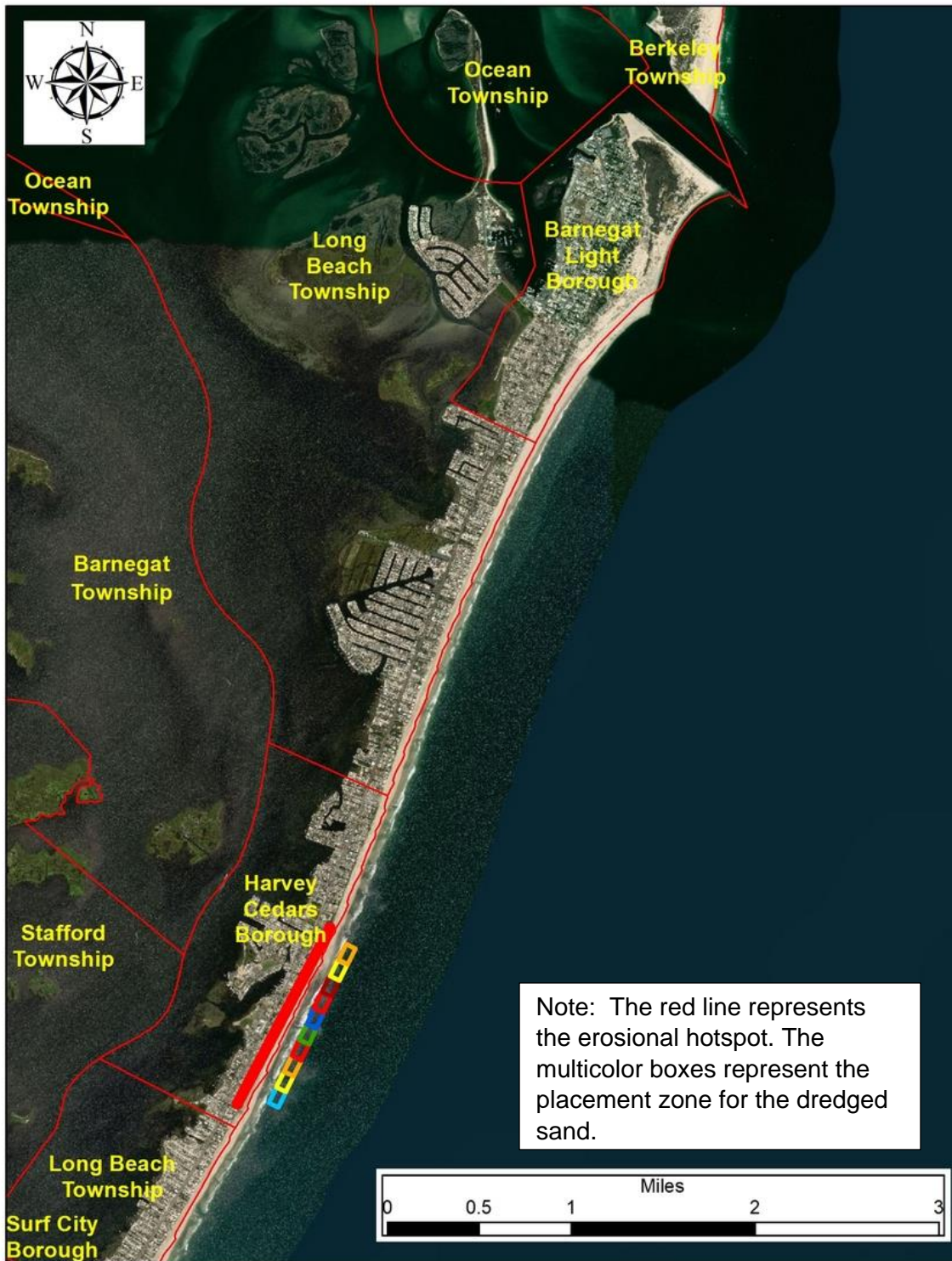
Figure 5. Location for the construction of the nearshore placement site at the southern half of Harvey Cedars, NJ.
