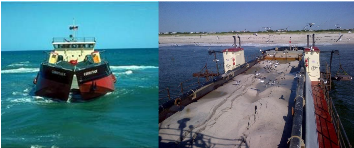
Figure 4. The Currituck placing sand in the nearshore zone of Barnegat Light during maintenance dredging operations (July 2015). This photo depicts the typical placement operation within the red box shown in Figure 3.
