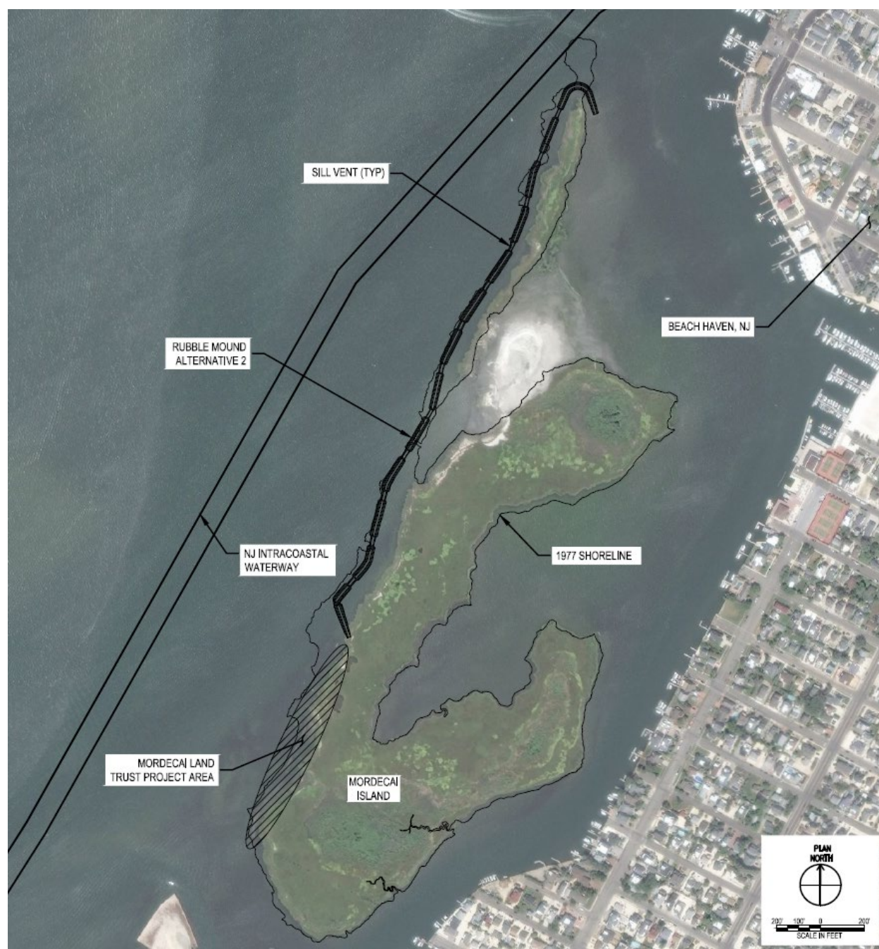
Figure 6.2: Tentatively Selected Plan Rubble Mound Plan View
