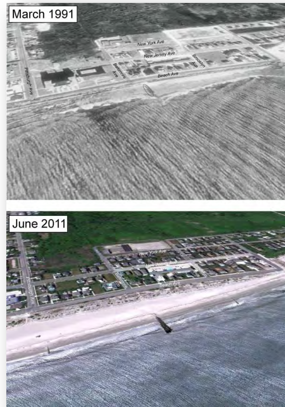
Figure 94. The groin at Baltimore Avenue in 1991 (upper panel) and conceptual proposed extension on 2011 aerial (lower panel).
