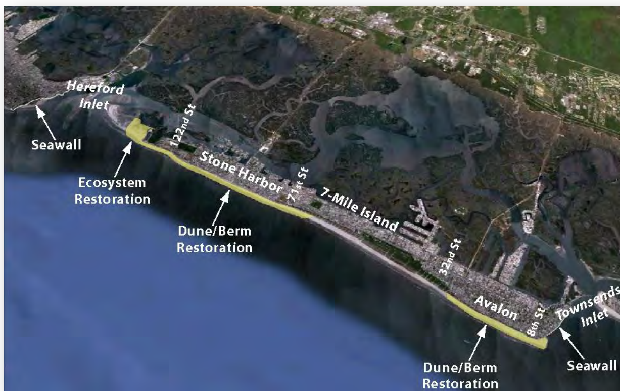
Figure 100. Townsends Inlet to Cape May Inlet (7-Mile Island) Authorized Shore Protection Project.
