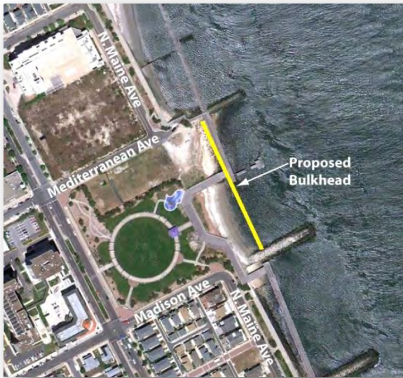
Figure 187. Proposed bulkhead expansions in Atlantic City along the Absecon Inlet shoreline.
