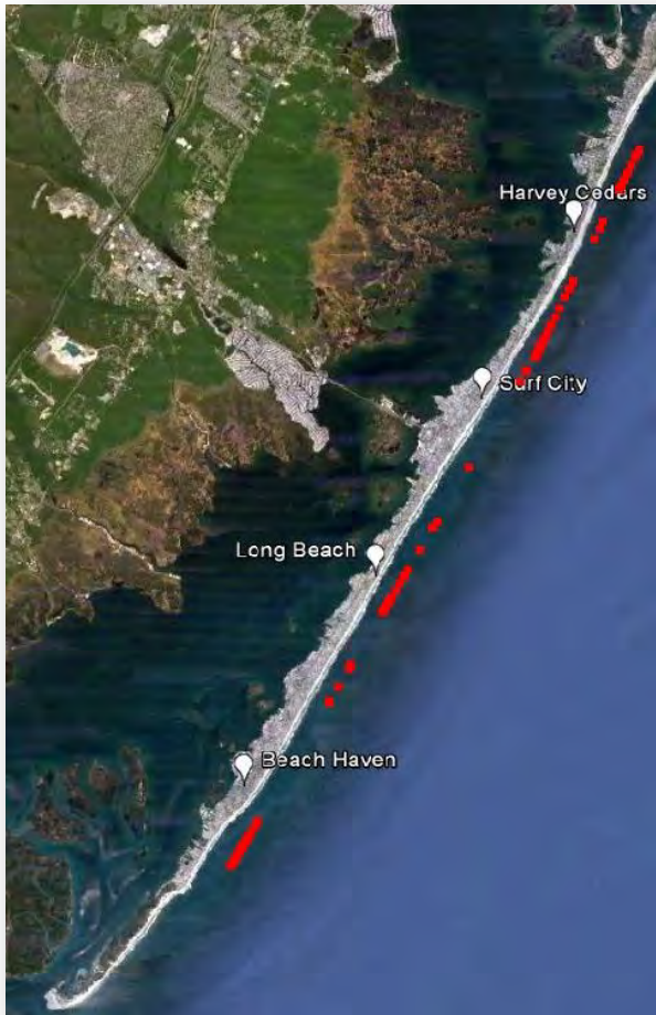
Figure 161. Erosional hotspots areas (shown in red) along Long Beach Island.
