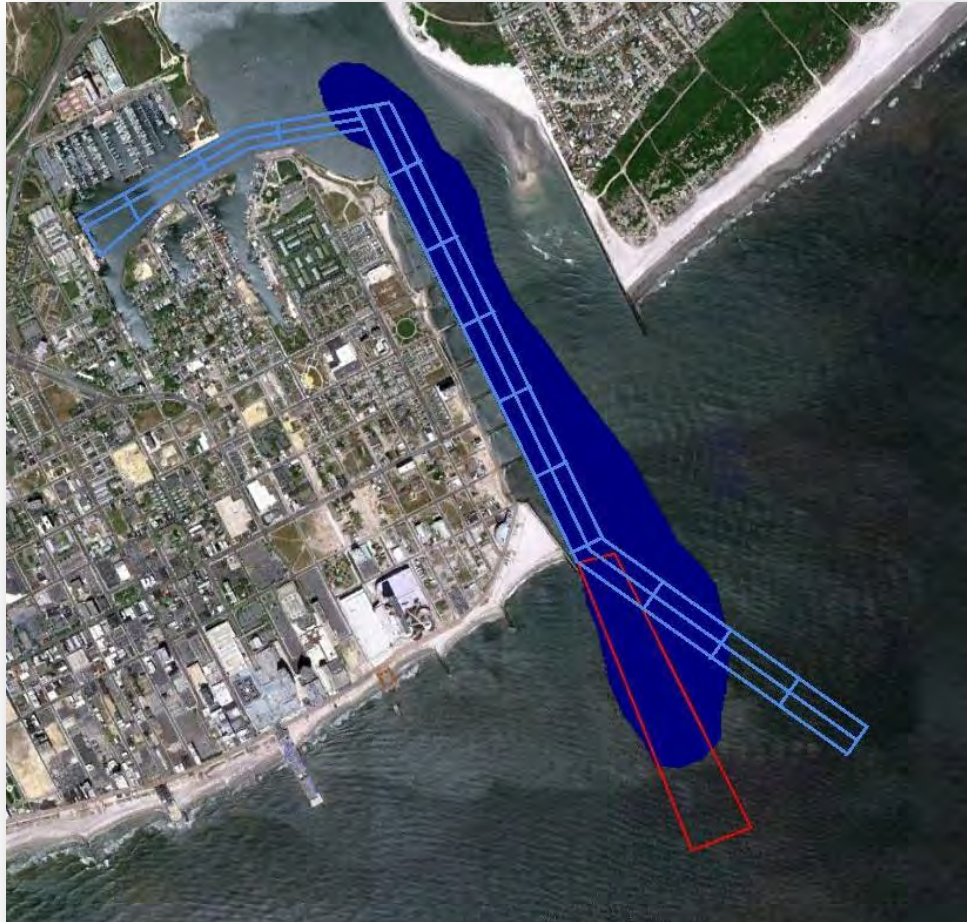
Figure 188. Potential modified dredge template at Absecon Inlet.
