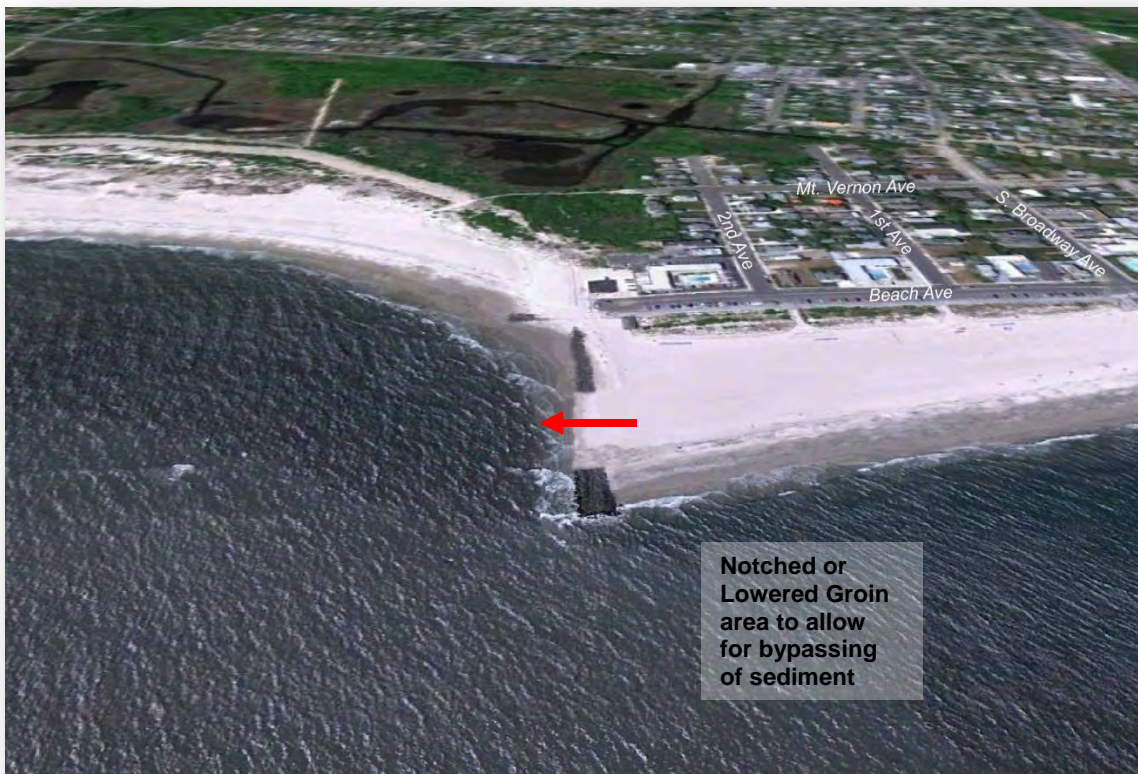
Figure 77. Conceptual design of the groin at 3 rd Avenue, impacts evaluated in the Lower Cape May Meadows project strategy section.
