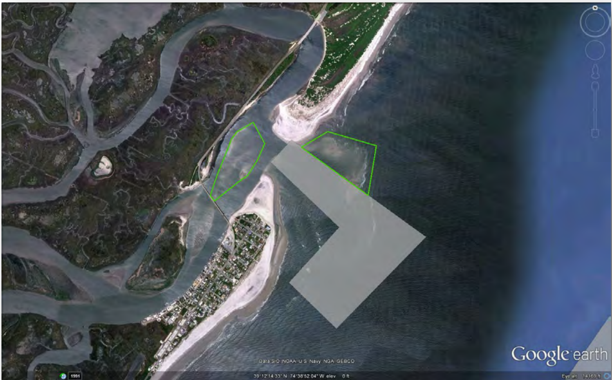
Figure 122. Potential borrow areas (green) at the ebb and flood tidal shoals of Corson Inlet. Permitted borrow areas shown as shaded white. Image courtesy of Google Earth®.
