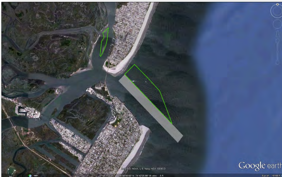
Figure 105. Potential borrow areas (green) at the ebb and flood tidal shoals of Townsends Inlet. Permitted borrow areas shown as shaded white. Image courtesy of Google Earth®.
