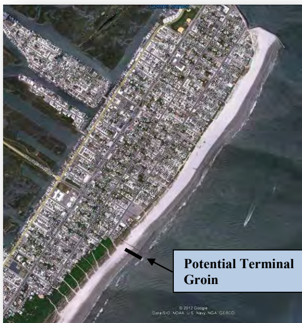
Figure 109. Potential location of a terminal groin for the Avalon beach nourishment template.
