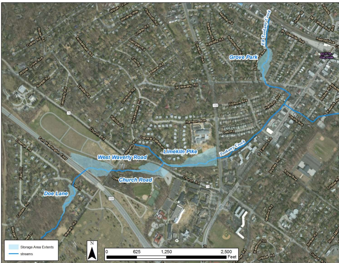
Figure 6 - Five Basins Considered in Upper Tookany Plan (Alternative 2)
