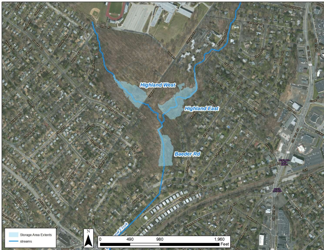
Figure 8 - Three Basins Considered in Baederwood Creek Plan (Alternative 4)
