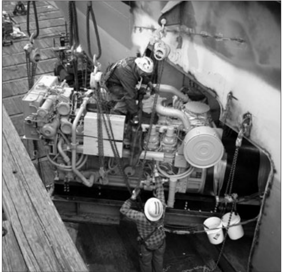
Installing an engine on a hopper dredge
