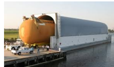
PEGASUS transporting the external tank for a shuttle launch
