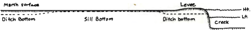
Figure 1. Side-view diagram of a sill (semi-tidal) OMWM system, with emphasis on the sill's shallow outlet.
