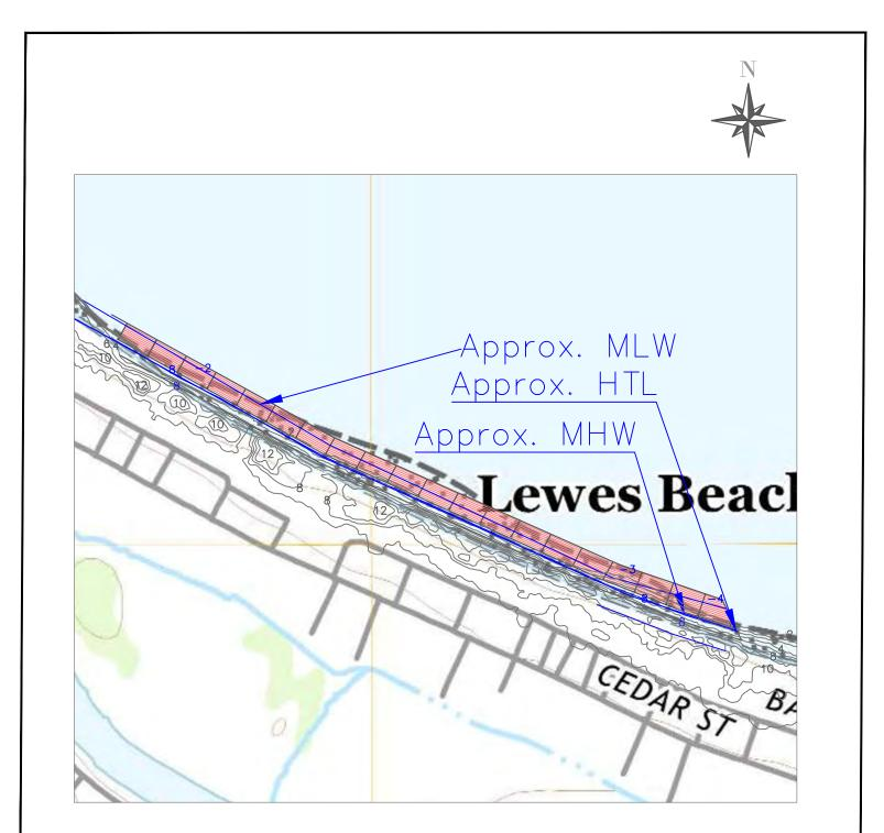
Proposed (Blue labels, red lines vs Existing LiDAR Contours (Black Labels, Grey Lines)
